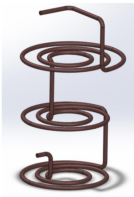
Figure 39 First concept of the reactor's heat exchanger configuration
