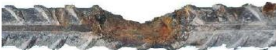
Figure 5.8: Loss of cross-sectional area due to pitting corrosion
