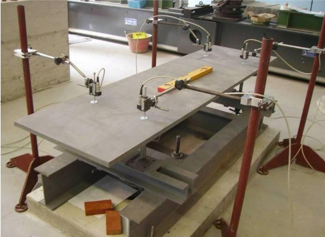
*Figure 103. The arch bridge model construction: testing of the settlement application system*
