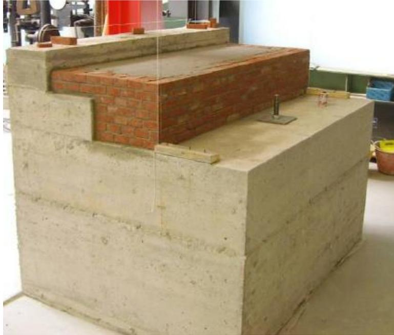
Figure 93. The arch bridge model construction: reinforced concrete block and masonry abutment
