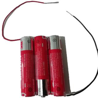
Figure 2.20: Circuit power supply: batteries in series.
