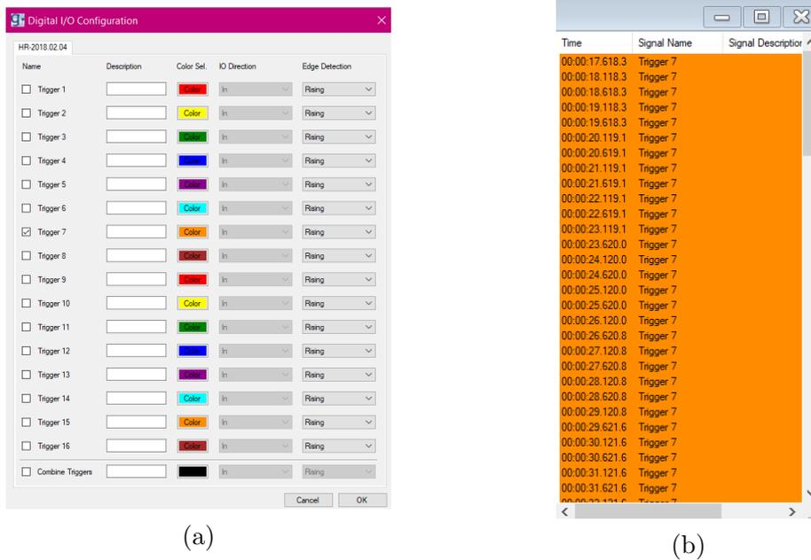
Figure 2.28: (a)List of triggers that can be selected: the trigger 7 was chosen arbitrarily. The trigger reading is enabled only on the rising edge; (b)Reading of trigger 7 every 500 ms.
