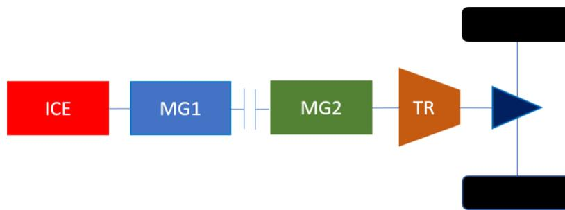
Figure 1.4: Representation of the Series-Parallel Power-train Architecture.
