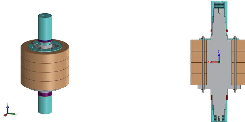
Figure 3.1.2: Rotor with four hubs and six magnets.
