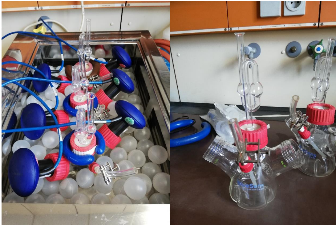
Figure 3.6 Experimental set-up of acid fermentation tests. On the right the BlueSens flask with the overpressure preventing device and sampling tube. On the left the final set-up with sensors fixed on the flasks.
