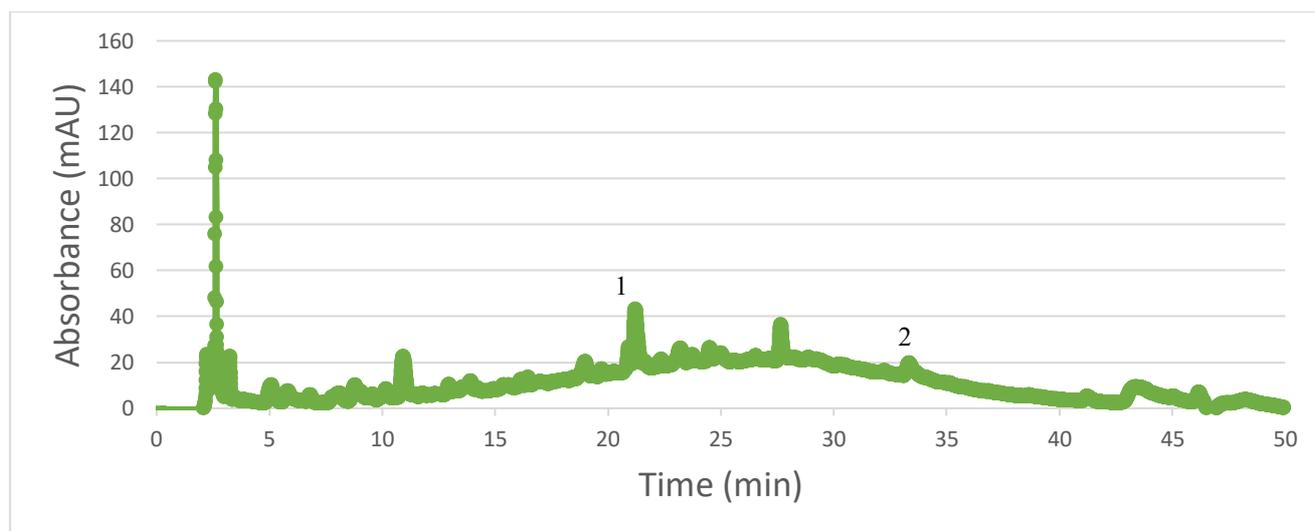
**Figure 41** - PLE Olive pomace chromatogram (370 nm) working at 100°C, 40 % EtOH, 1 cycle during 5 minutes
