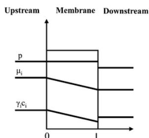
Figure 24 - Solution-diffusion model (Vandezande, Gevers, and Vankelecom 2008)
