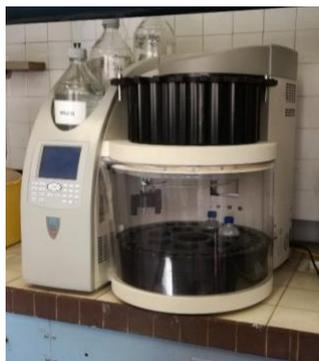
*Figure 30 - Equipment for pressurized liquid extraction -Dionex ASE 350*
