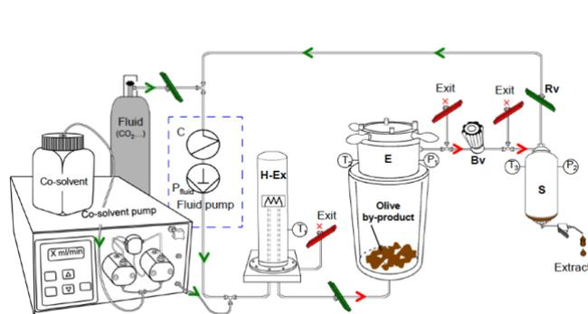
Figure 20 - Schematic lab-scale set-up of supercritical fluid extraction (Roselló-Soto *et al.* 2015)
