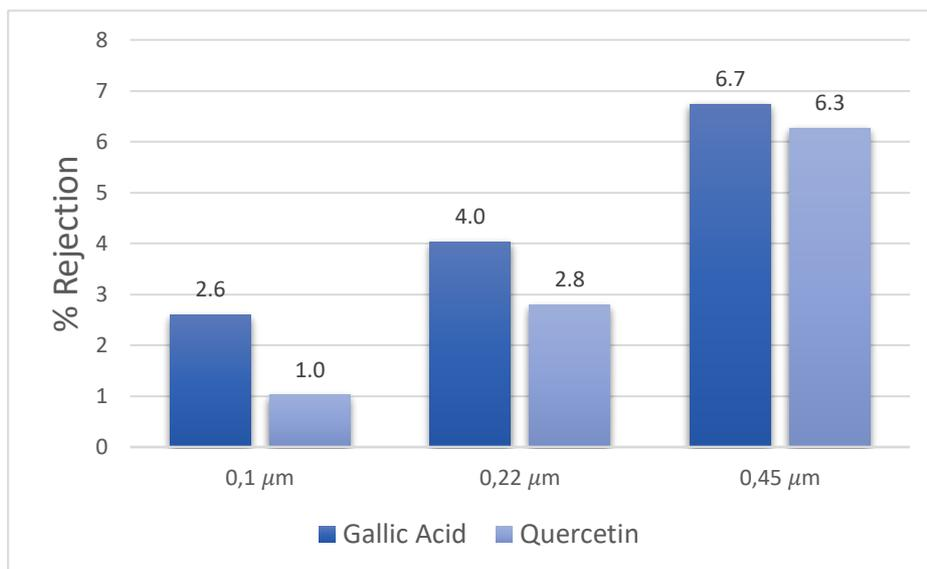
**Figure 50** - Microfiltration results for gallic acid and quercetin
