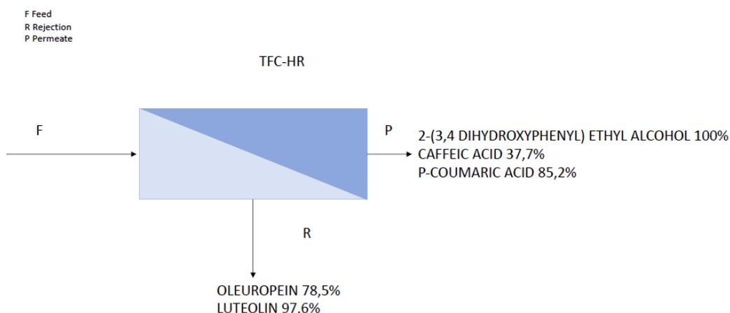
**Figure 56** - Scheme of the TFC-HR membrane system performance and corresponding result
