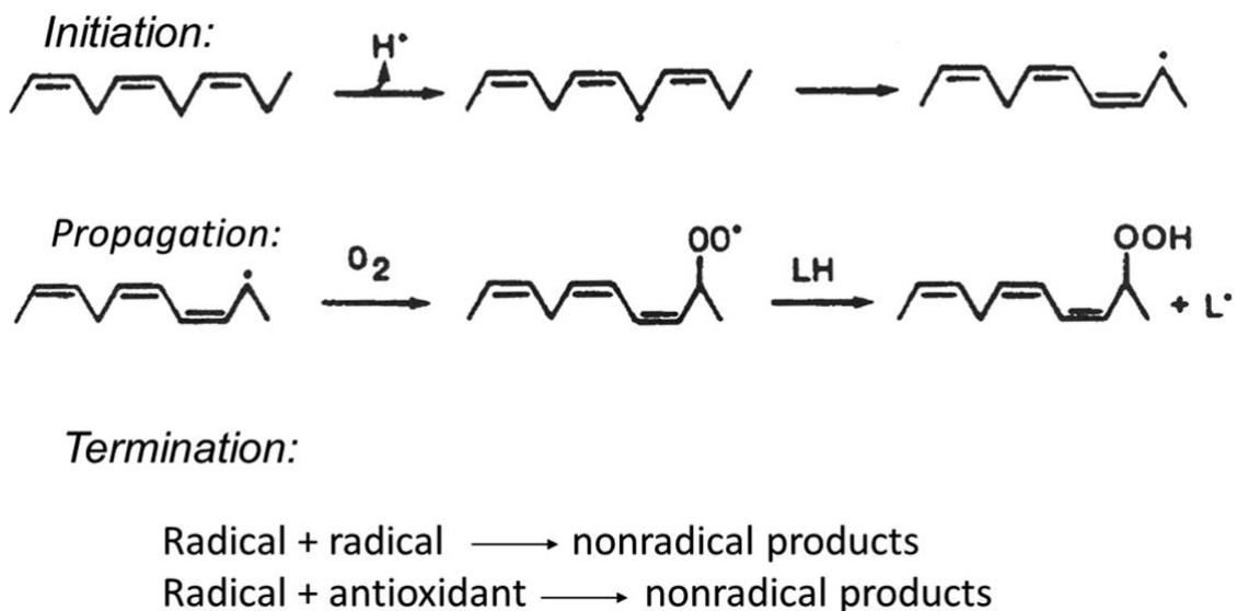
**Figure 1** – The three stages of lipid peroxidation: initiation, propagation, termination (Yang *et al.* 2018)
