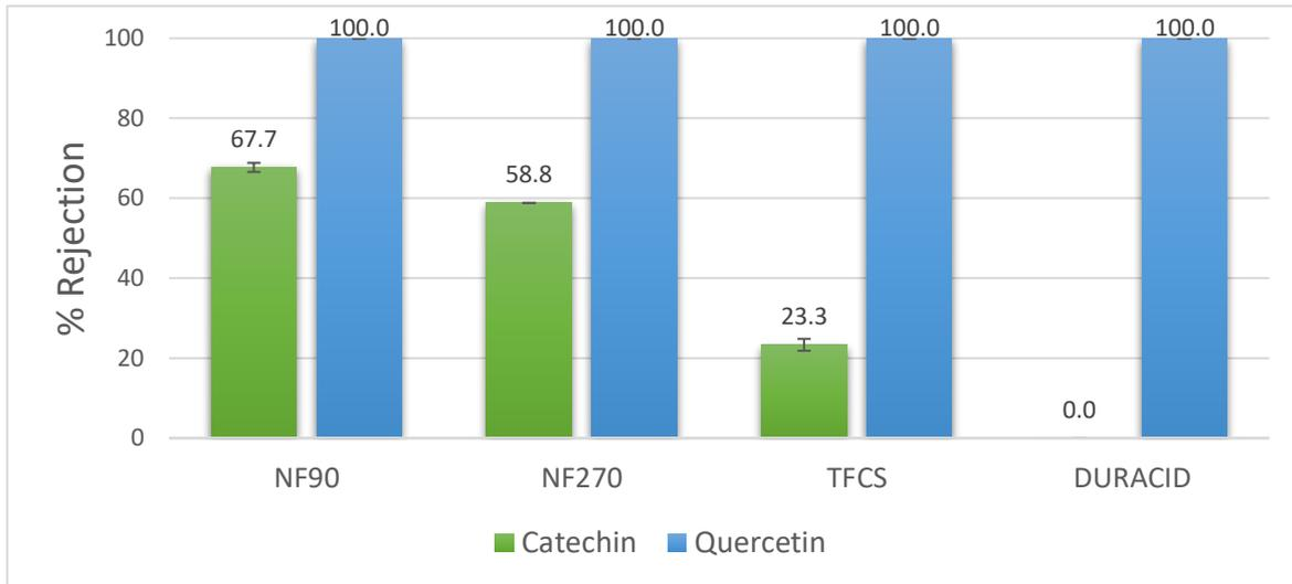
**Figure 52** –Rejection percentages for catechin and quercetin by nanofiltration
