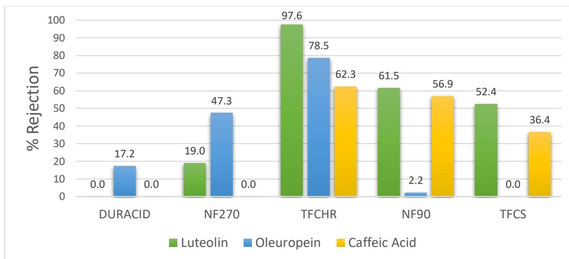
*Figure 55 - Nanofiltration results for luteolin, oleuropein and caffeic acid (% rejection)*
