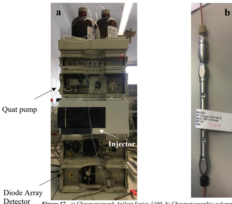
Figure 37 - a) Chromatograph Agilent Series 1100, b) Chromatographic column
