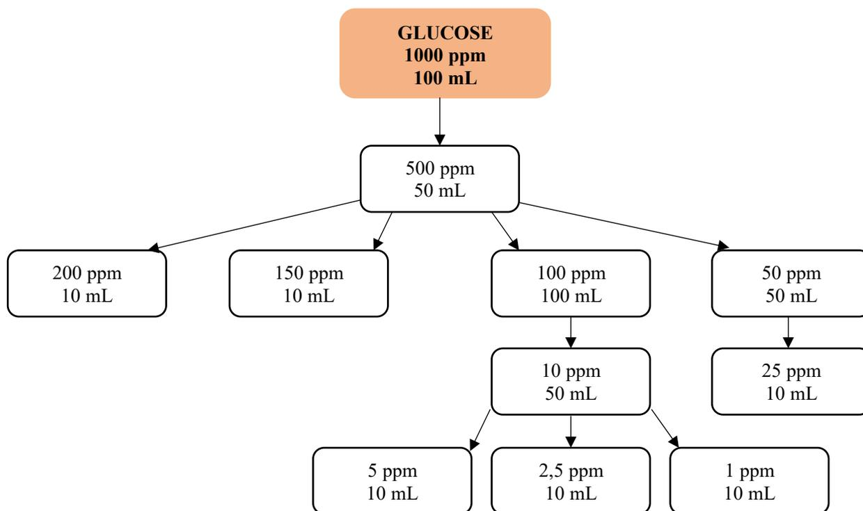
*Figure 38 - Preparation of glucose calibration line*
