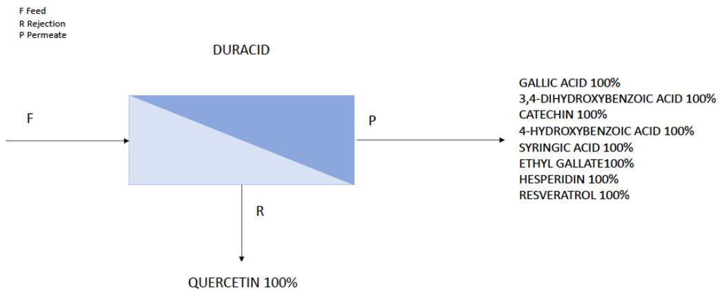
**Figure 53** - Scheme of the membrane system performance for DURACID membrane and corresponding result
