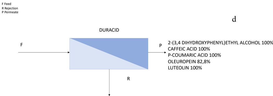
**Figure 57 - Nanofiltration membranes schemes a) NF270, b) NF90, c) TFCS, d) DURACID**
