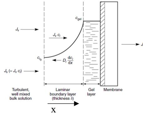
**Figure 22** – Schematic representation of gel-layer model
