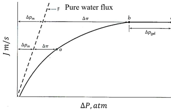
Figure 23 – Flux vs applied pressure
