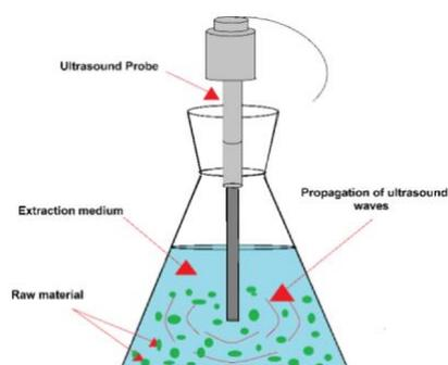
**Figure 17** - Ultrasound system coupled to a probe (Medina-Torres *et al.* 2017)
