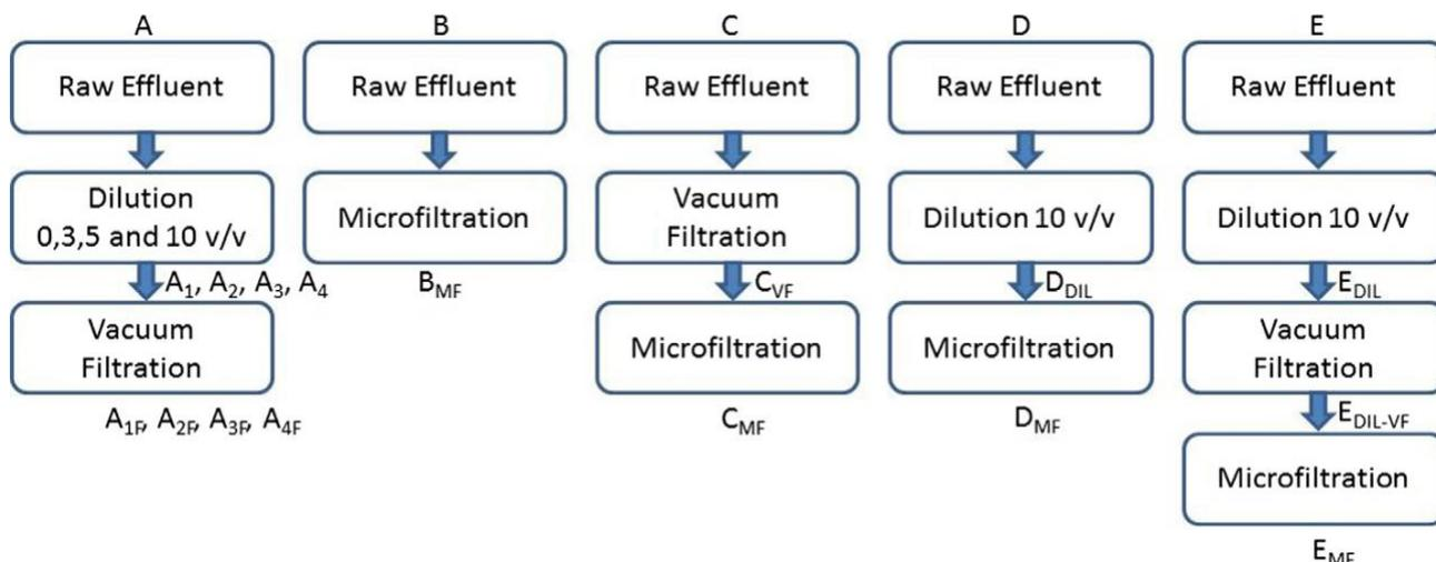
Figure 25- Flow chart of the experiments (Giacobbo et al. 2015)
