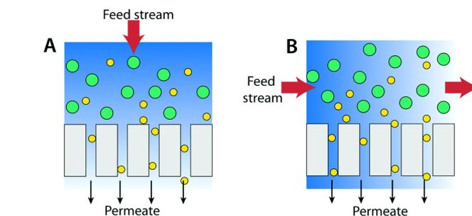
Figure 21 - Scheme of dead-end filtration (A) and cross-flow filtration (B)
