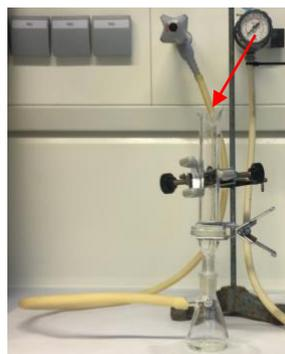
*Figure 35 - Microfiltration equipment*
