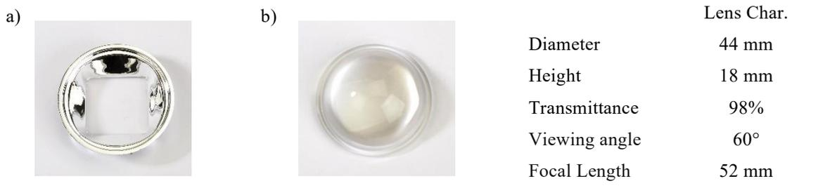
Figure 46: a) Reflector collimator; b) Lens; Lens characteristics [52].
