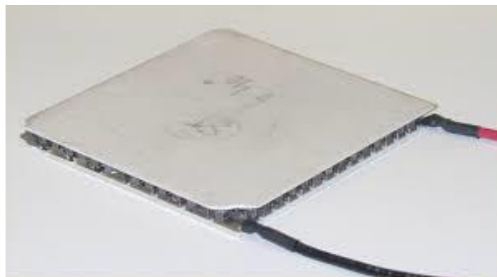
Figure 31 - A common Peltier cell
