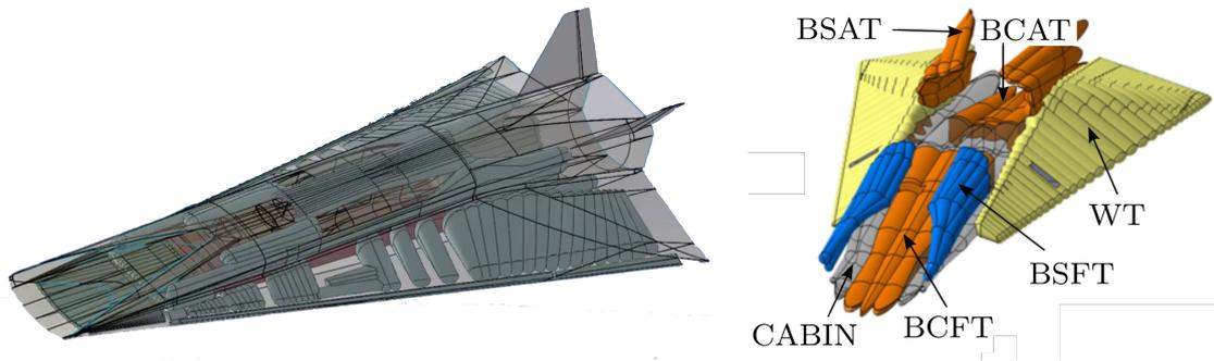
Figure 2.14. Tanks configuration for STRATOFLY MR3 (LHS) and LAPCAT MR2 (RHS).
