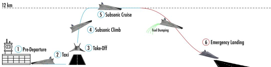
Figure 6.6. Scenario 8: Emergency landing after the Subsonic Cruise.
