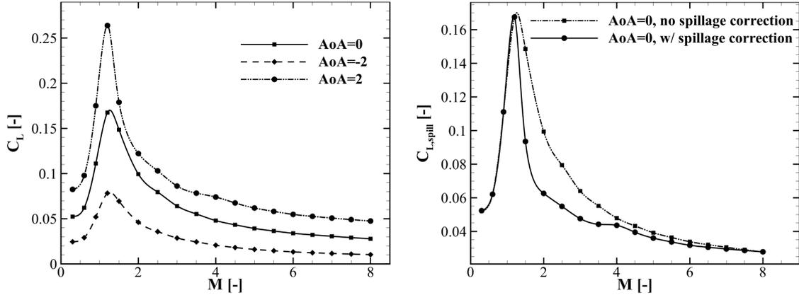
Figure 2.8. Lift coefficient as a function of Mach number and angle of attack with and without spillage correction, as used in ASTOS. Credit: [18]
