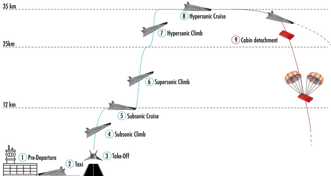
Figure 6.8. Scenario 14: Cabin and cockpit detachment during Hypersonic Cruise.
