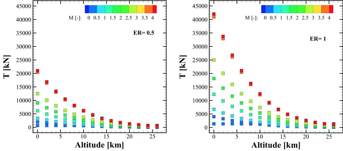
Figure 2.10. ATR performances as a function of altitude and Mach number at ER=0.5 and ER=1, as used in ASTOS. Credit: [18]
