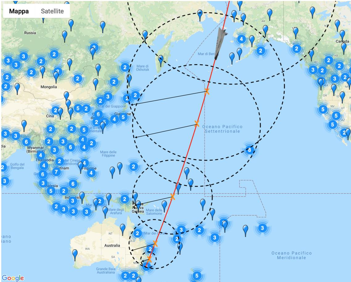
Figure 9.8. Map of airports close to STRATOFLY MR3 trajectory potentially reachable after a DMR failure. Qualitative illustration.
