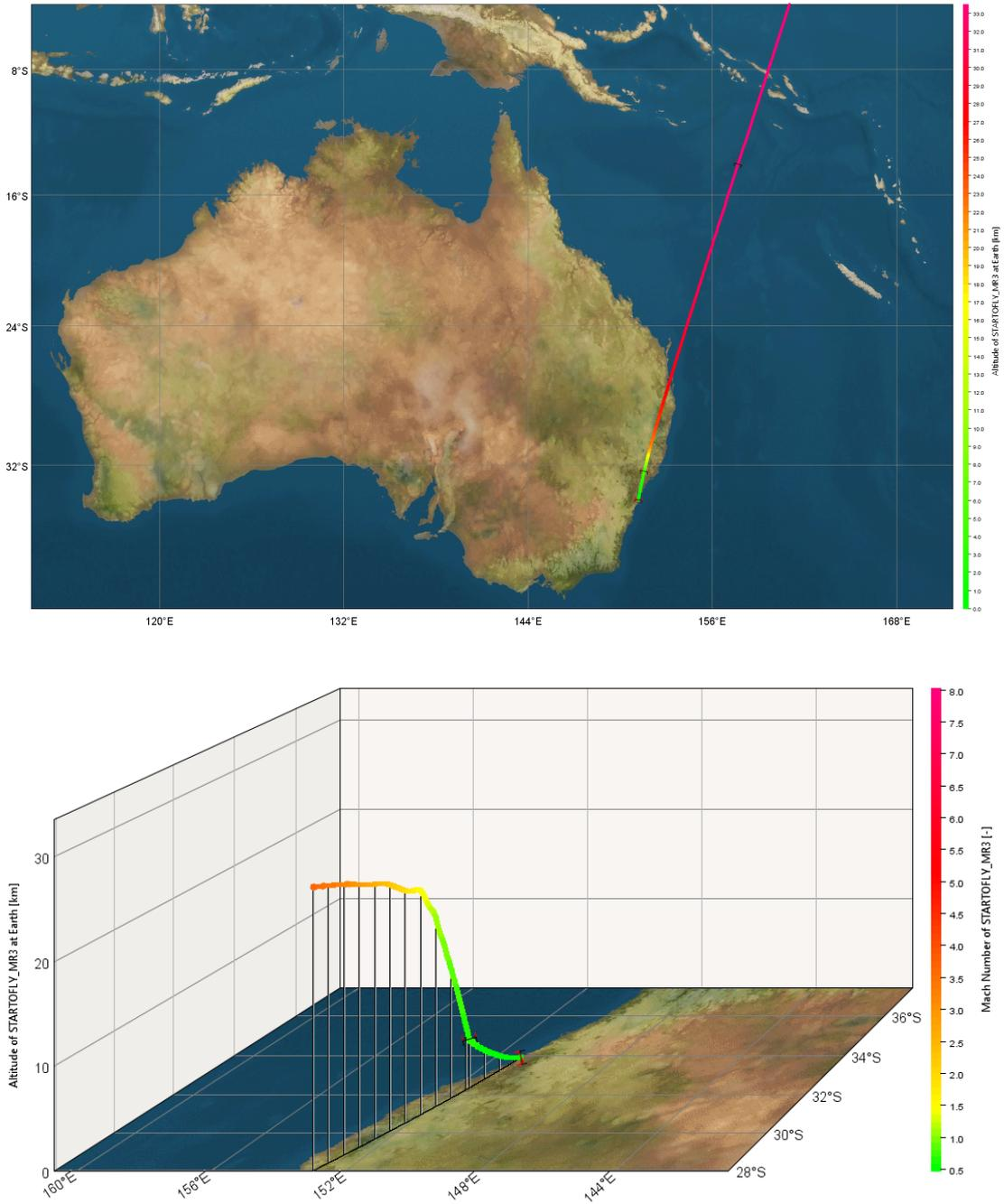
Figure 8.9. Final part of trajectory and Landing to Sydney Airport in the case of overland final approach (Option A). 2D map (top) - 3D view looking in southern direction (bottom).
