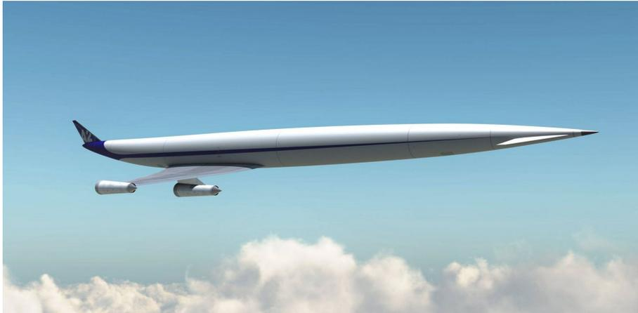
Figure 1.18. Illustration of the *LAPCAT A2*, outcome of LAPCAT I project for civil Mach 5 transport. Credit: [33]
