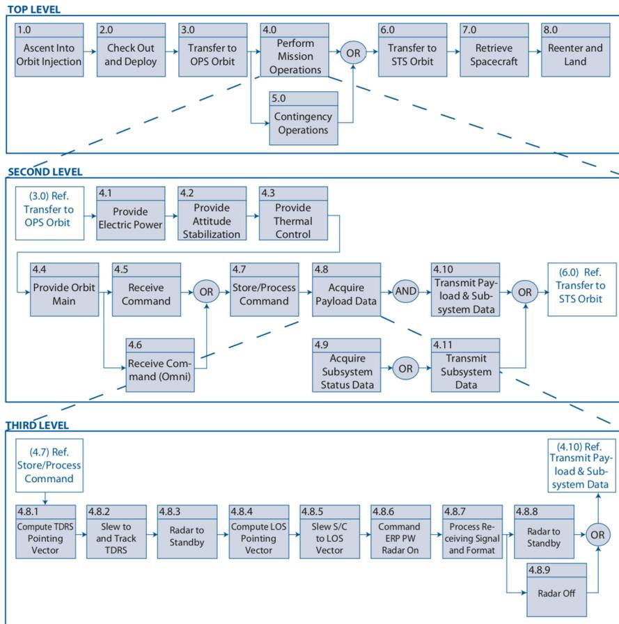
Figure 3.3. Example of a Functional Flow Block Diagram. Credit: [21]
