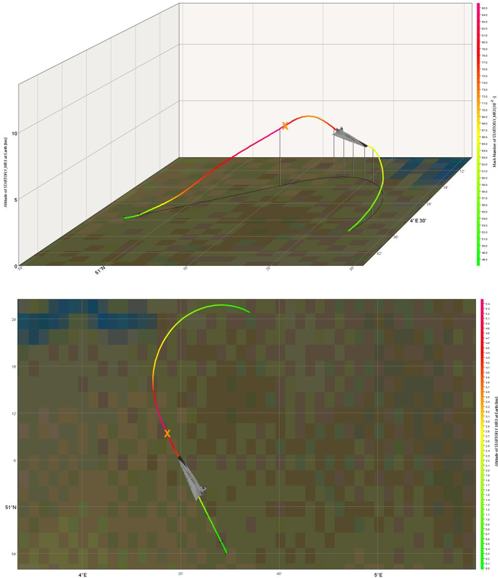
Figure 9.1. Scenario 6: Catastrophic event after an ATR failure affecting all the 6 engines occurs during early subsonic climb. (top) 3D view looking in western direction - (bottom) 2D map.
