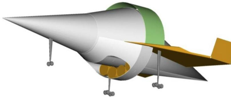
Figure 1.22. Illustration of the mbda Mach 8 civil aircraft concept, conceived within LAPCAT-II project. Credit: [31]
