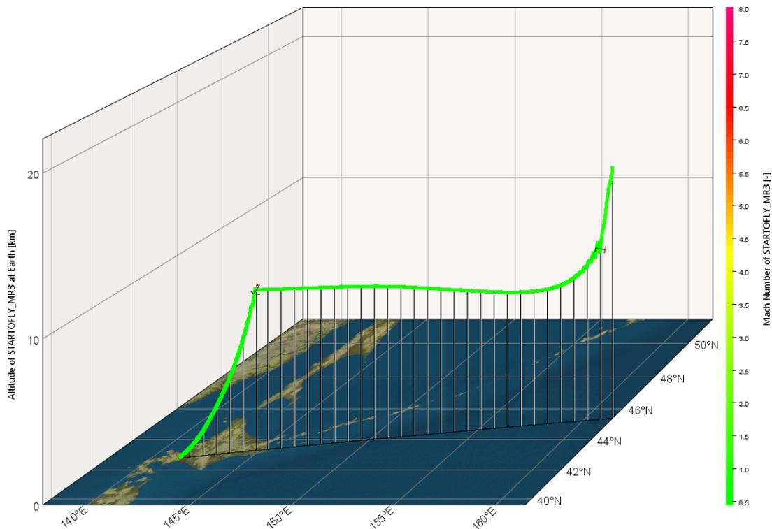
Figure 9.12. Emergency Landing to Sapporo New Chitose Airport after a failure occurs during hypersonic cruise to the DMR at mission time  $t = 5832 s$ . 3D view looking in northern direction.
