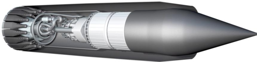
Figure 1.19. Illustration of the *SABRE* engine developed by ReactionEngines. Credit: [51]
