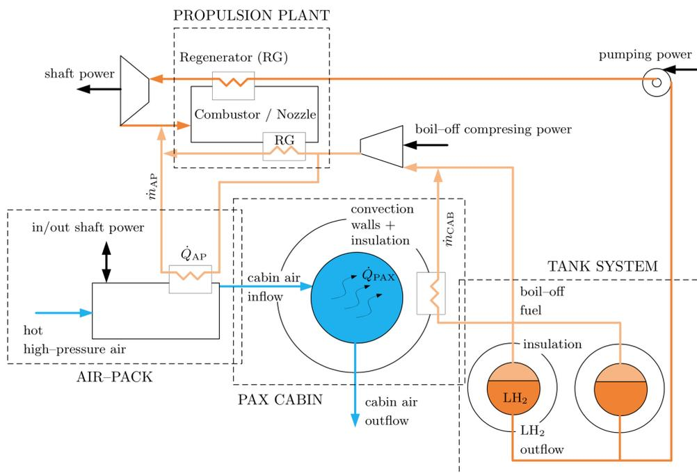
Figure 2.12. Illustration of the Thermal and Energy Management Subsystem. Credit: [12]
