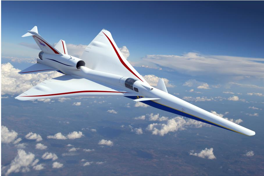
Figure 1.13. Illustration of the Lockheed Martin X-59 QueSST, experimental vehicle aimed to demonstrate low sonic boom technologies. Credit: [49]
