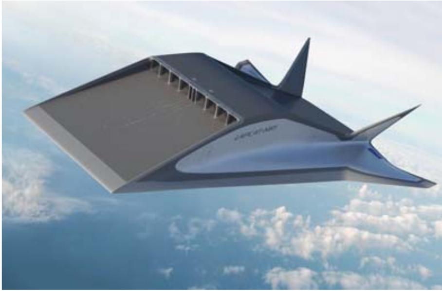
Figure 1.20. Illustration of the *LAPCAT MR1*, outcome of LAPCAT I project for civil Mach 5 transport. Credit: [33]
