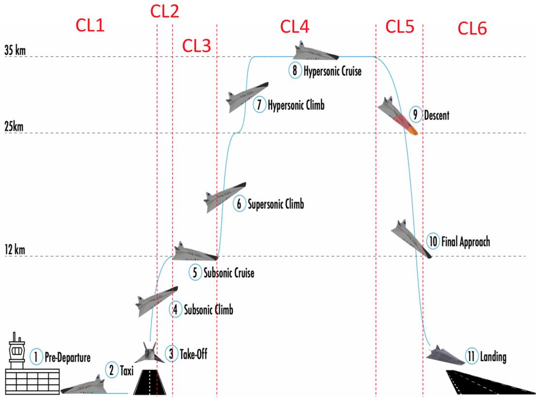
Figure 6.2. Graphical description of phases clusterization.
