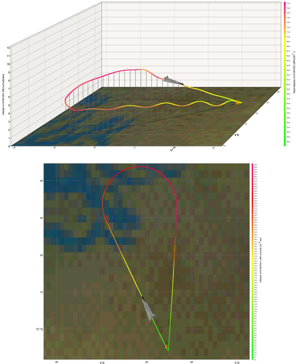
Figure 9.2. Scenario 5: Emergency landing to departure airport soon after take off as consequence of an ATR failure affecting 5 out of 6 engine. Only one ATR engine is available. (top) 3D view looking in eastern direction - (bottom) 2D map.
