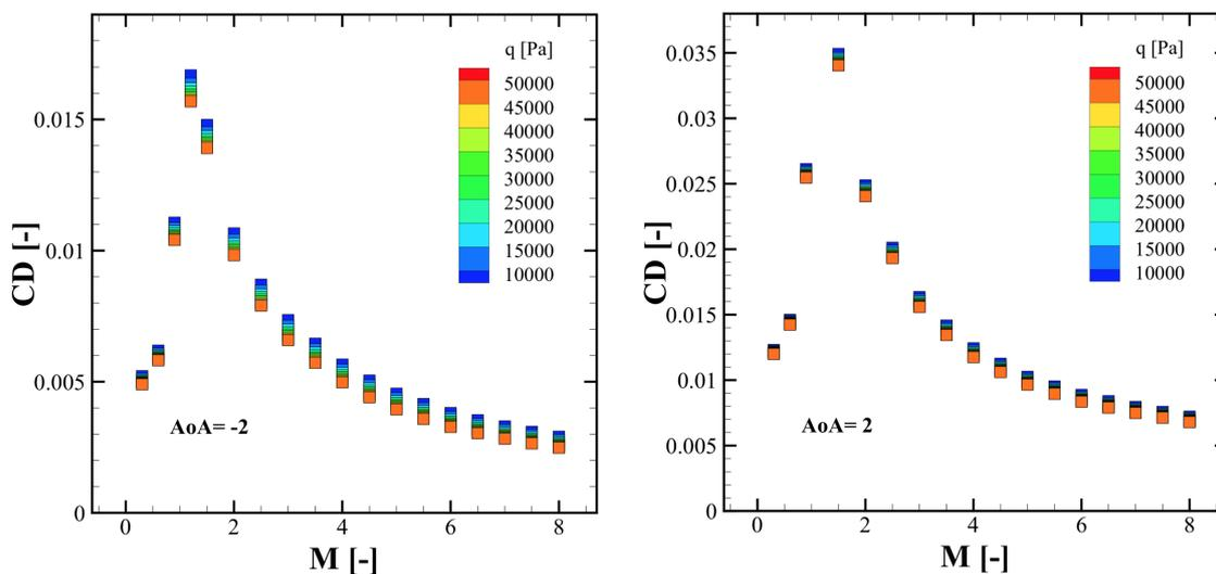
Figure 2.7. Drag coefficient for two different angles of attack as a function of Mach number and dynamic pressure, as used in ASTOS. Credit: [18]
