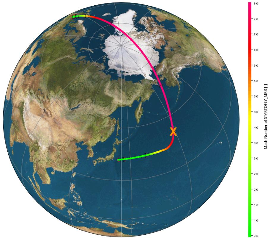
Figure 9.15. Satellite view on the Emergency Splashdown near Tokyo after a failure occurs during hypersonic cruise to the DMR at mission time  $t = 6356 s$ .
