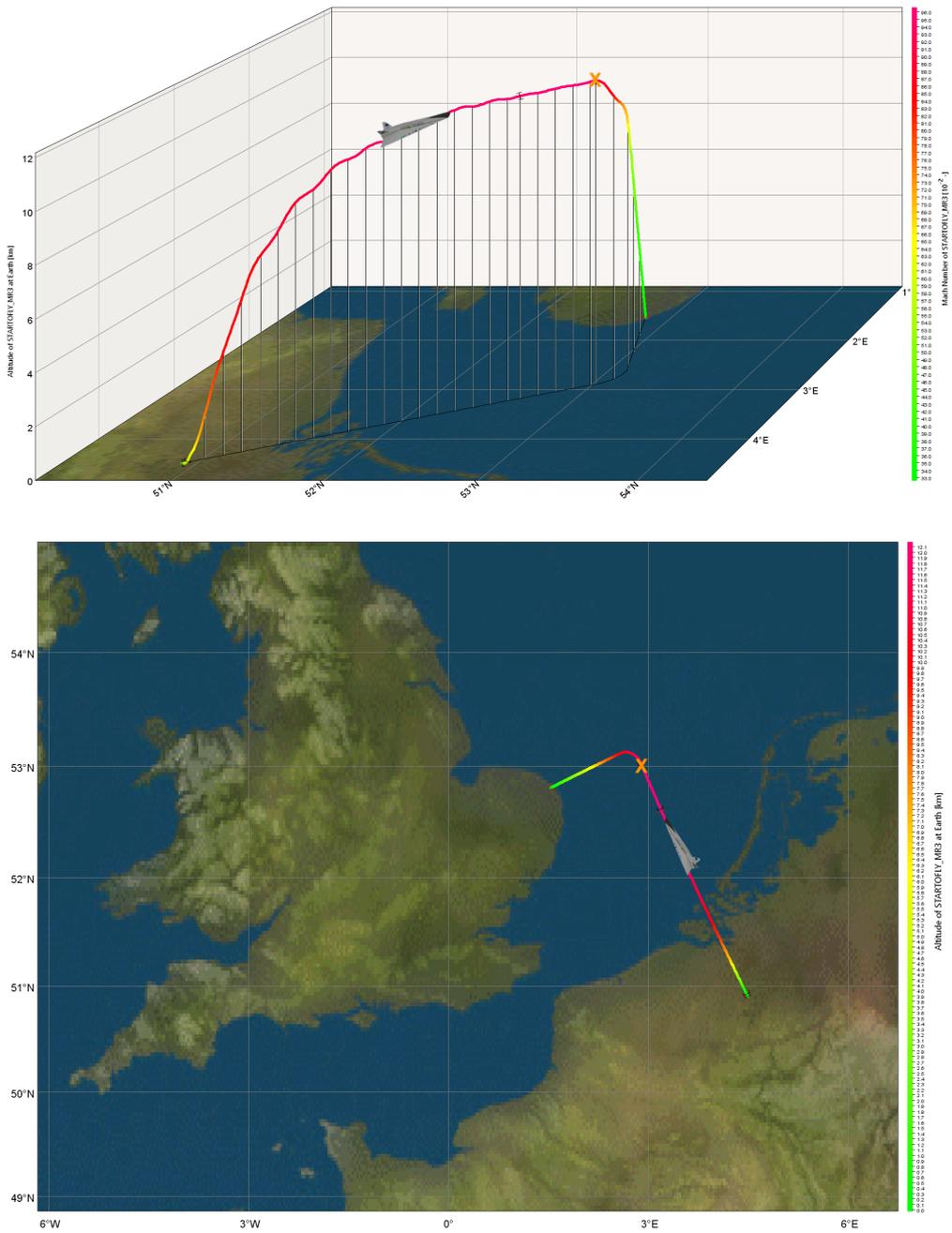
Figure 9.4. Scenario 8: Emergency landing to Norwich Airport (UK) after an ATR failure occurs during subsonic cruise. None of the ATR engines is available. (top) 3D view looking in western direction - (bottom) 2D map.
