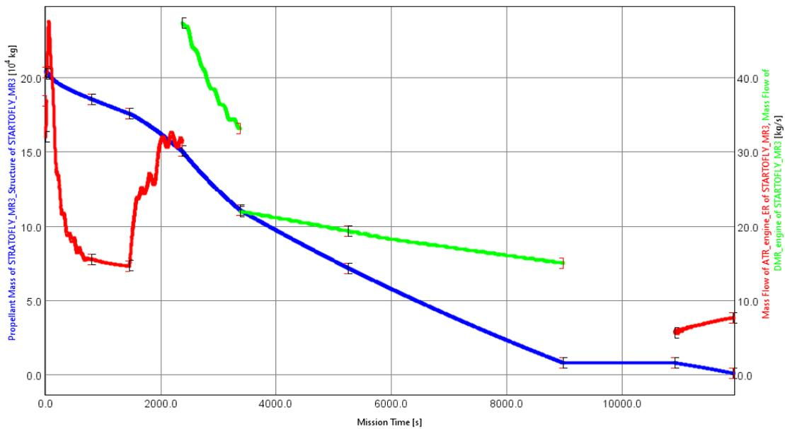
Figure 8.11. Fuel mass and fuel massflow *vs.* Mission Time in the case of overland final approach (Option A).
