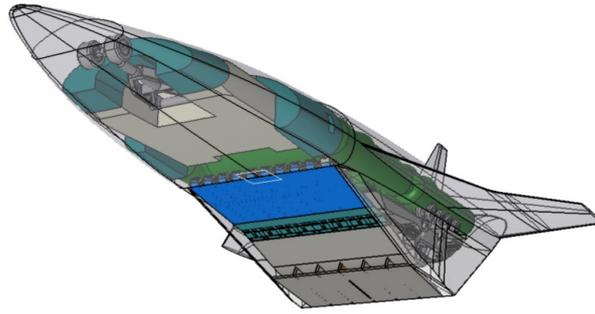
Figure 1.21. Illustration of the ONERA/ULB/UniROMA Mach 8 civil aircraft concept, conceived within LAPCAT-II project. Credit: [31]
