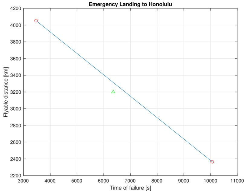
Figure 9.19. Flyable distance after failure *vs.* time on which a DMR failure occurs and distance from failure point to Honolulu Airport (green triangle) at mission time  $t = 6356$  s.
