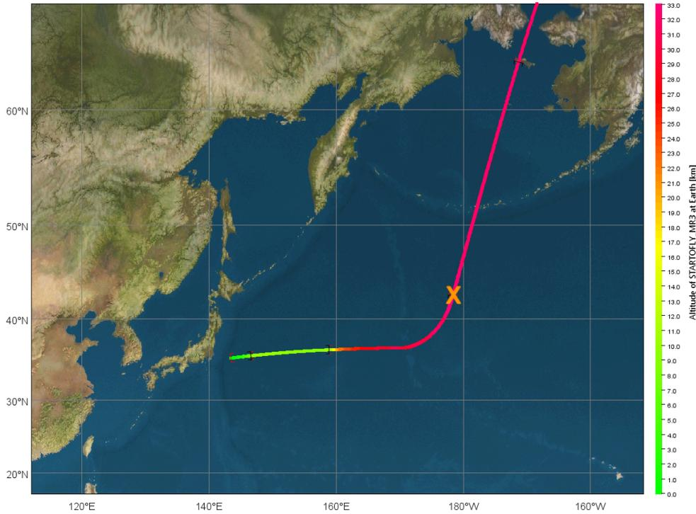
Figure 9.16. 2D trajectory of an the Emergency Splashdown near Tokyo after a failure occurs during hypersonic cruise to the DMR at mission time  $t = 6356$  s.
