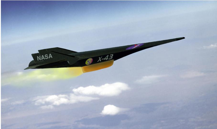
Figure 1.9. The X-43A Hypersonic Experimental Vehicle, first air-breathing aircraft ever reaching hypersonic speed. Credit: [49]
