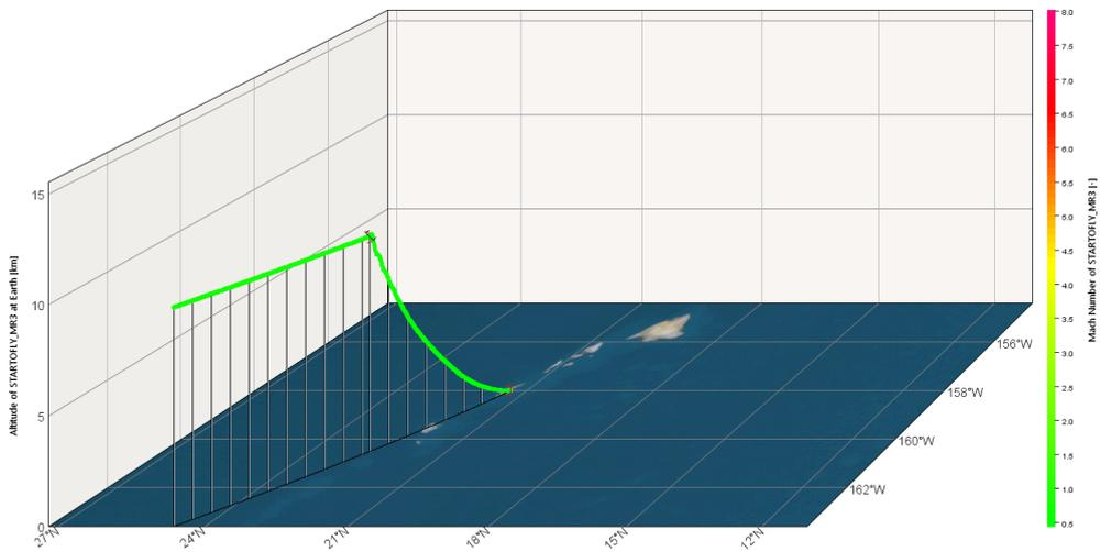
Figure 9.22. Emergency Landing to Honolulu Airport after a failure occurs during hypersonic cruise to the DMR at mission time  $t = 6356$  s. 3D view looking in eastern direction.
