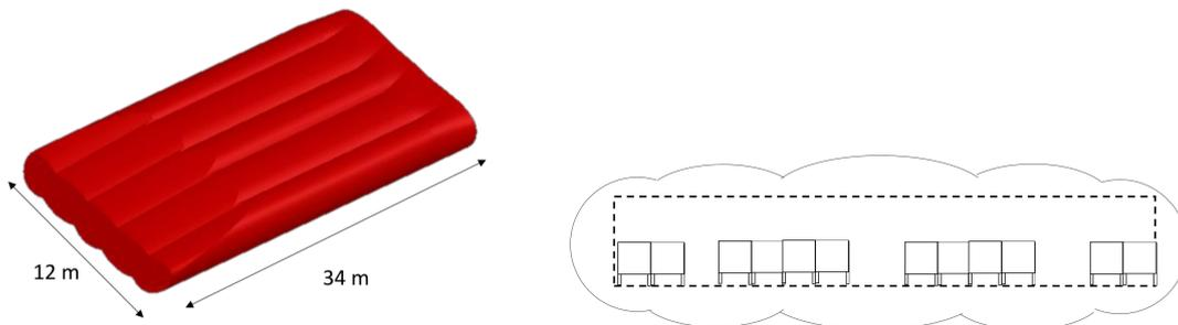
Figure 2.6. STRATOFly MR3 passenger cabin dimensions and internal configuration.
