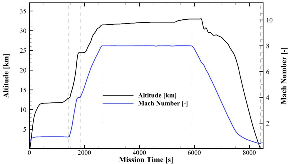
Figure 4.3. Mach number and flight altitude versus mission time during the Brussels-Sidney LAPCAT MR2 reference mission. Credit: [18]
