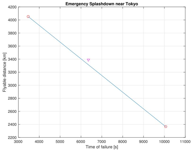
Figure 9.14. Flyable distance after failure *vs.* time on which a DMR failure occurs and distance from failure point to Tokyo Haneda Airport (purple triangle) at mission time  $t = 6356$  s.
