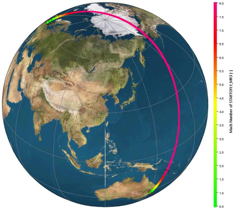
Figure 8.8. View on complete trajectory in the case of overland final approach (Option A).
