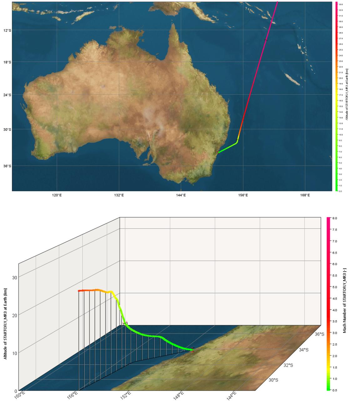
Figure 8.13. Final part of trajectory and Landing to Sydney Airport in the case of oversea final approach (Option B). 2D map (top) - 3D view looking in southern direction (bottom).
