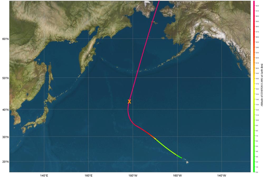
Figure 9.21. 2D trajectory of an Emergency Landing to Honolulu Airport after a failure occurs during hypersonic cruise to the DMR at mission time  $t = 6356$  s.
