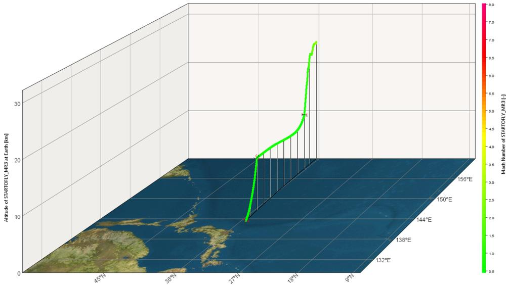
Figure 9.17. Emergency Splashdown near Tokyo after a failure occurs during hypersonic cruise to the DMR at mission time  $t = 6356$  s. 3D view looking in eastern direction.
