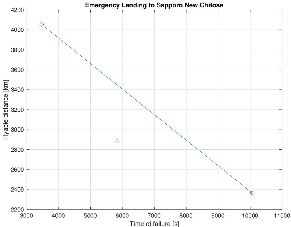
Figure 9.9. Flyable distance after failure *vs.* time on which a DMR failure occurs and distance from failure point to Sapporo New Chitose Airport (green triangle) at mission time  $t = 5832$  s.
