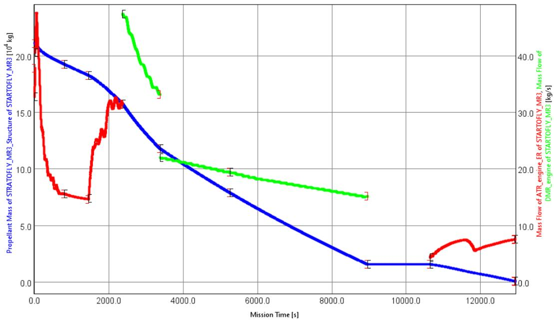
Figure 8.15. Fuel mass and fuel massflow *vs.* Mission Time in the case of oversea final approach (Option B).
