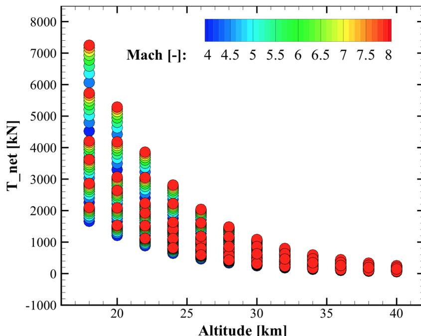
Figure 2.11. DMR performances as a function of altitude and Mach number at different sets of ER and AoA, as used in ASTOS. Credit: [18]
