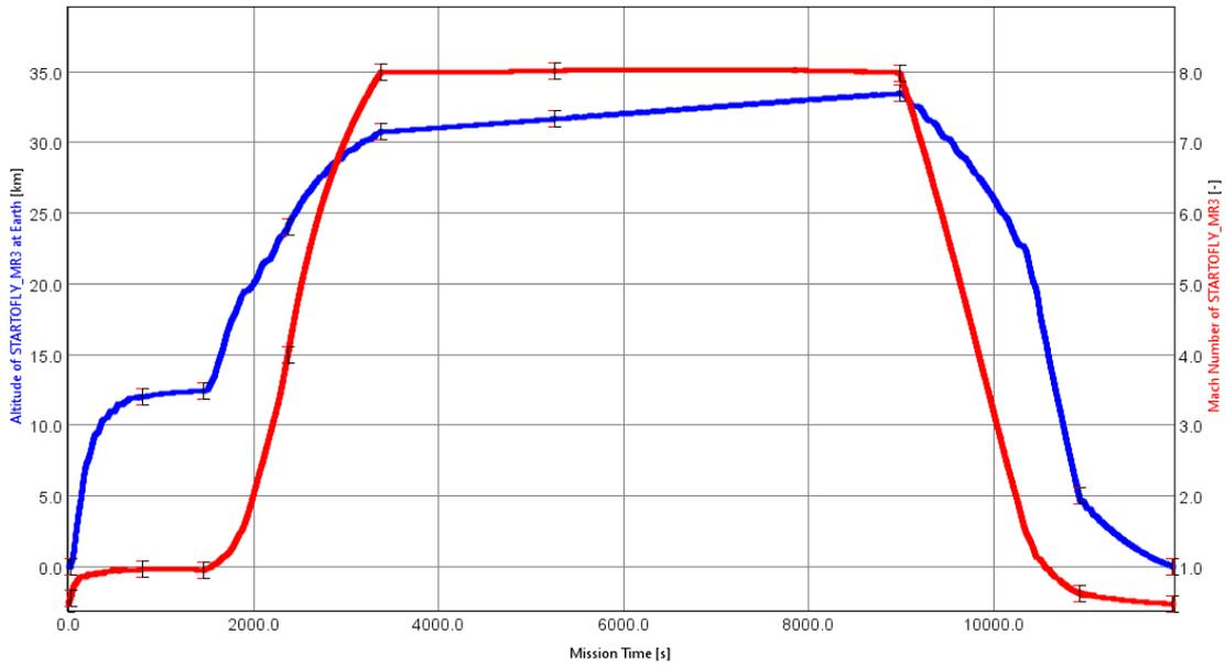
Figure 8.10. Flight Altitude and Flight Mach Number *vs.* Mission Time in the case of overland final approach (Option A).
