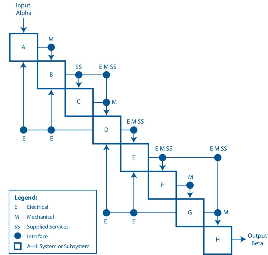
Figure 3.4. Example of a N2 diagram. Credit: [21]
