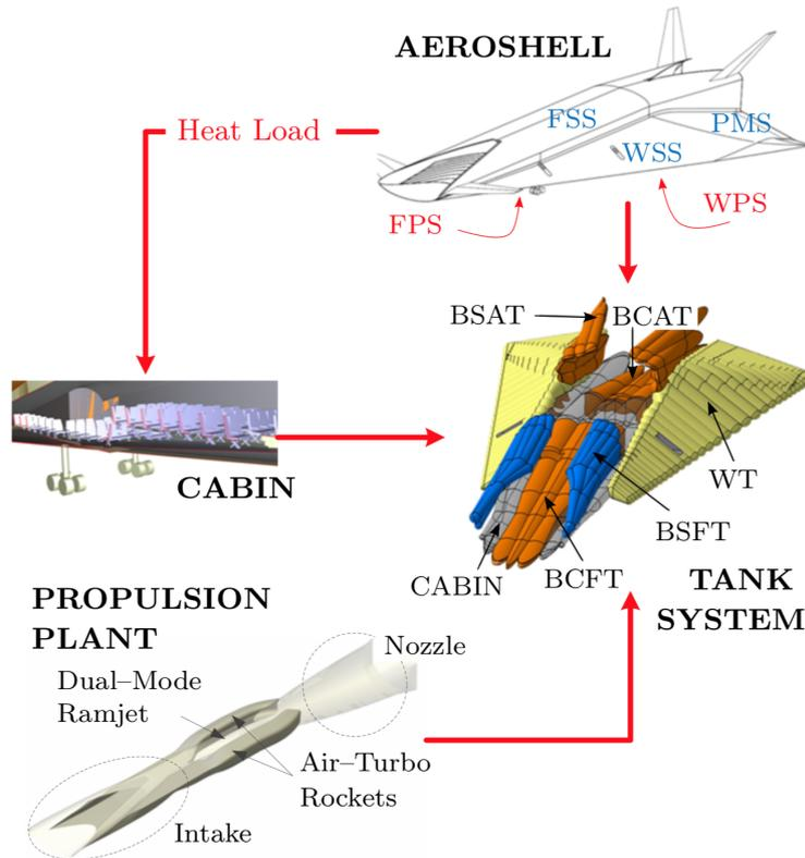
Figure 7.9. Illustration of the cooperation among TEMS, TPS, ECLSS, propellant subsystem and propulsion plant.
