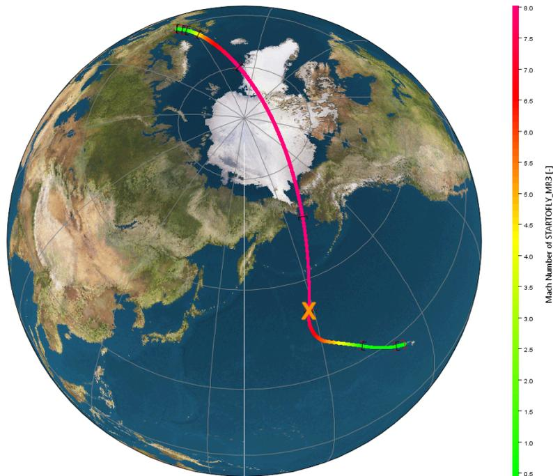
Figure 9.20. Satellite view on the Emergency Landing to Honolulu Airport after a failure occurs during hypersonic cruise to the DMR at mission time  $t = 6356$  s.
