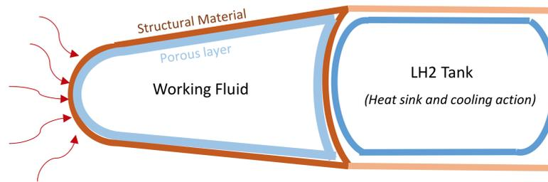
Figure 2.13. Illustration of the heat conduction concept of the Thermal Protection Subsystem. Credit: [12]
