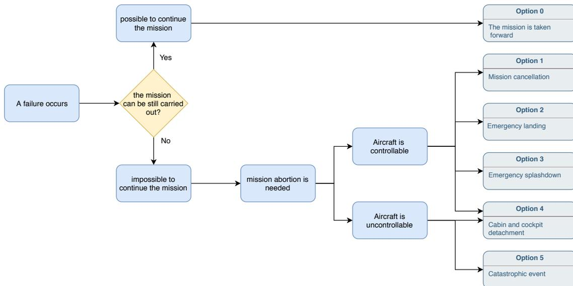
Figure 6.1. Propulsive Subsystem Failure related Consequences.
