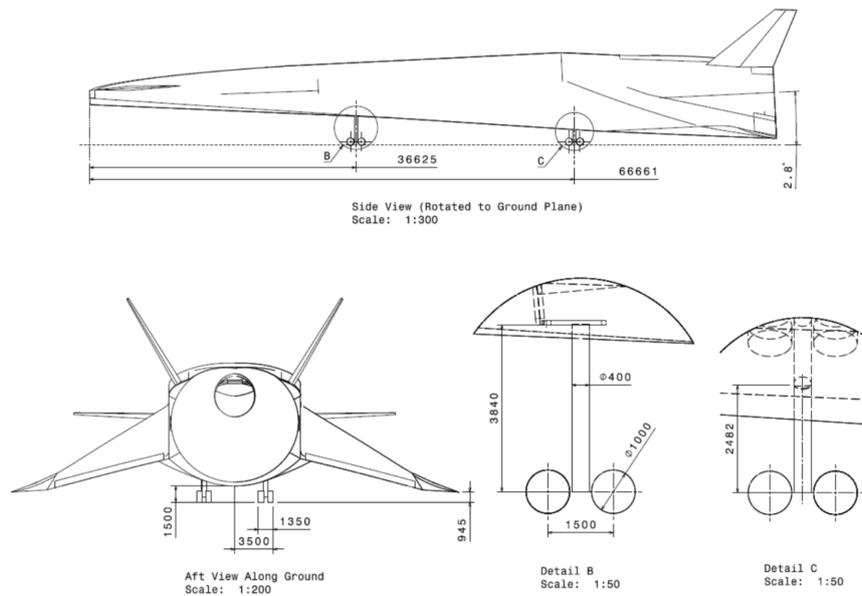
Figure 2.15. LAPCAT MR2 landing gear geometrical characteristics.
