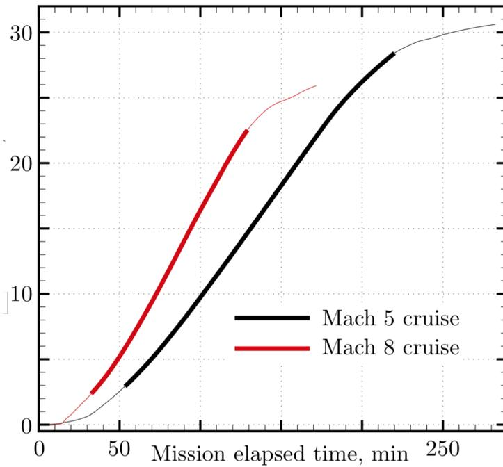
Figure 1.25. The thermal paradox. Integrated heat load vs. mission time for a Mach 5 and a Mach 8 vehicle. Credit: [11]
