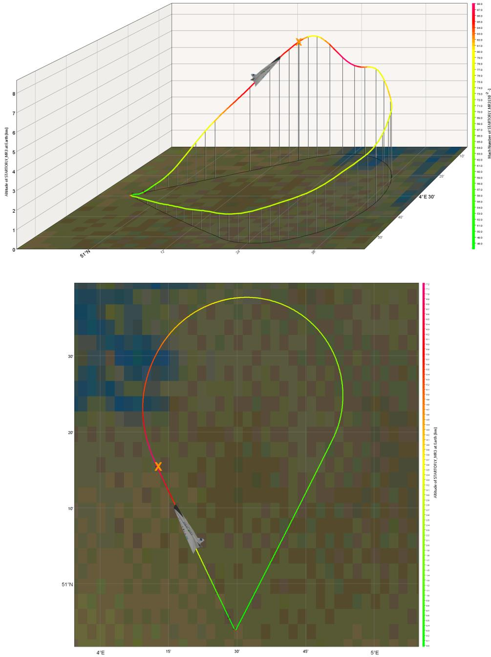
Figure 9.3. Scenario 8: Emergency landing to departure airport after an ATR failure occurs during subsonic cruise. As a consequence, only 1 out of 6 engines is available. (top) 3D view looking in western direction - (bottom) 2D map.
