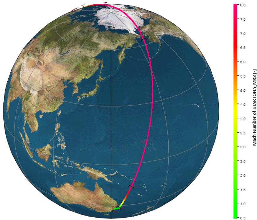
Figure 8.12. View on complete trajectory in the case of oversea final approach (Option B).
