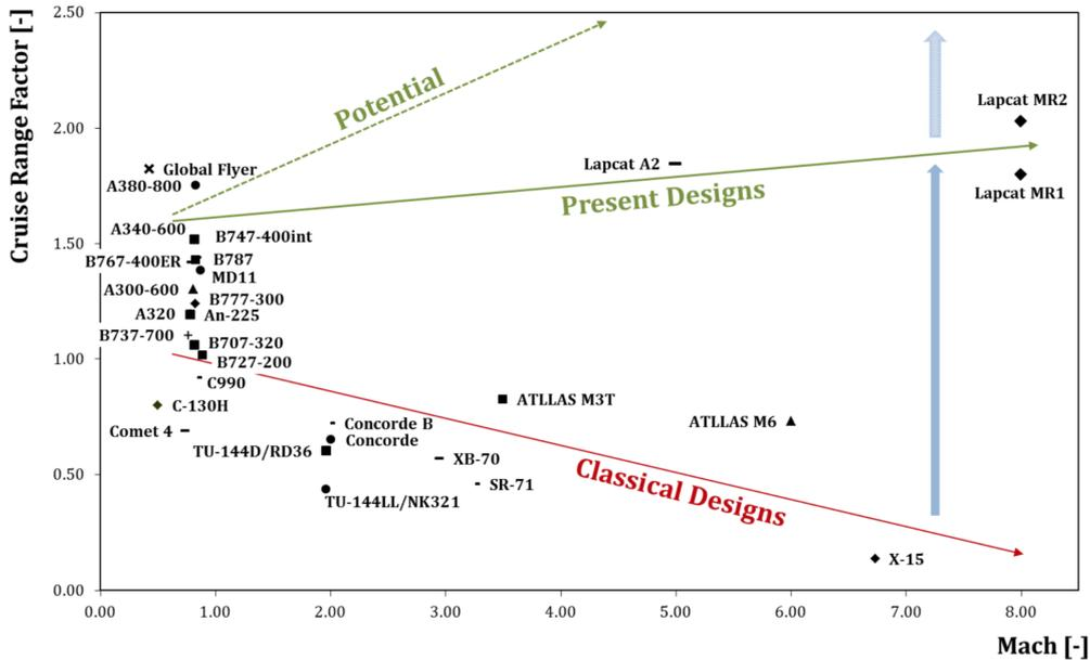
Figure 1.24. Different aircrafts as a function of their Cruise Range Factor and cruise Mach number. Credit: [31]
