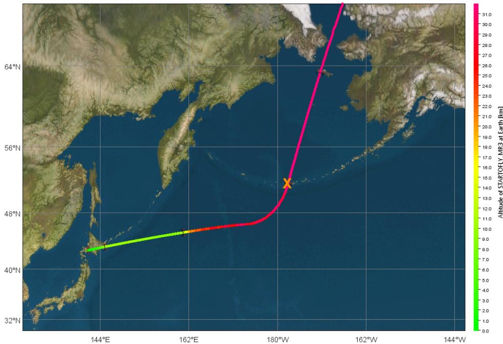
Figure 9.11. 2D trajectory of an Emergency Landing to Sapporo New Chitose Airport after a failure occurs during hypersonic cruise to the DMR at mission time  $t = 5832 s$ .
