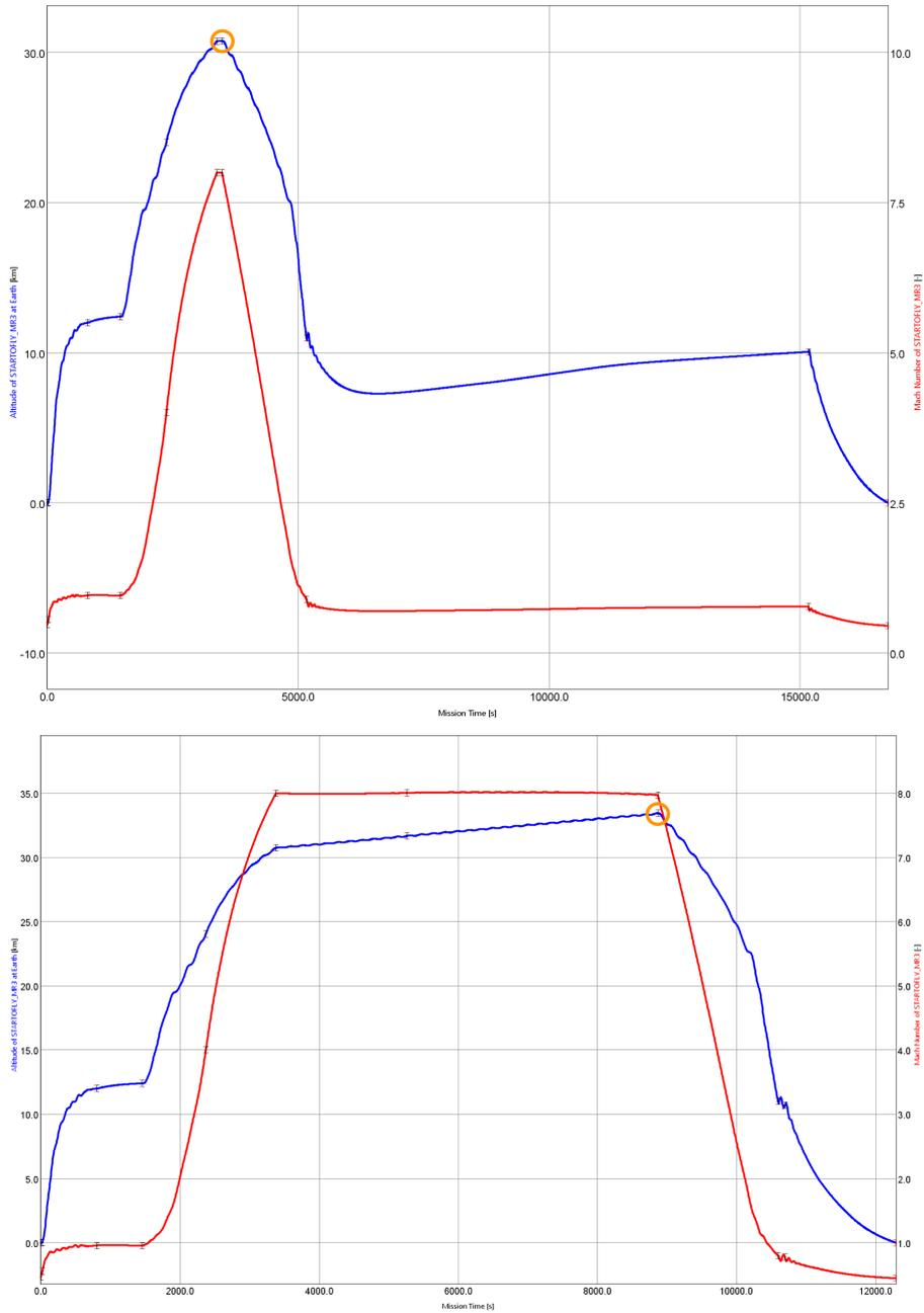
Figure 9.5. Flight Altitude and Flight Mach Number *vs.* Mission Time in the case of a DMR failure occurring (top) at the beginning of hypersonic cruise - (bottom) at the end of hypersonic cruise. The point of failure is highlighted with an orange circle.
