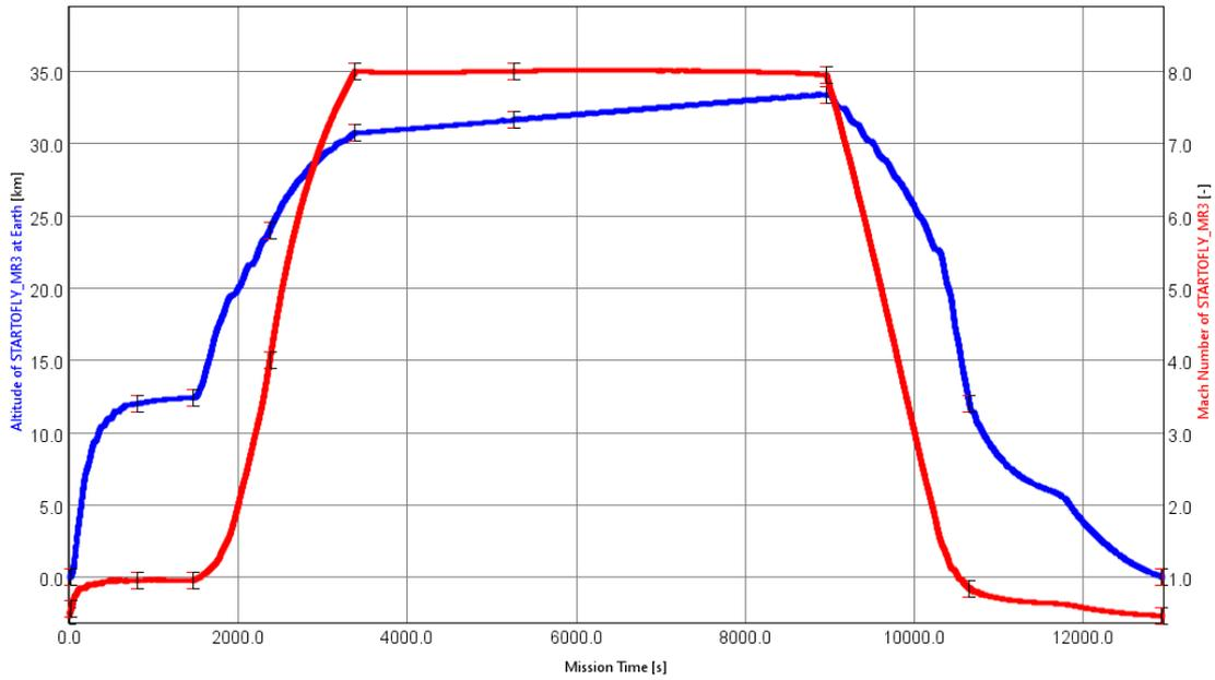
Figure 8.14. Flight Altitude and Flight Mach Number *vs.* Mission Time in the case of oversea final approach (Option B).
