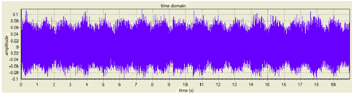
Figure 6.4 Normal working vibration waveform (time domain)
