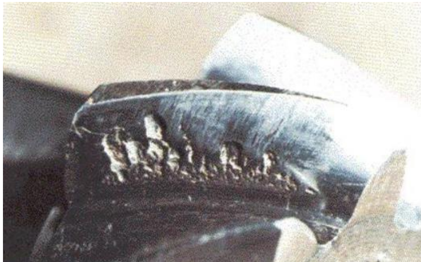
Figure 6.1 tooth surface wear
