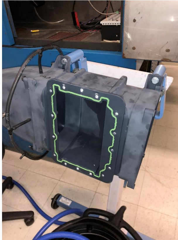
Figure 20: CAC housing test piece for CSB
