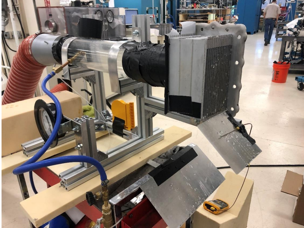
Figure 26: Spray bench with HX attached
