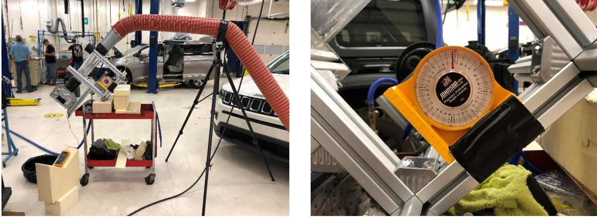
Figure 28: Magnetic protractor fitted to spray bench
