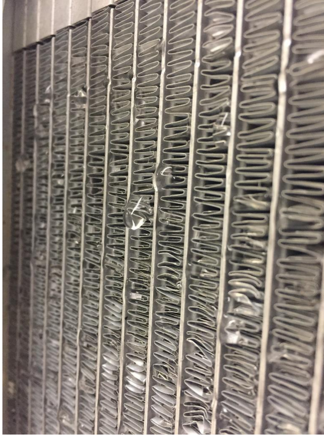
Figure 3: Droplet hanging at the end of the CAC fin
