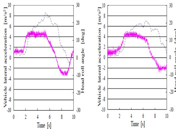
Figure 14: *Head Motion without (left) and with (right) device*
