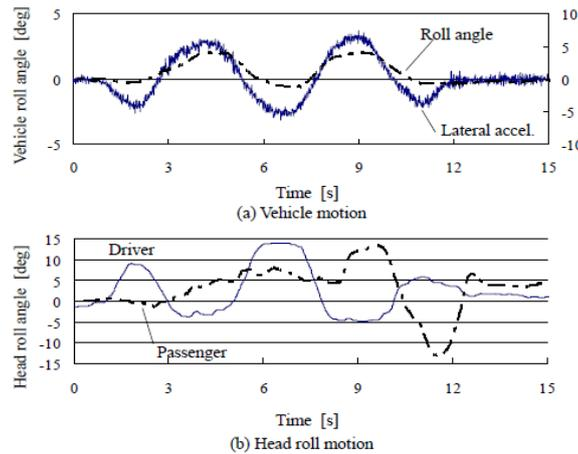
Figure 11: *Hard Condition Head Roll Motion*
