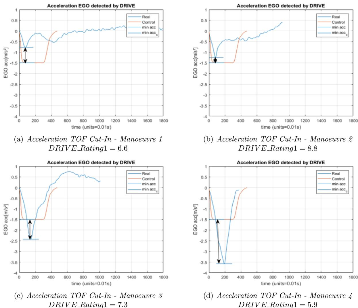
Figure 130: Minimum Acceleration Comparison: TOF free-lane Cut-In
