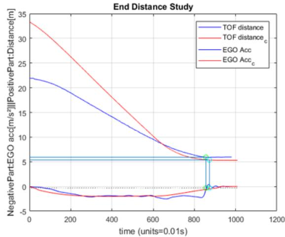
Figure 55: *End-Distance of Follow Vehicle Stop Manoeuvre*
