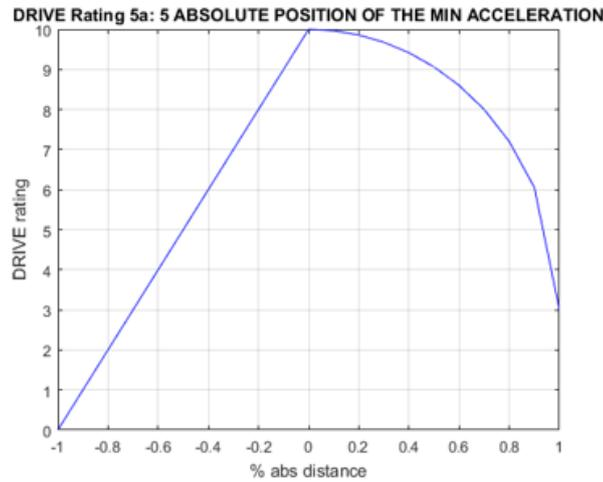
Figure 47: Visualisation of DRIVE Rating 5a in TOF-Approach
