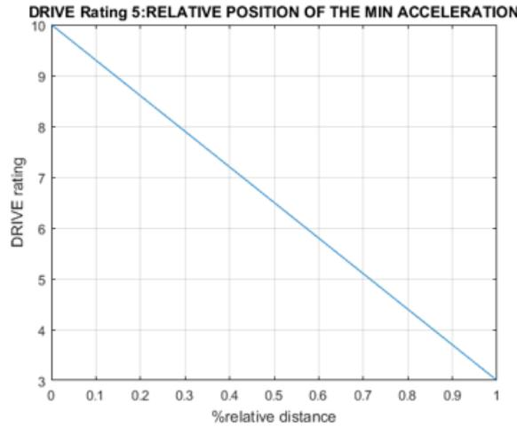
Figure 45: Visualisation of DRIVE Rating 5 in TOF-Approach
