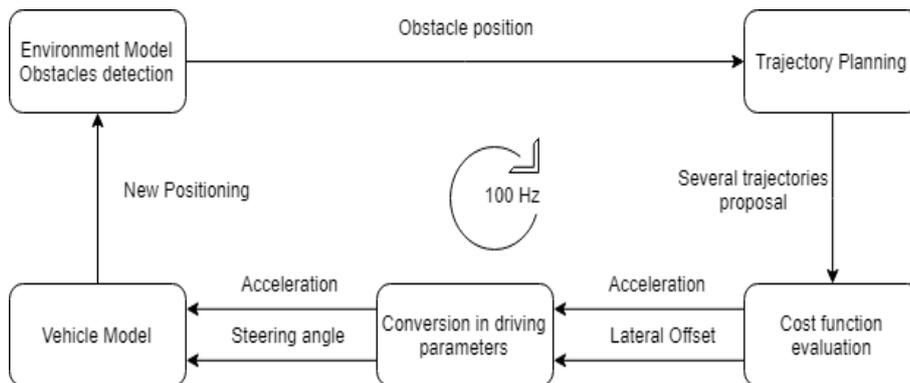
Figure 22: *Controller Logic*
