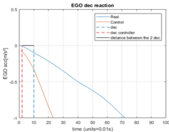
(c) Response Delay TOF Cut-In - Manoeuvre 3
