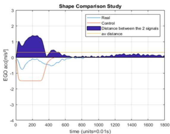
(a) Acceleration Shape TOF Cut-In - Manoeuvre 1
