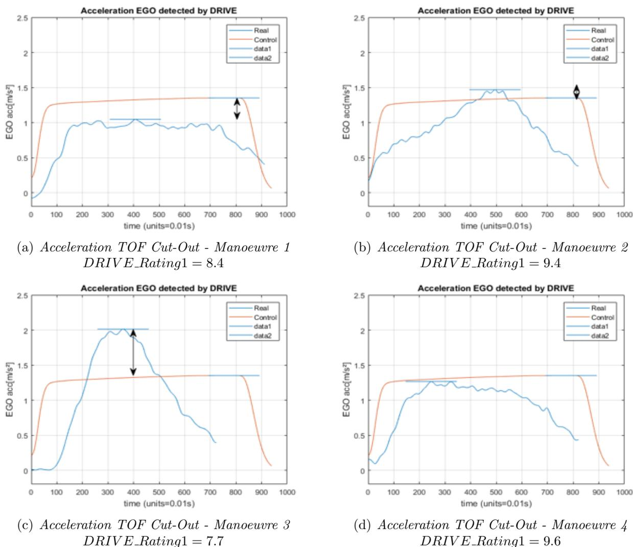
Figure 122: Maximum Acceleration Comparison: TOF free-lane Cut-Out low speed
