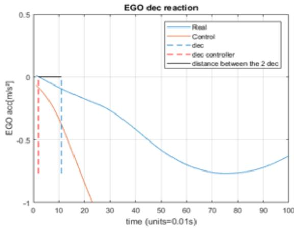
(a) Response Delay TOF Cut-In - Manoeuvre 1
