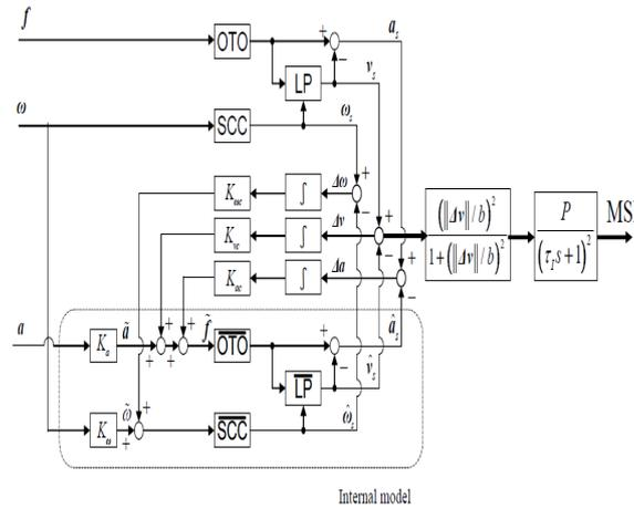
Figure 9: *Motion Sickness controller*
