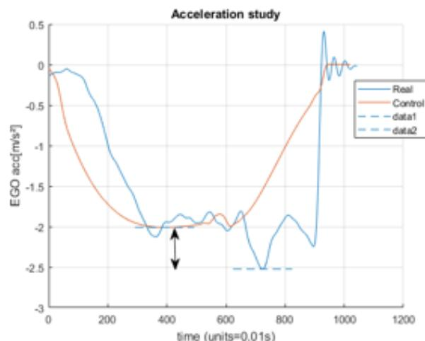
Figure 53: Ego Acceleration of Follow Vehicle Stop Manoeuvre: Minimum Acceleration Study
