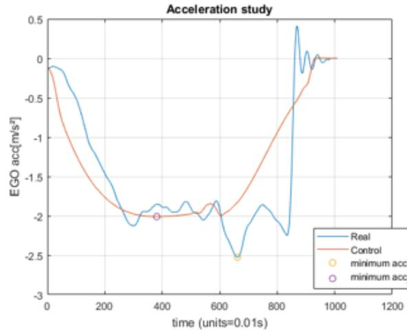
Figure 59: *Relative Position of the Minimum Acceleration of Follow Vehicle Stop Manoeuvre*
