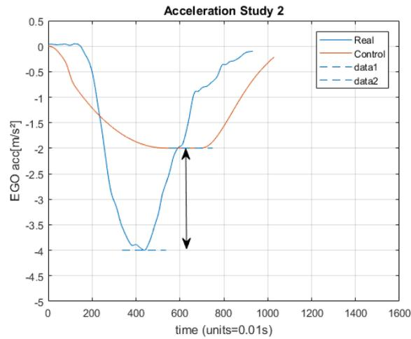
Figure 33: *Ego Acceleration of TOF-Approach Manoeuvre: Minimum Acceleration Study*
