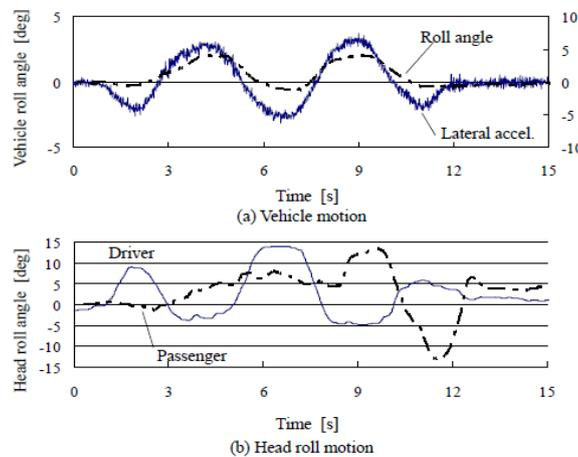
Figure 10: *Mild Condition Head Roll Motion*
