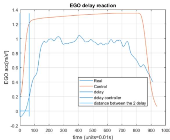
Figure 71: *TOF free-lane Cut-Out Manoeuvre: Response Delay*
