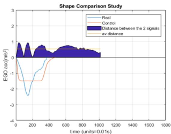
(c) Acceleration Shape TOF Cut-In - Manoeuvre 3
