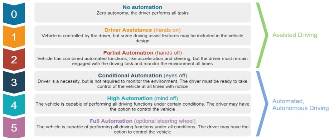
Figure 1: Table with SAE Automation Levels
