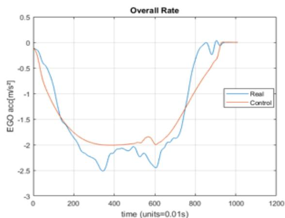
(d) *Manoeuvre 4 - Overall DRIVE\_Rating = 8.6*Figure 109: *Relative Position Analysis Comparison: Follow Vehicle Stop*
