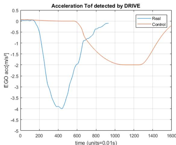
Figure 32: *Ego Acceleration of TOF-Approach Manoeuvre detected by AVL-DRIVE<sup>TM</sup>*
