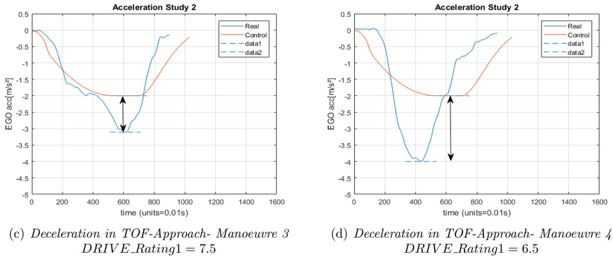
Figure 86: *TOF-Approach Low Speed: Minimum Acceleration Comparison*
