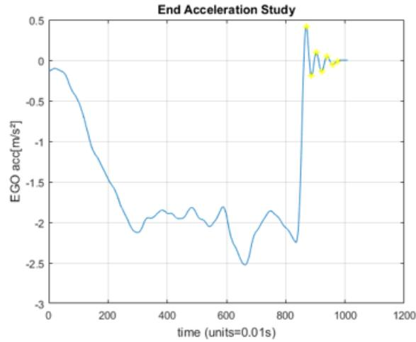
Figure 58: *End-Acceleration Analysis of Follow Vehicle Stop Manoeuvre*
