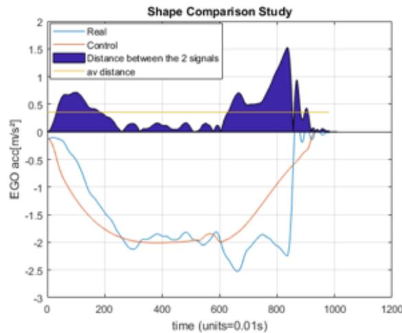
Figure 57: Acceleration Shape Comparison of Follow Vehicle Stop Manoeuvre
