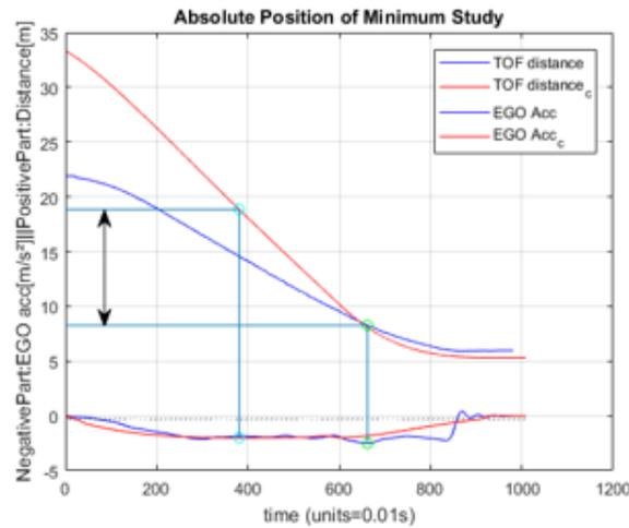
Figure 60: *Absolute Position of the Minimum Acceleration of Follow Vehicle Stop Manoeuvre*
