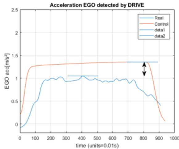
Figure 70: *TOF free-lane Cut-Out Manoeuvre: Maximum Acceleration*
