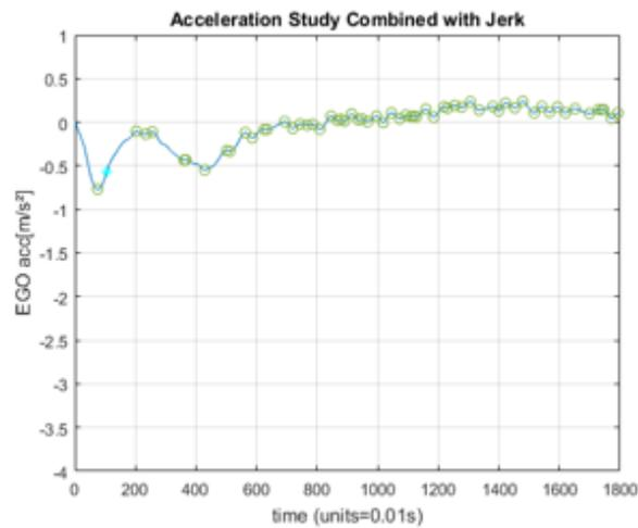
Figure 78: *TOF free-lane Cut-In Manoeuvre: Jerk Gradient Evaluation*
