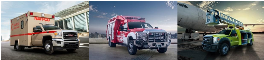
Fig70 Example of transformation on Heavy duty chassis by NAFFCO. From left to right: Ambulance, Firefighting vehicle, Aerial rescue vehicle.
