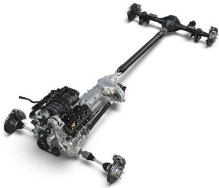
Fig14 2019 Ram 1500 powertrain scheme
