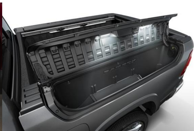
Fig17 RamBox cargo management system
