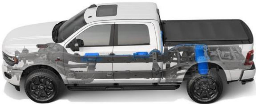
Fig22 2019 Ram 2500 air suspension
