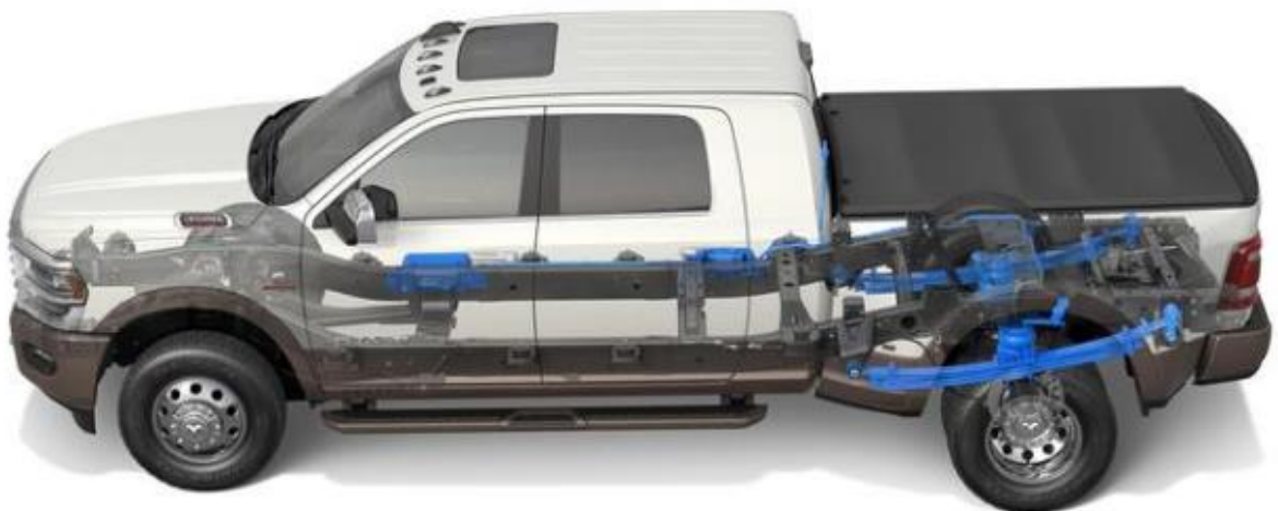
Fig23 2019 Ram 3500 with combined air suspension
