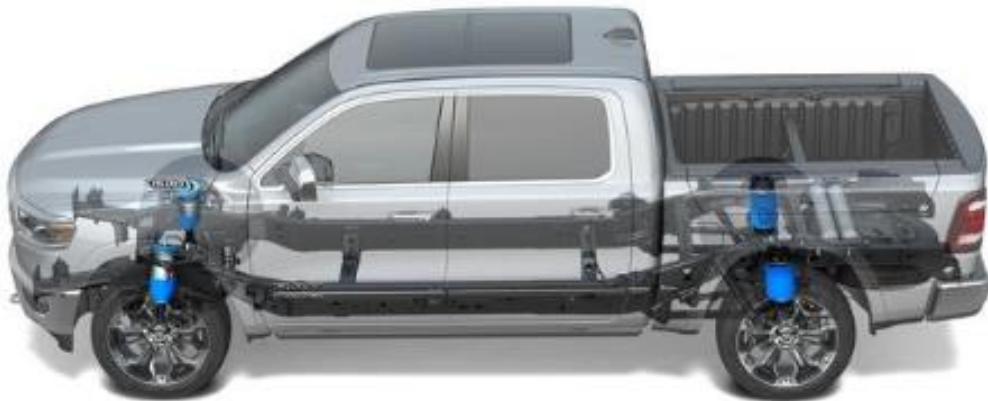
Fig12 2019 Ram 1500 Air suspension
