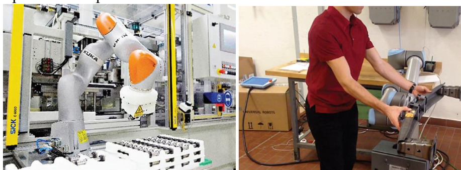
Figure 2.6 Collaborative robots in SKODA AUTO-KUKA LBR iiwa[3]
