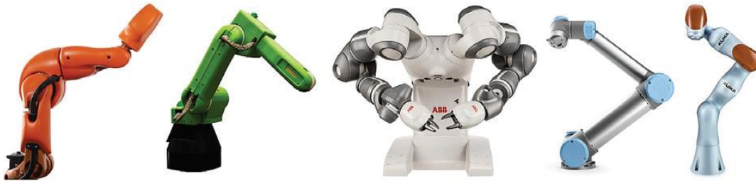
Figure 2.11 Collaborative robots – MRK-Systeme KR SI, Fanuc CR-35iA, ABB YuMi, UR5, KUKA LBR iiwa
