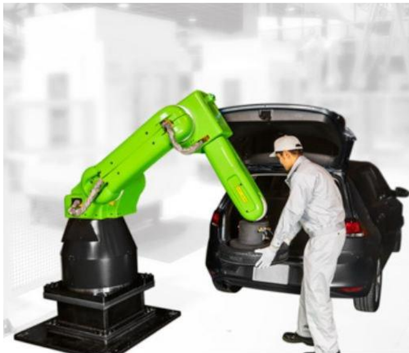
Figure 2.8 Hand Guiding Method[6]
