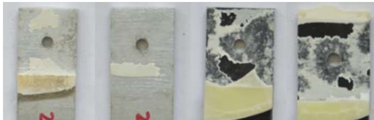
Figure A-5: FM of Uralane bonded-only DLJs - 22 cycles
