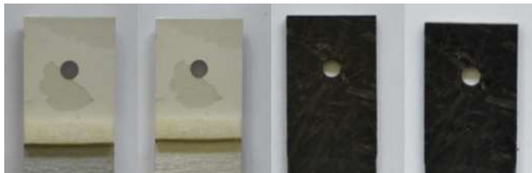
Figure A-1: FM of Uralane bonded-only DLJs - 0 cycle
