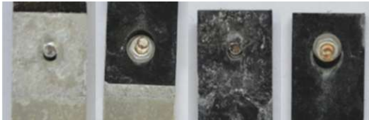
Figure A-15: FM of bolted-only DLJs - 7 cycles
