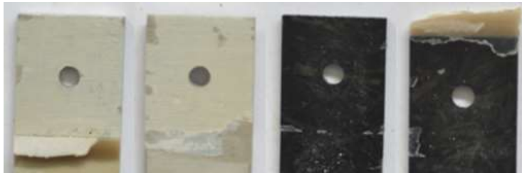
Figure A-12: FM of Epibond bonded-only DLJs - 30 cycles
