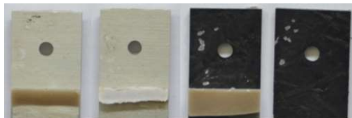
Figure A-10: FM of Epibond bonded-only DLJs - 14 cycles
