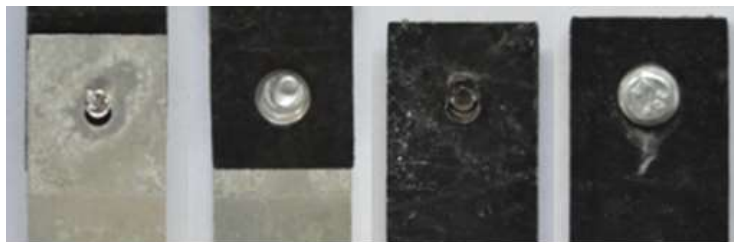
Figure A-14: FM of bolted-only DLJs - 1 cycle
