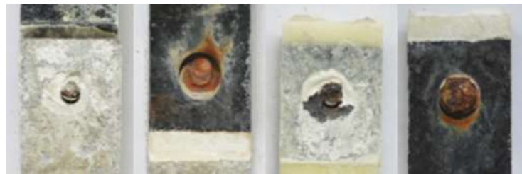
Figure A-24: FM of hybrid bonded/bolted DLJs - 30 cycles
