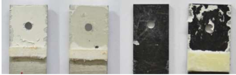
Figure A-3: FM of Uralane bonded-only DLJs -7 cycles
