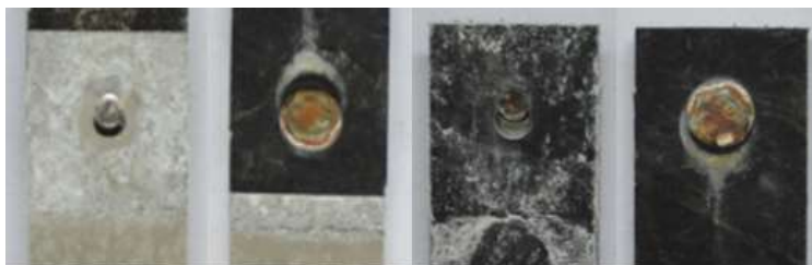
Figure A-16: FM of bolted-only DLJs - 14 cycles
