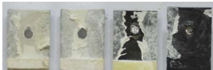
Figure A-22: FM of hybrid bonded/bolted DLJs - 14 cycles
