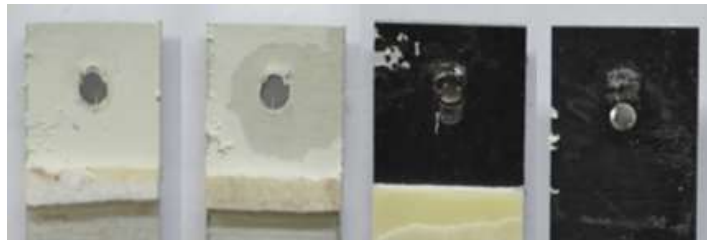
Figure A-20: FM of hybrid bonded/bolted DLJs - 1 cycle
