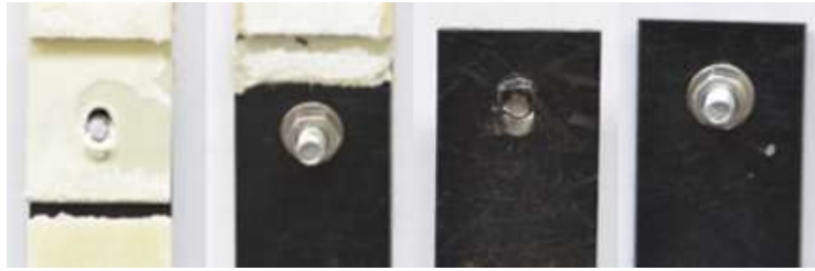
Figure A-19: FM of hybrid bonded/bolted DLJs - 0 cycle
