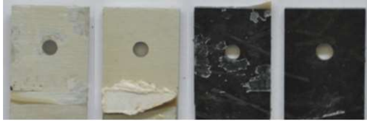
Figure A-11: FM of Epibond bonded-only DLJs - 22 cycles
