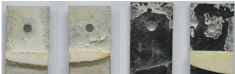
Figure A-4: FM of Uralane bonded-only DLJs – 14 cycles
