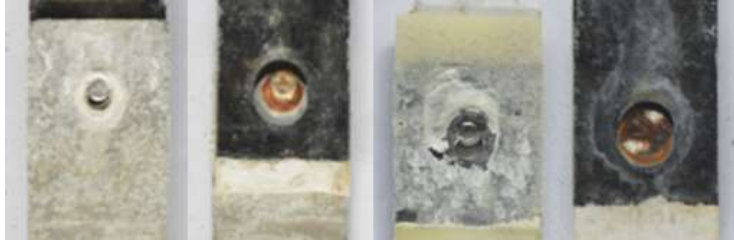
Figure A-23: FM of hybrid bonded/bolted DLJs - 22 cycles
