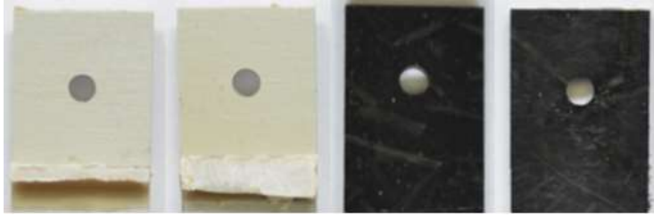
Figure A-7: FM of Epibond bonded-only DLJs - 0 cycle
