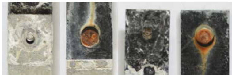
Figure A-18: FM of bolted-only DLJs - 30 cycles
