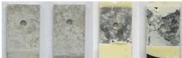
Figure A-6: FM of Uralane bonded-only DLJs - 30 cycles
