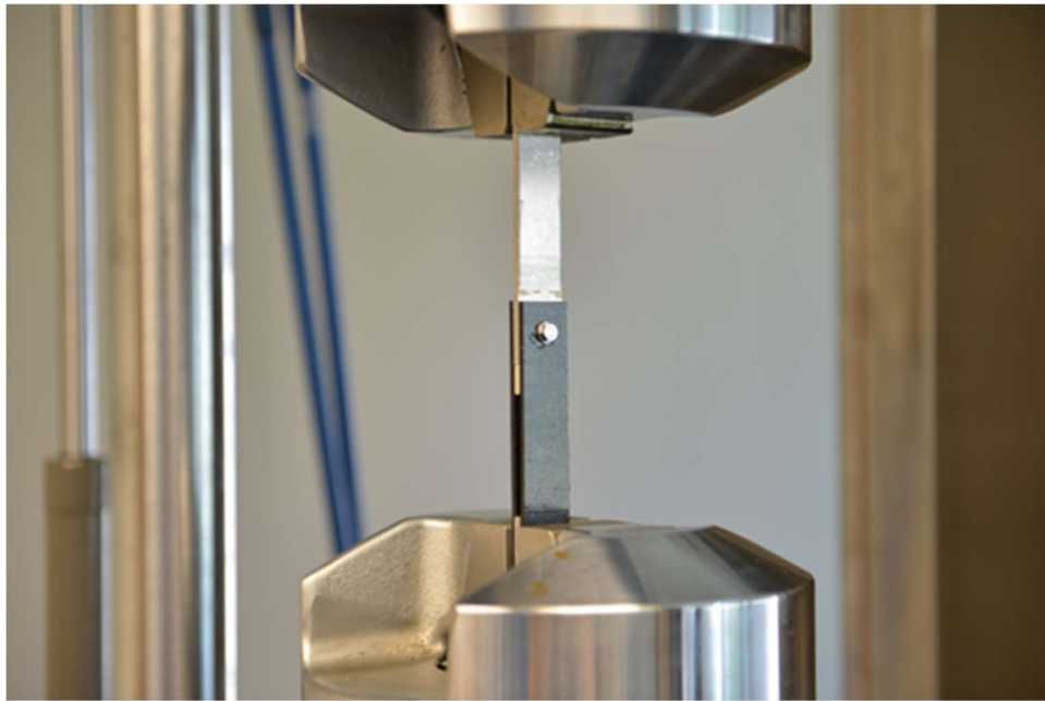
Figure 2-8: Hybrid bonded/bolted DLJs under tensile test
