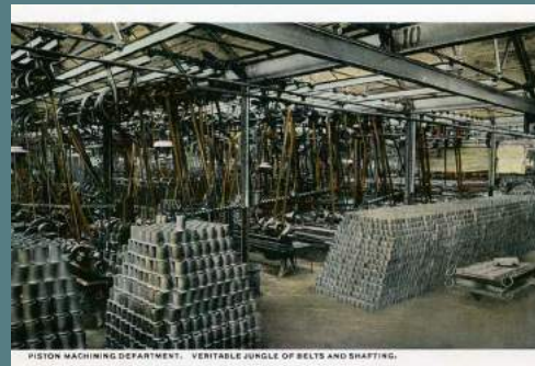
PISTON MACHINING DEPARTMENT. VERITABLE JUNGLE OF BELTS AND SHAFTHING.
