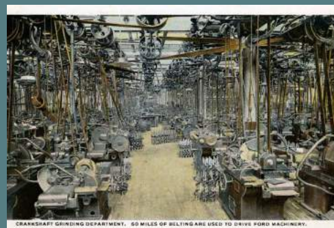
CRANKSHAFT GRINDING DEPARTMENT, 60 MILES OF BELTING ARE USED TO DRIVE FORD MACHINERY.
