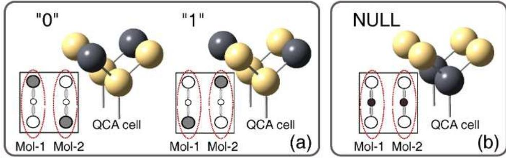
Figure 1.2: Six quantum dots molecular QCA cell scheme.(a) '0' and '1' logic state (b) 'NULL' state with charge in the third dots [3].
