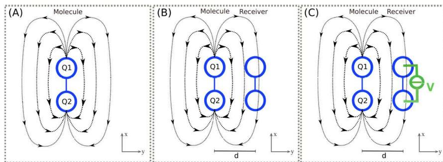
Figure 2.1: Definition of electric field generated by a molecule and obtained voltage at the receiver.
