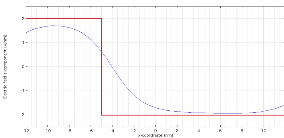
Figure 6.2: Trend of the obtained electric field inside the trench of the wire during the first phase (blue line). The red line represents the ideal behaviour in which all the molecules of a clock zone are subject to the same values of electric field.
