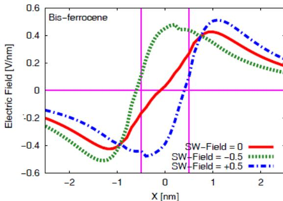
Figure 2.2: Electric field at the receiver calculated in equilibrium condition and with a positive and negative applied switching field [26].
