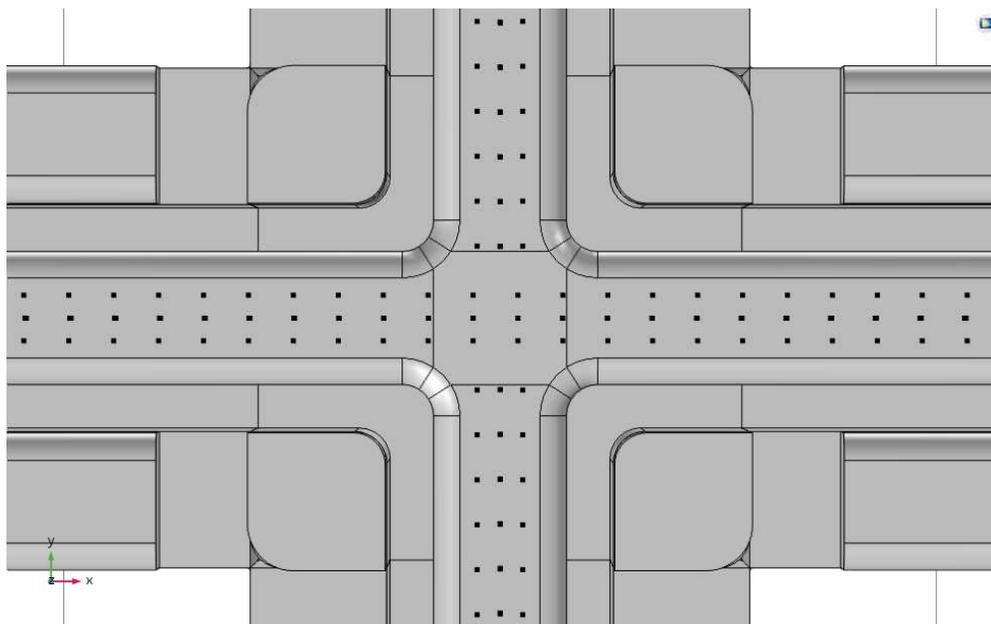
Figure 6.10: Top view of the majority voter central region in the structure where the realization of the electrodes required a resolution equal to 3 nm.
