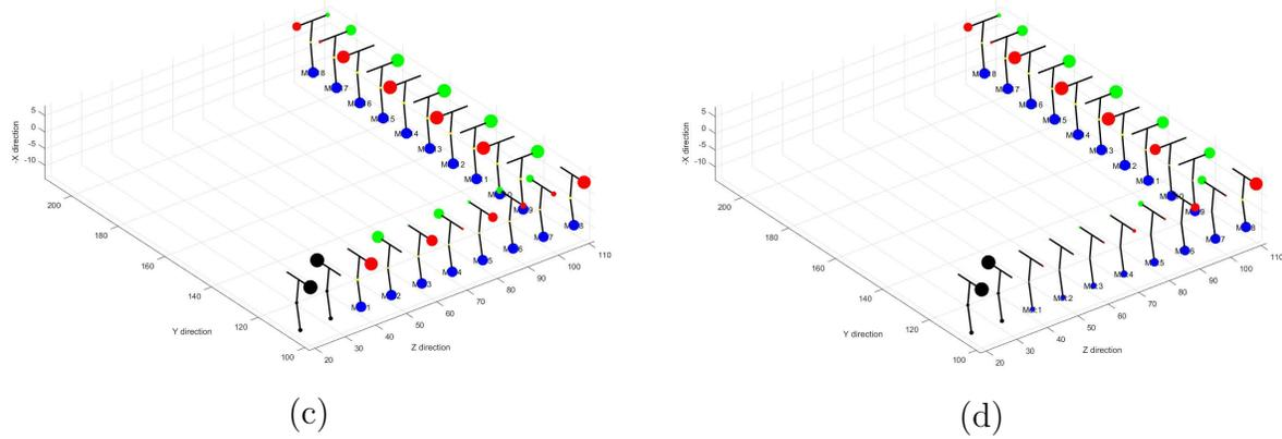
Figure 6.18: Propagation of the information in the angle structure without the molecular QCA cell at the end of the input binary wire.
