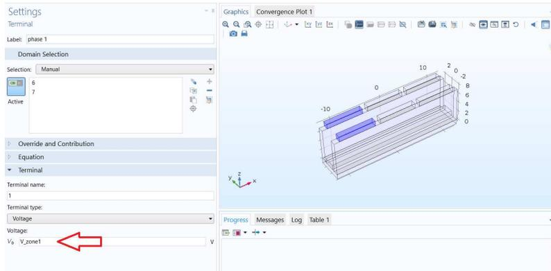
Figure 4.3: Physics and settings to associate to the first clock zone of the binary wire the correct voltage value. For the others two the same procedure has been followed changing the domain selected.
