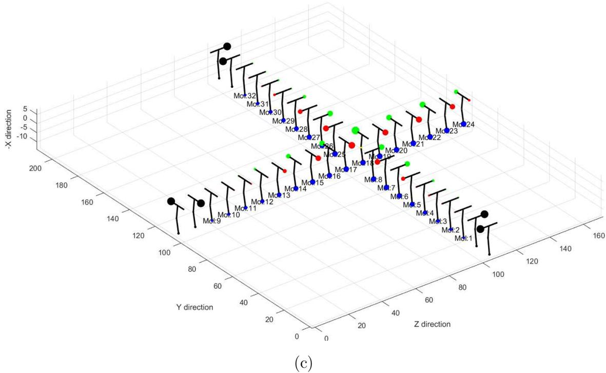
Figure 6.12: Propagation in the majority voter with the larger structure; inputs logic values equal to top=1, center=0 and bottom=1 so the correct output values is equal to 1. (a) first phase, (b) second phase, (c) third phase.
