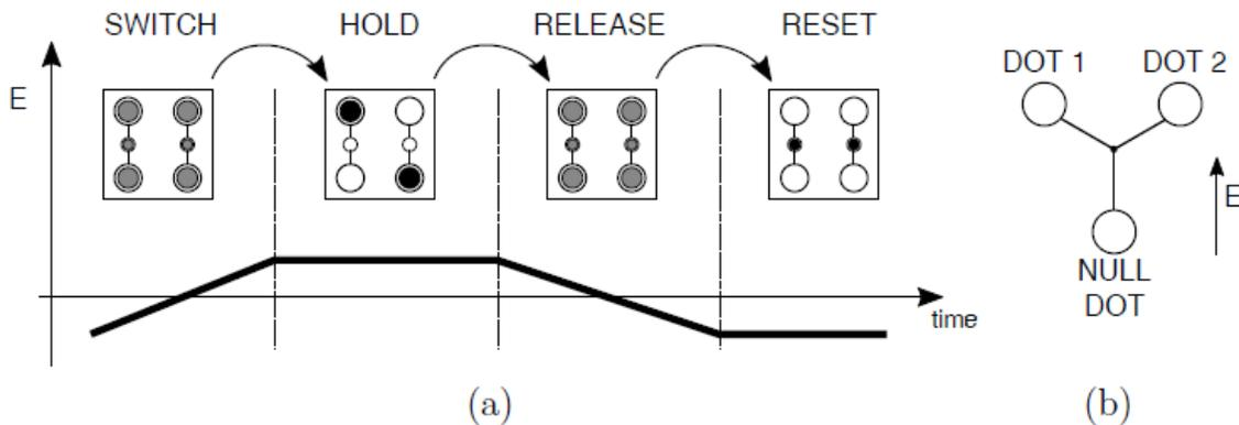
Figure 1.7: Clock phase definition and resulting effect on the molecular QCA cell. (a) Sequence of the phases in the various instants of time. (b) Representation of the bis-ferrocene molecule with electric field vector.
