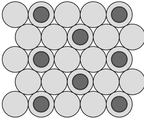
Figure 1.10: Organization of Sulphur atoms, in dark grey, on Au(111) in grey. The ratio between gold and sulphur atoms is 3:1.
