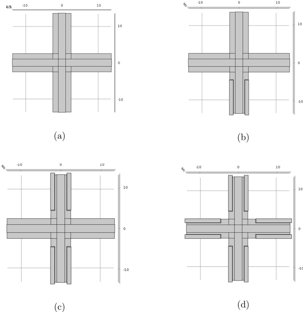
Figure 4.6: Steps for the creation of the side dielectrics (top views). (a) Crossroad formed by the bottom electrode and the bottom dielectric; (b) creation of two sides dielectric; (c) exploiting the function *Mirror* with the origin as point of reflection, the dielectric on the other side has been realized; (d) the function *Rotate* is used to generate the others two rotating the firsts of 90 degrees.
