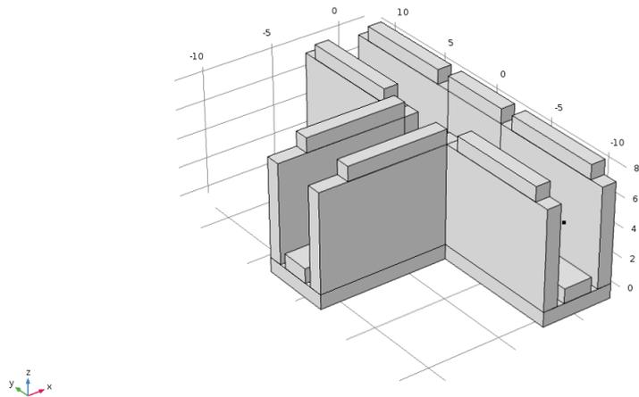
Figure 4.10: Geometry used for the Comsol simulation of the T structure (prospective view).
