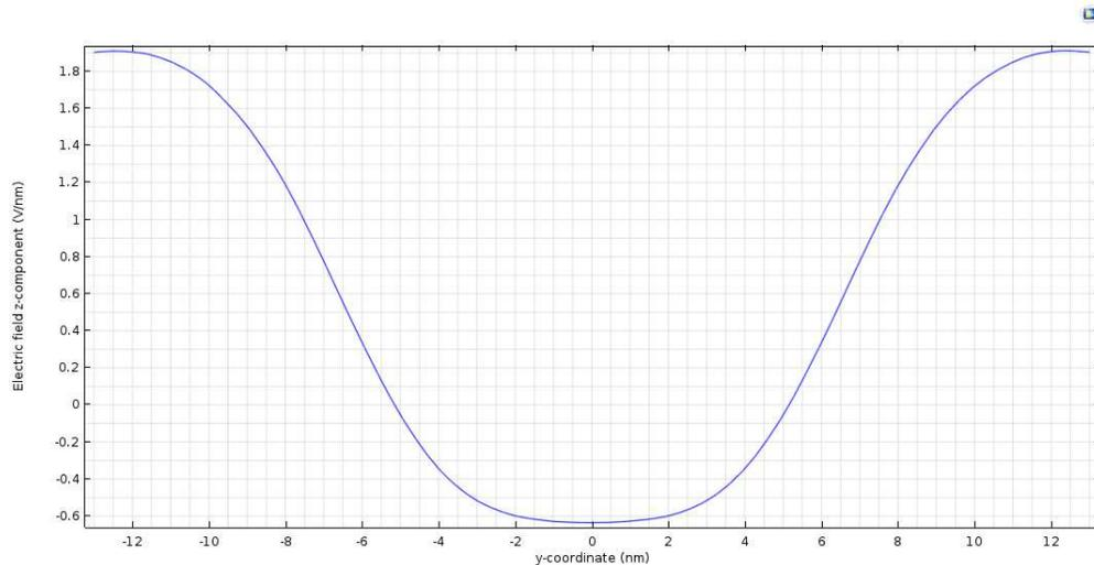
Figure 6.11: Trend of the electric field inside the trench of the majority voter with larger trench during the first phase when the inputs are switched on.
