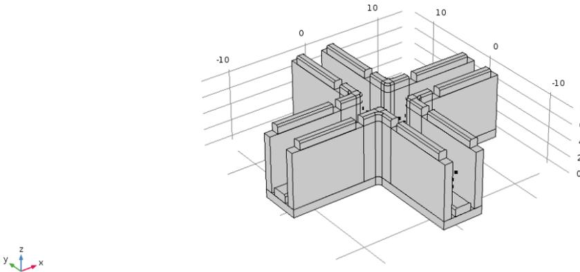
Figure 4.7: Geometry used for the Comsol simulation of the majority voter in the ideal case (prospective view).
