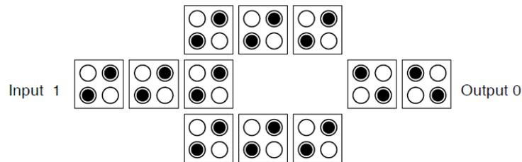
Figure 1.4: Cells placement for inverter structure.
