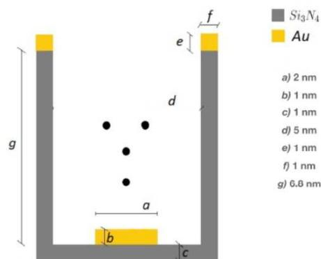
Figure 1.8: Section of the structure used for the realization of the trench in molecular QCA.
