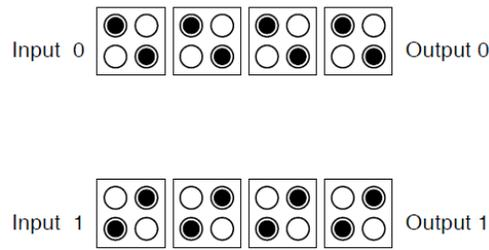
Figure 1.3: Cells placement for binary wire structure.
