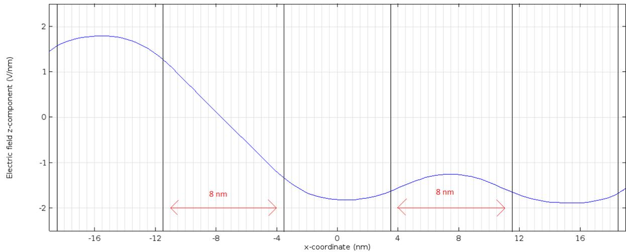
Figure 6.5: Trend of the electric field in the binary wire with the gap equal to 8 nm during the first phase of the propagation.
