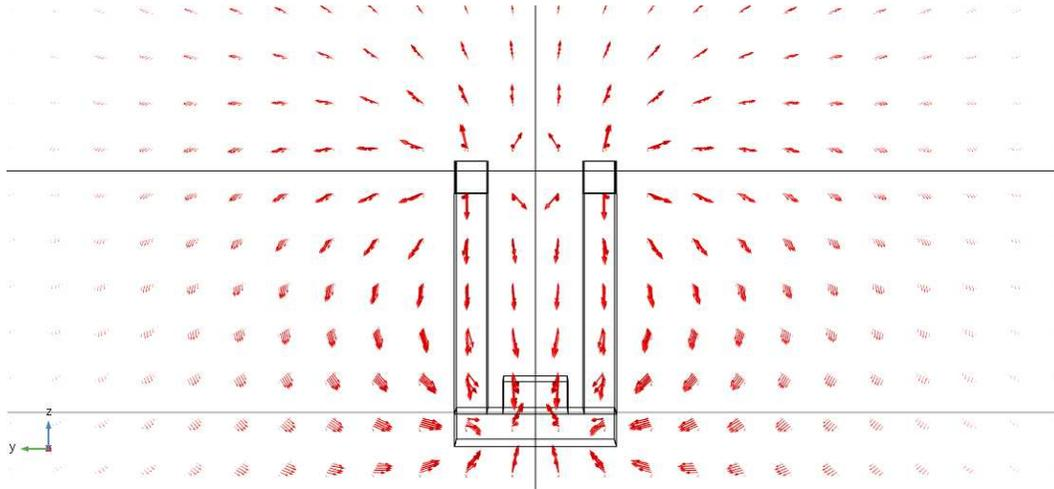
Figure 6.1: Field lines generated by the electrodes in the trench of a wire. The applied voltage in this case is positive so they are oriented towards the bottom.
