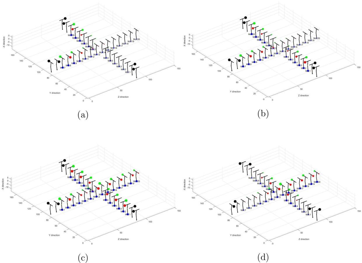
Figure 6.9: Complete propagation in the majority voter with one input delayed in the second approach. The input values are top=1, center=0, bottom=1. (a) the bottom input remains off while the others two are on, in order to simulate the delay. (b) all the inputs are switched on but no logic value is present in the central cell. (c) the central cell and the output are switched on and the computation is performed. (d) the inputs are switched off.
