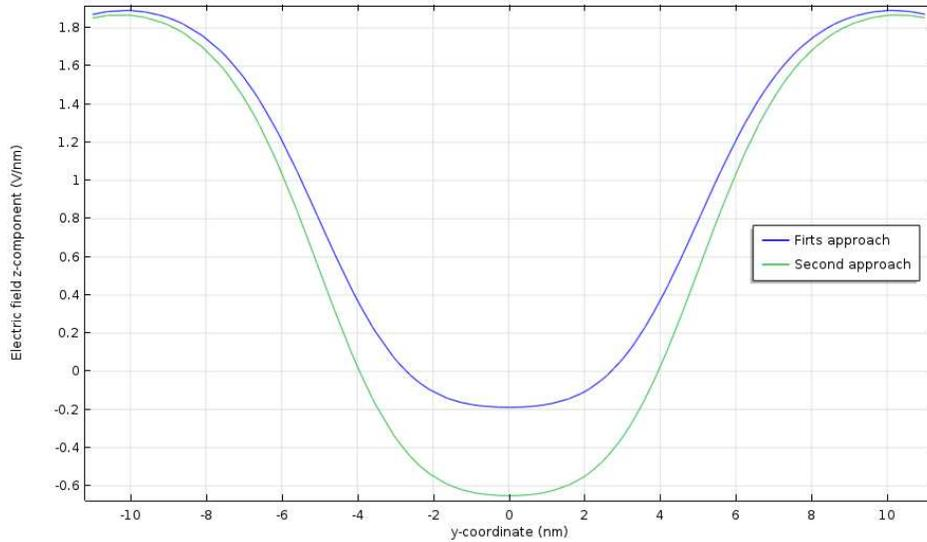
Figure 6.7: Trend of the electric field inside the trench of the majority voter in the two approaches described during the first phase in which the inputs are switched on; blue line first approach, green line second approach.
