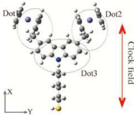
Figure 1.6: Bis-ferrocene molecule structure [8].
