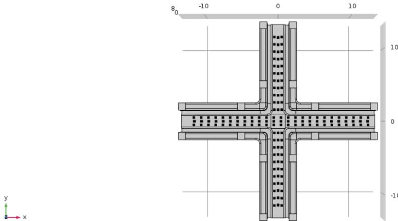
Figure 4.8: Geometry used for the Comsol simulation of the majority voter in the ideal case (top view).
