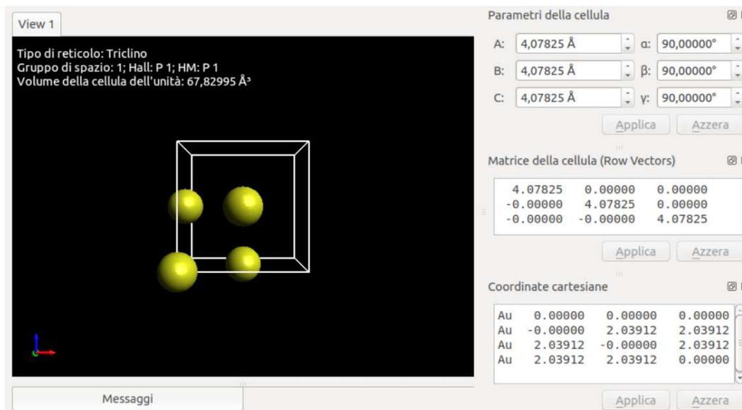
Figure 8.1: Unit cell of the Au slab created with Avogadro.
