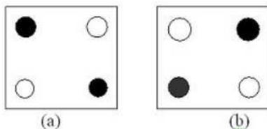
Figure 1.1: QCA cell possible configurations with black dot associated to a negative charge and white ones associated to a positive charge. (a) logic state '0' (b) logic state '1'.
