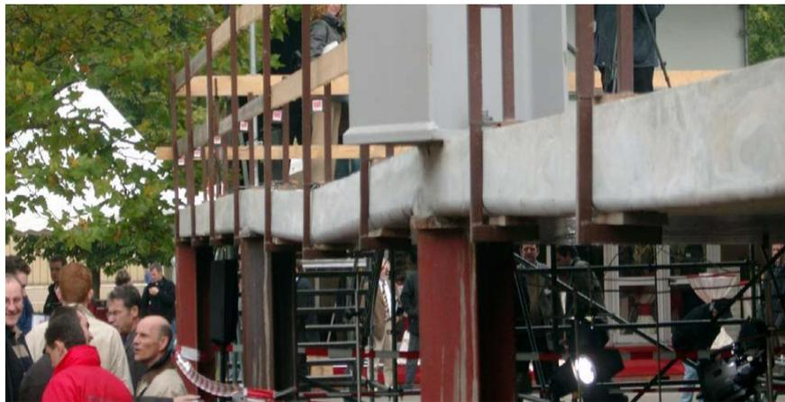
Figure 21: Deformed slab after loading of an edge field [9]
