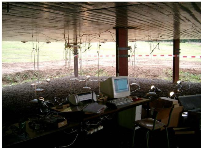
Figure 17: Application of displacement transducers beneath the slab [9]
