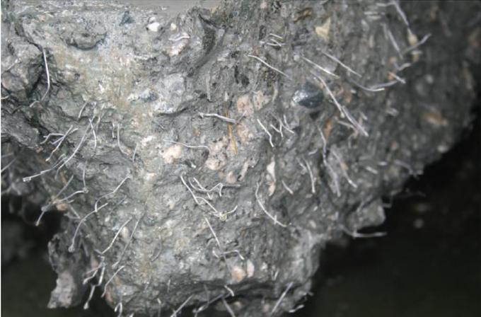
Figure 6: Fracture surface of steel fibre-reinforced concrete [3]
