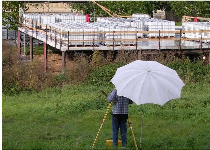
Figure 18: Uniformly distributed load on the HRFA full-scale forging test at Bissen, 2004.[9]
