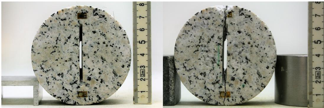
Figure 4.31: Picture of G4 sample (400° C) before and after the test
