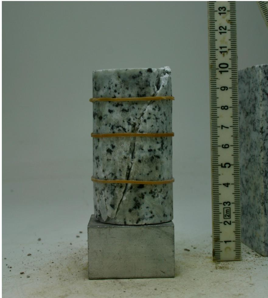
Figure 3.13: Photo of the specimen after the triaxial test
