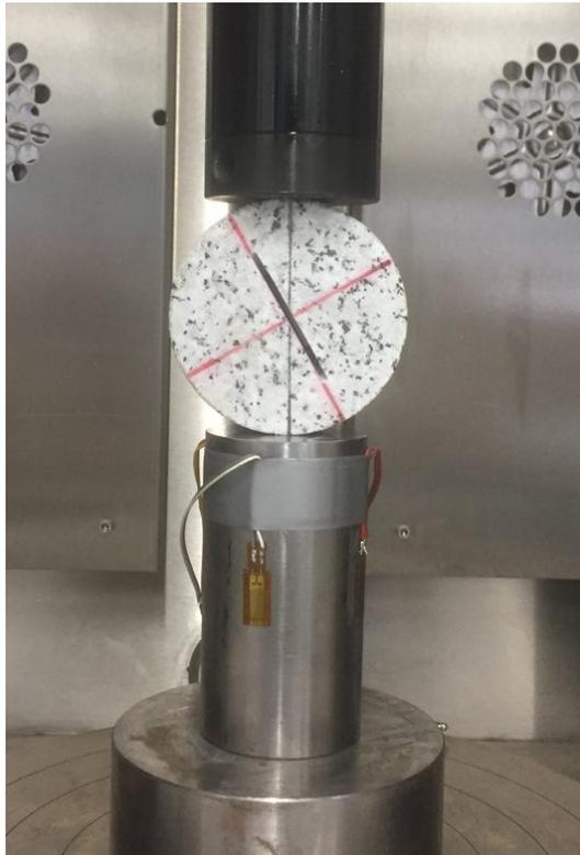
Figure 4.49: G1 sample during the mode II fracture toughness test
