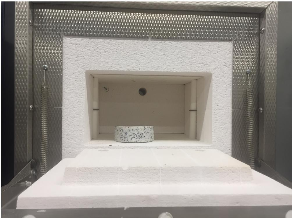
Figure 4.2: CCNBD sample into the oven ready for the thermal treatment
