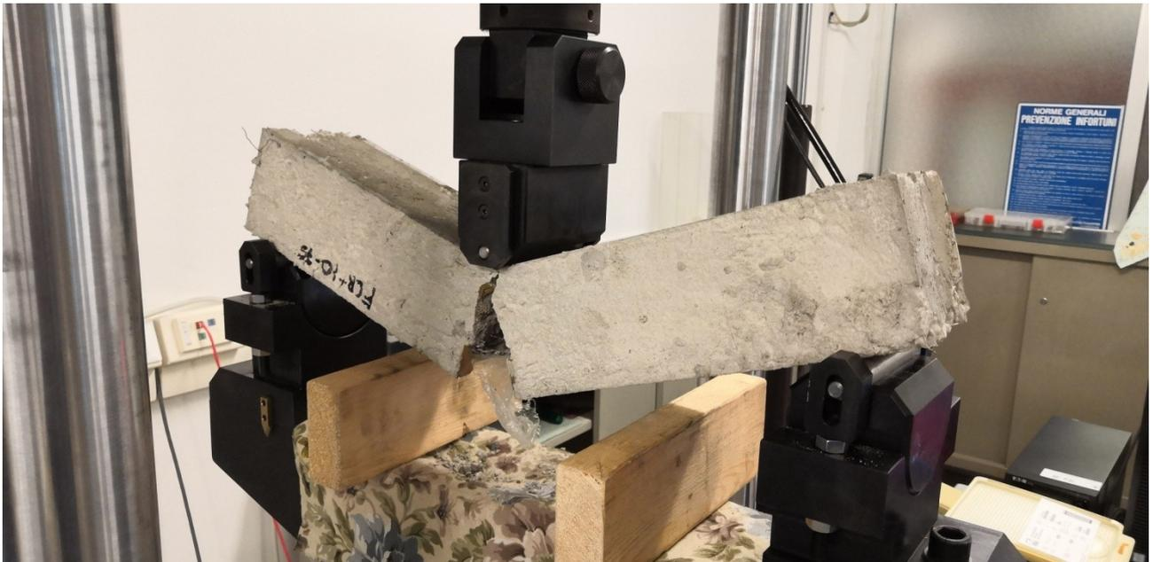
Figure 3.7: Failure of the specimen
