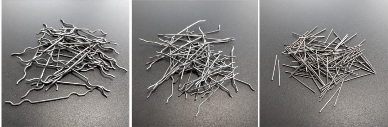
Figure 3.2: Detail of the steel fibers adopted for the experimentation, from left to right: READYMESH MX-500, READYMESH MS-350 and READYMESH MM-150
