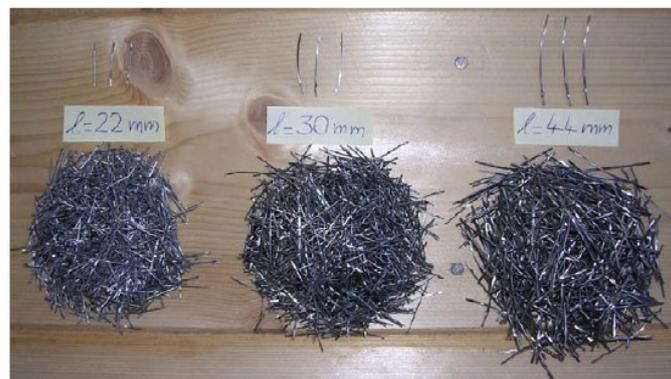
Figure 2.10: Steel fibers adopted for the experimentation
