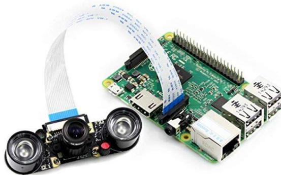
*Figure 9.17: night vision camera connected to Raspberry Pi*
