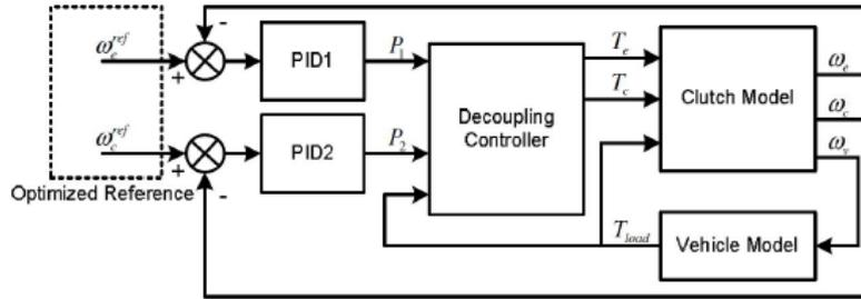
Figure 2.7: Scheme of decoupling control implemented in [3].
