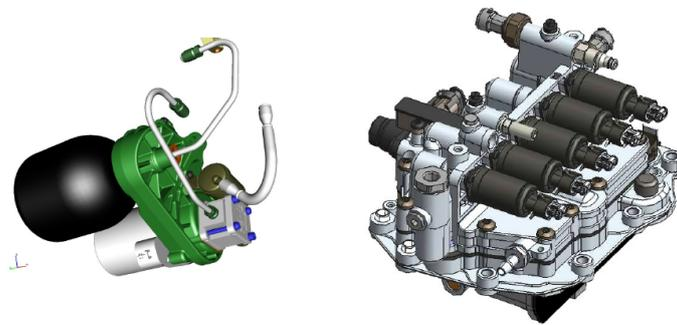
Figure 2.3: Hydraulic Power Unit and Complete Actuation Module.
