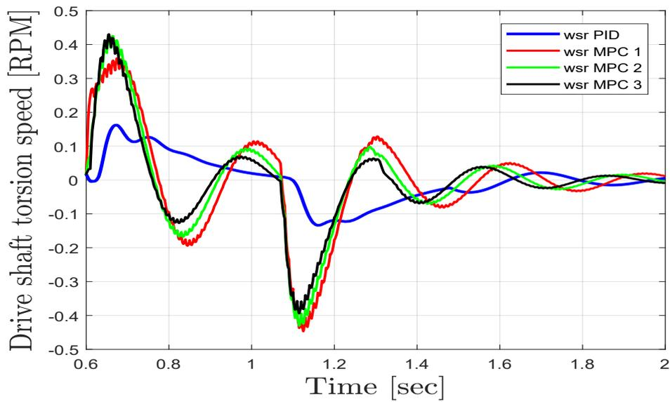
Figure 5.4: Drive shaft torsion speed simulation results.
