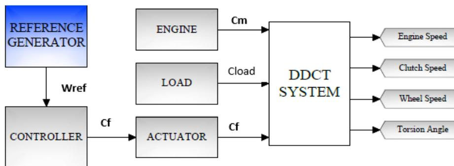
Figure 2.9: Block diagram of the DDCT system.
