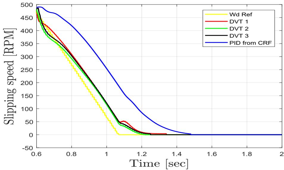
Figure 5.21: Slipping speed Triple output control.
