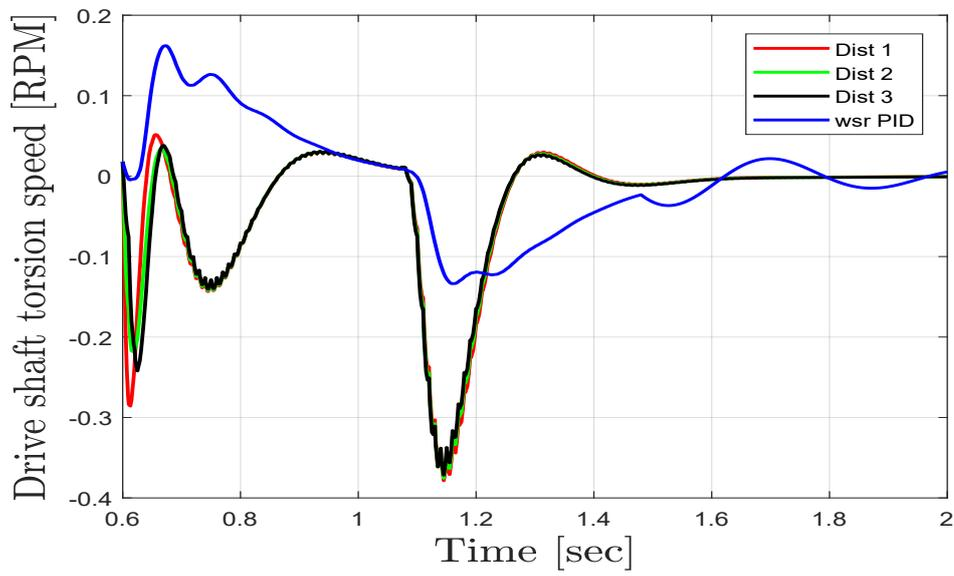
Figure 5.30: Drive shaft torsion speed with driver disturbance.
