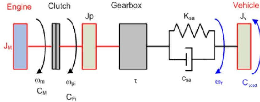
Figure 3.2: Linear driveline scheme.
