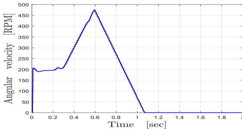
Figure 2.12: Reference signal for clutch slipping speed.
