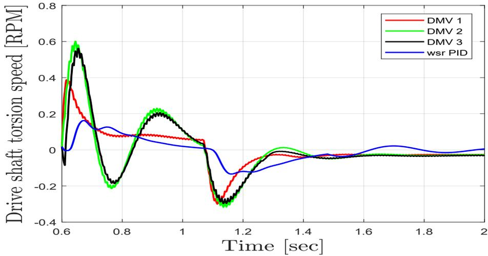
Figure 5.9: Drive shaft torsion speed Double Manipulated Variable.
