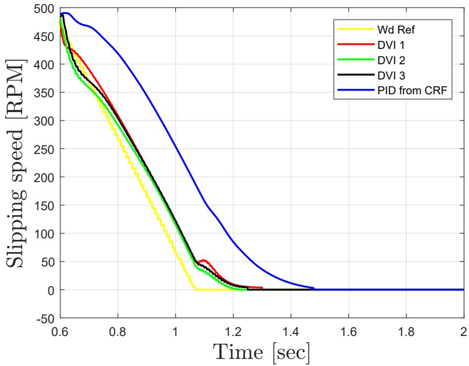
Figure 5.14: Slipping speed Double Manipulated Variable with Integrator.
