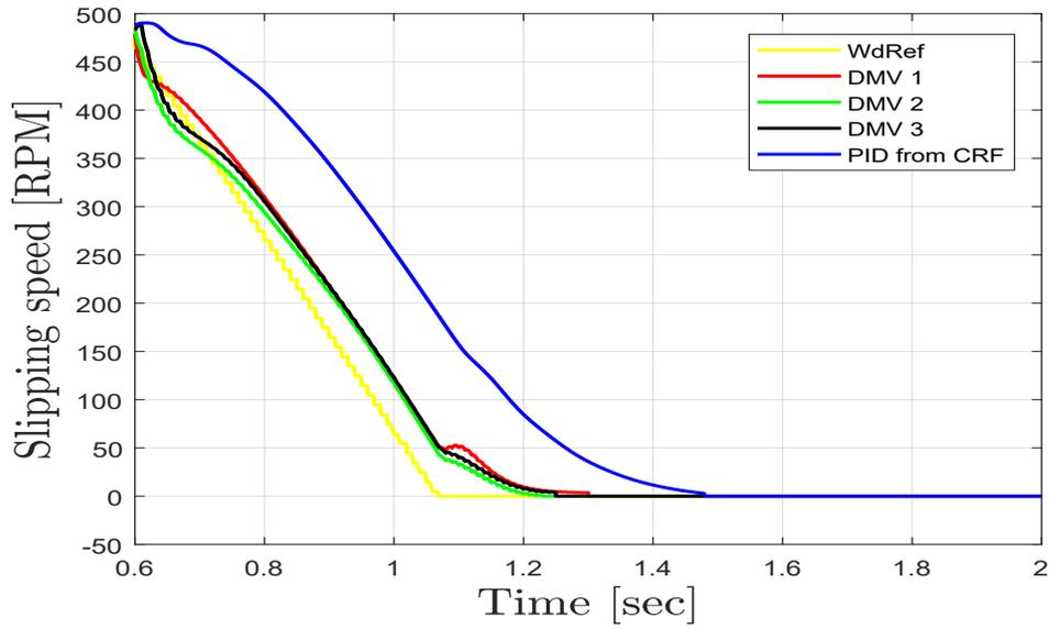
Figure 5.7: Slipping speed Double Manipulated Variable.
