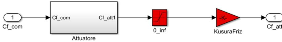
Figure 2.13: Inner part of the actuator.
