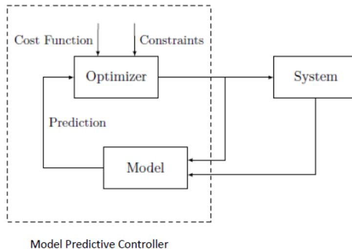
Figure 4.1: Block scheme of an MPC.
