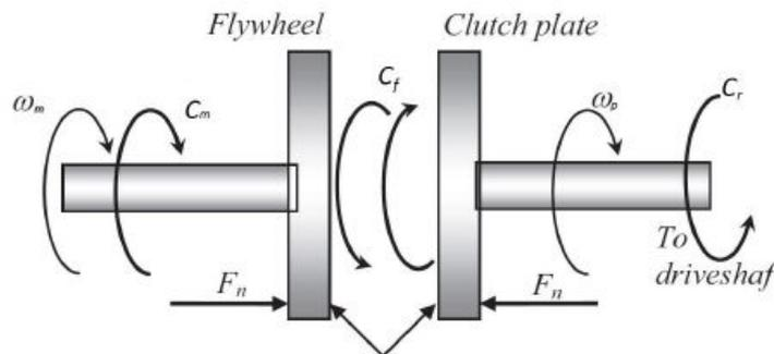
Figure 2.5: Schematic model of a dry-clutch.
