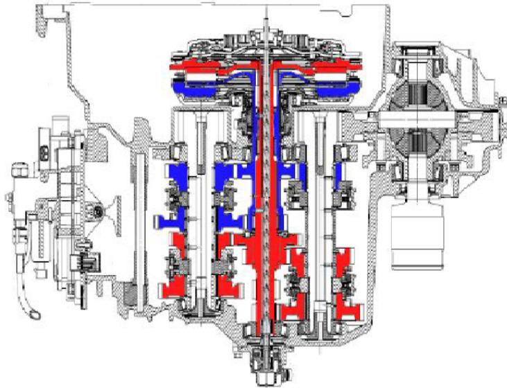
Figure 2.2: Cross section of the C635 DDCT.
