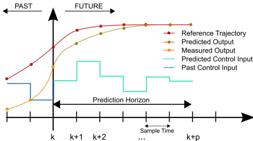
Figure 4.2: Receding Horizon principle.
