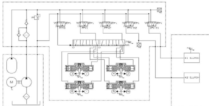
Figure 2.4: C635 DDCT complete actuation circuit.
