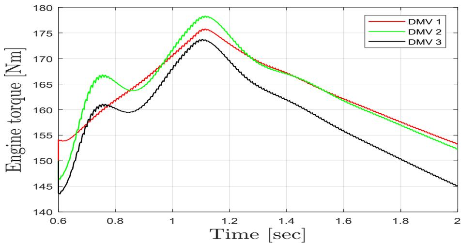
Figure 5.10: Engine torque Double Manipulated Variable.
