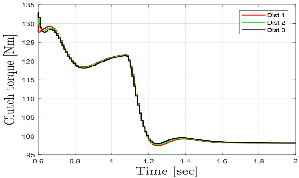
Figure 5.32: Clutch torque with driver disturbance.
