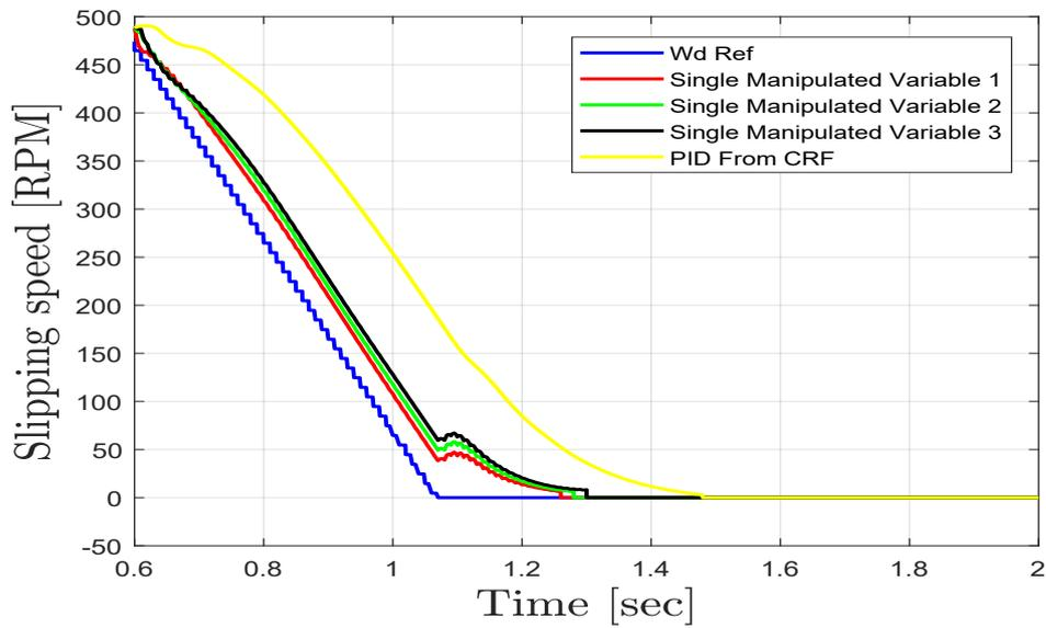
Figure 5.2: Slipping speed simulation results.
