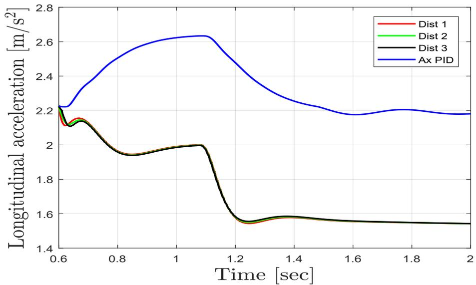
Figure 5.33: Longitudinal acceleration with driver disturbance.
