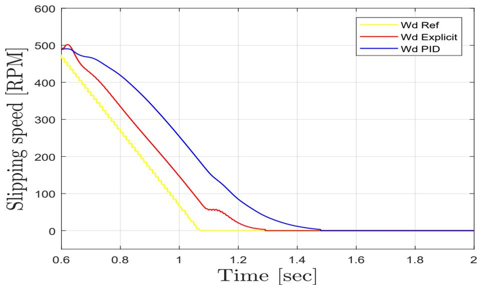
Figure 6.2: Slipping speed obtained with explicit MPC.
