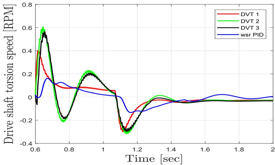
Figure 5.23: Drive shaft torsion speed Triple output control.
