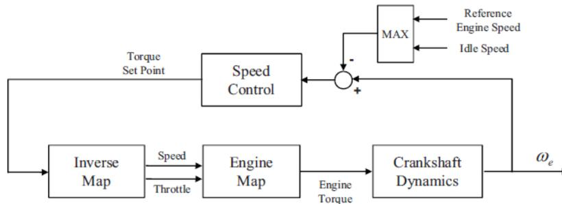
Figure 2.8: Block diagram of the engine speed/torque control analysed in [4].
