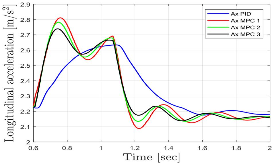
Figure 5.3: Longitudinal acceleration simulation results.
