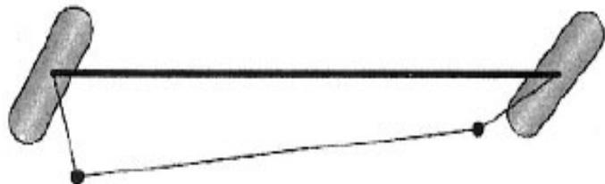
Figure 3.4: Differential steer from a trapezoidal tie-rod arrangement
