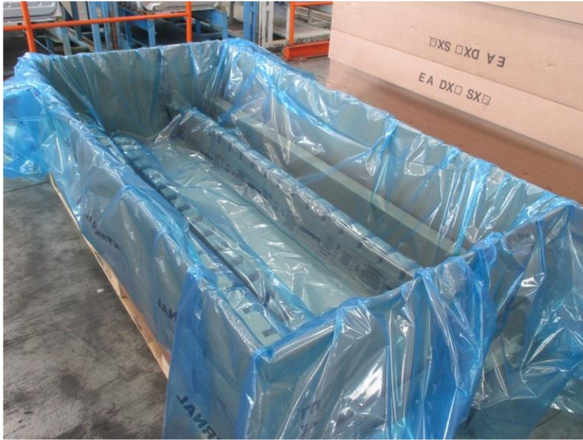
Figure 3.5 Laying of a VCI sheet into the box [FCA photo]
