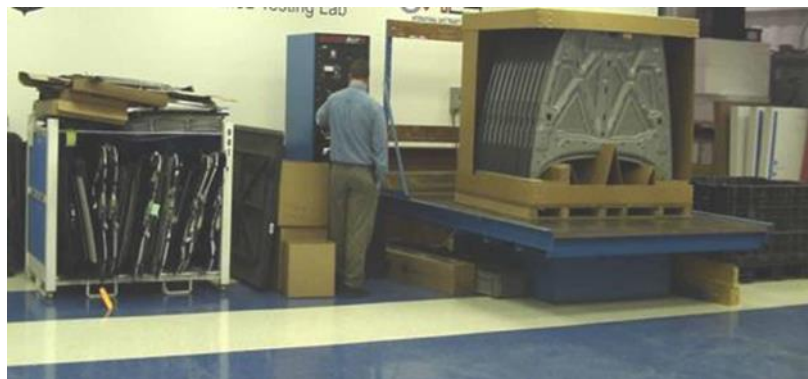
Figure 3.2 "Shake Table" test [FCA photo]
