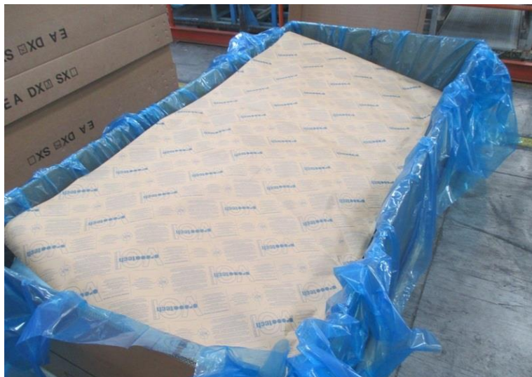
Figure 3.6 Laying of VCI sheet above the items [FCA photo]
