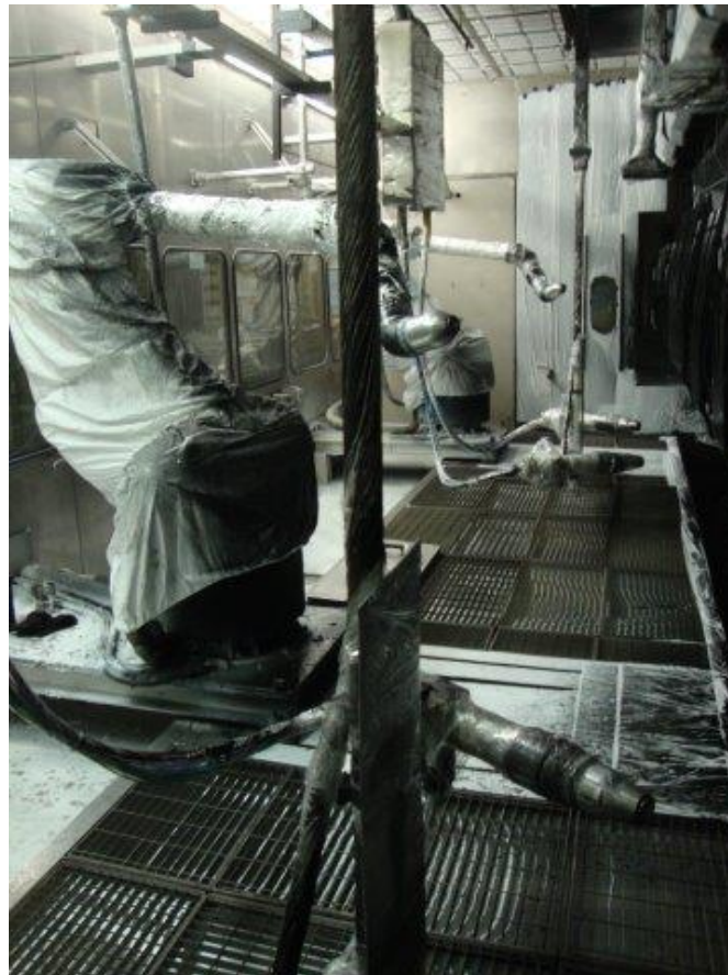
Figure 33. The robots work close to the racks due to the shiftable floor
