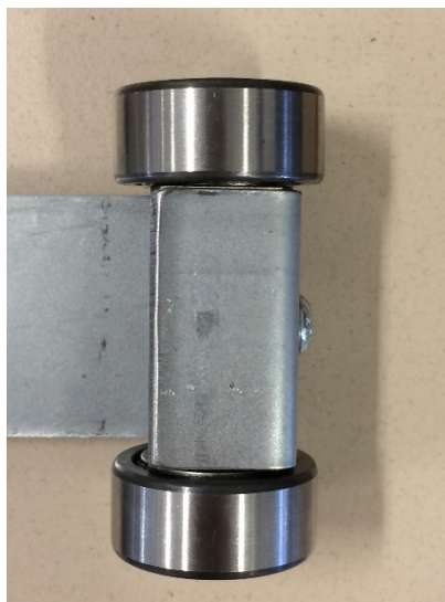
Figure 23. Detail of wheels running on the conveyor
