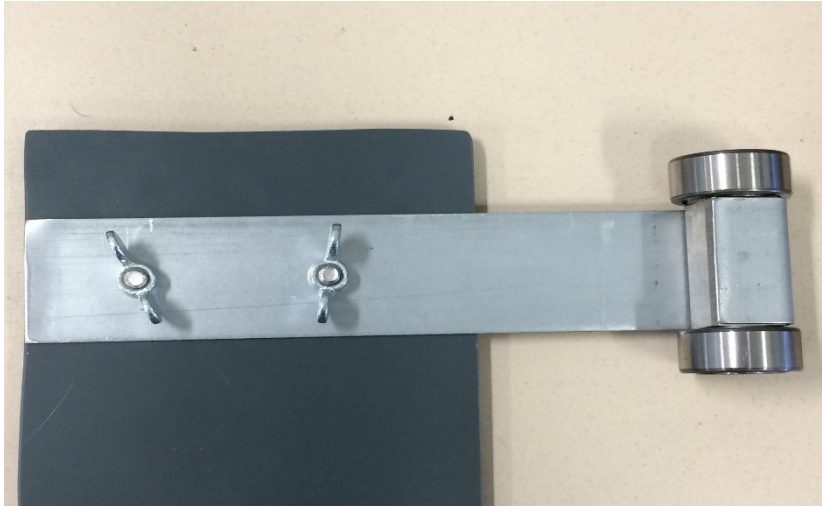
Figure 22. Tool realized using wheels, plugs and metal sheet
