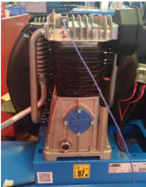
Figure 56- Experimental set up vibration test point 1
