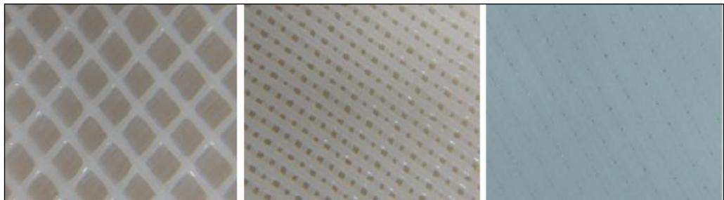
*Figure 3. Infill options, from the left: low, high and solid [9]*
