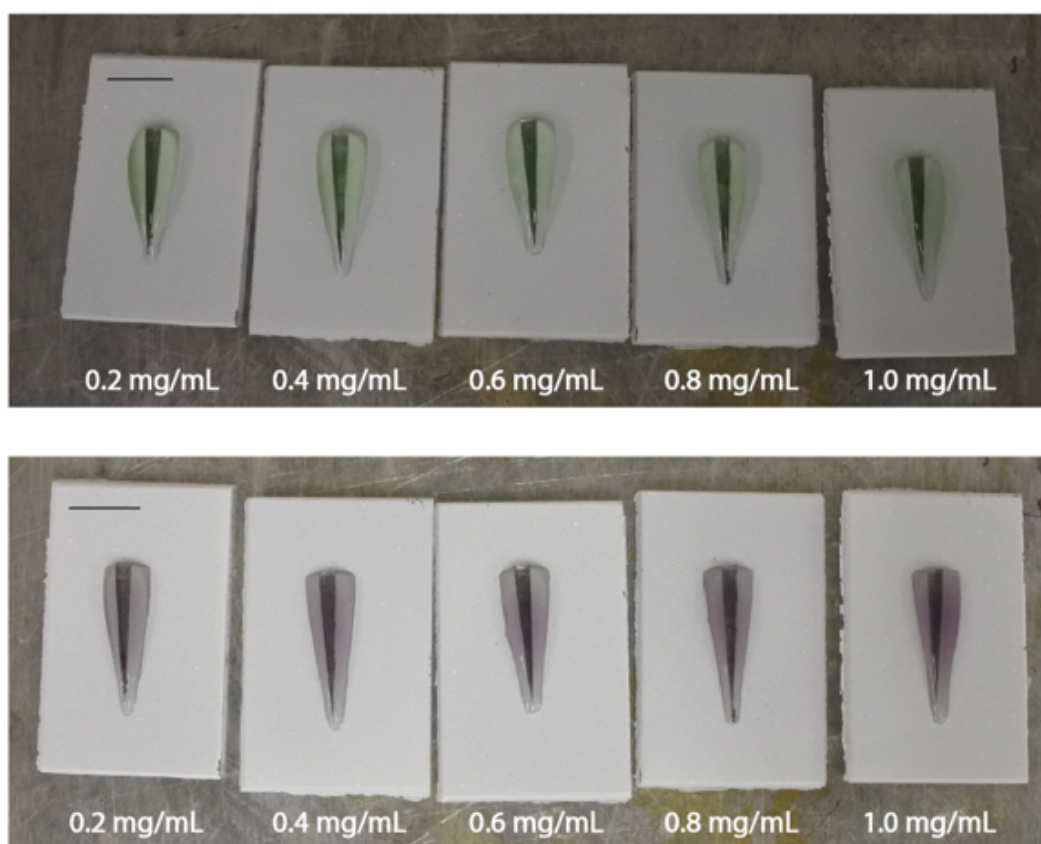
Figure 36: (a) 160\ \mu\text{L} of green BCA reagent is dispensed at the beginning of the track and transported to cover all the transport and detection region of each substrate. (b) The color of the reagent changes due to the presence of the proteins and its intensity is proportional to the concentration. Notice that as the concentration of added BSA bound to the axial track increases, so does to intensity of the purple color.
