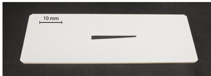
Figure 12: Wedge-shaped amine-functionalized track on a TiO_2 :PMC superhydrophobic background.
