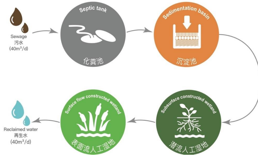
Figure 4.10 water purification system of honghu lantian ecological park (source: author)
