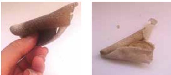
If the layer is very thin, the material loses water and it will be more fragile and will present ruptures.
