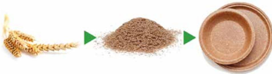
*“Our production process does not require significant amounts of water, or mineral resources, or chemical compounds. From 1 ton of pure, edible wheat bran we can produce up to 10,000 units of plates or bowls.*
