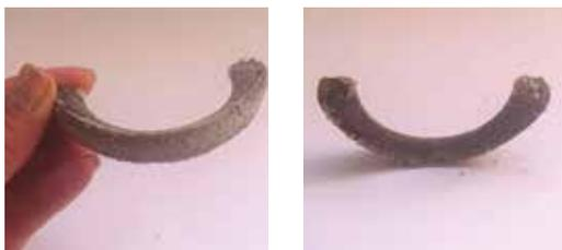
The material will not maintain the shape of the mold during the cooling process, it will contract unless it takes a specific shape when drying.
