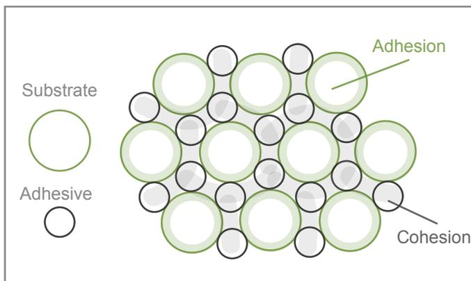
Figure 3 Substrate and husk rice particles Adhesion - Cohesion
