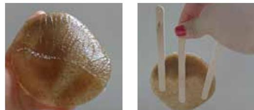
The content of glycerin in the Basic composition acts such as plastification allowing the solidification process, if you put more than that the material will be sticky and with an excess of liquids.
