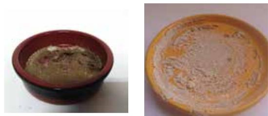
The material of the mold must allow to mix the substance on the right way and be uniformly heated, if the material is porous as the ceramic the substance may adhere to the bottom or become powder when drying.
