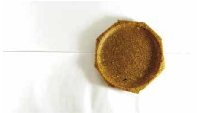
From the results obtained by *D. Perozzi* it is possible to analyze some behavior of the material similar to thermoplastic materials. For example, once formed and brought to room temperature it can be ground or pulverized and re-heated to be reformed.
