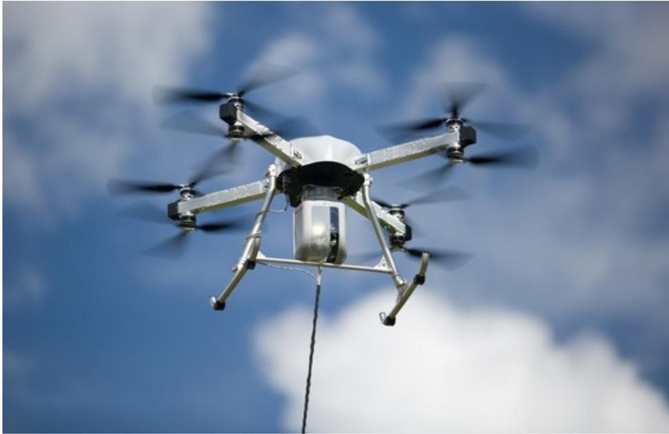
Figure 1.4: Watt 200 tethered drone
