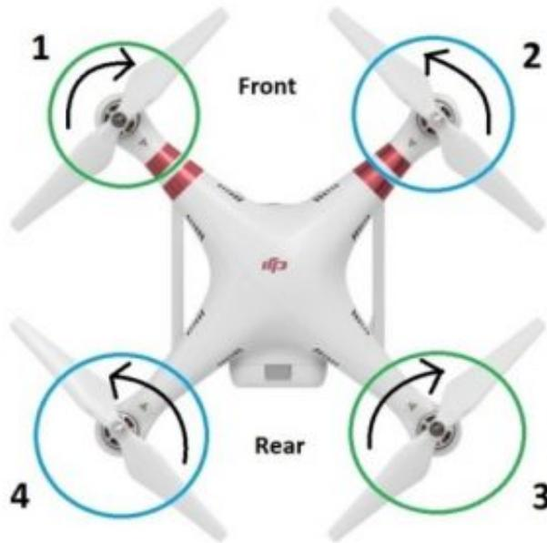
Figure 5.1: Angular speed convention
