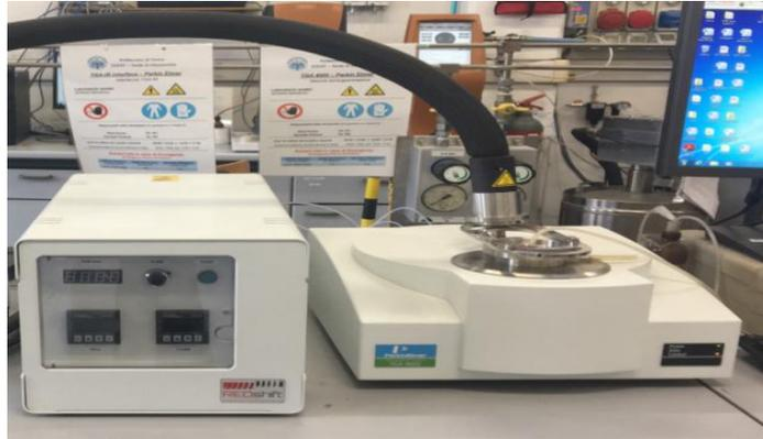
**Figure 1.21.** TGA 4000-Perkin Elmer
