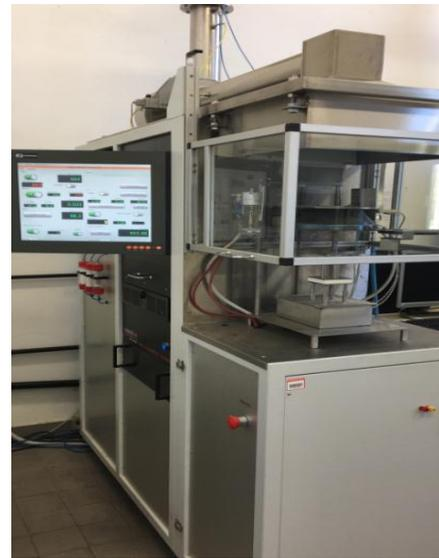
**Figure 1.24.** Laboratory cone calorimeter
