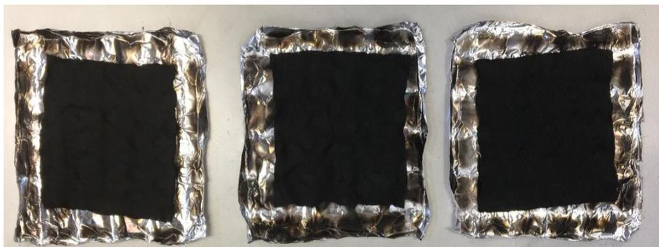
**Figure 3.12.** Residue of COT+SOL (70/30) after cone calorimetry test
