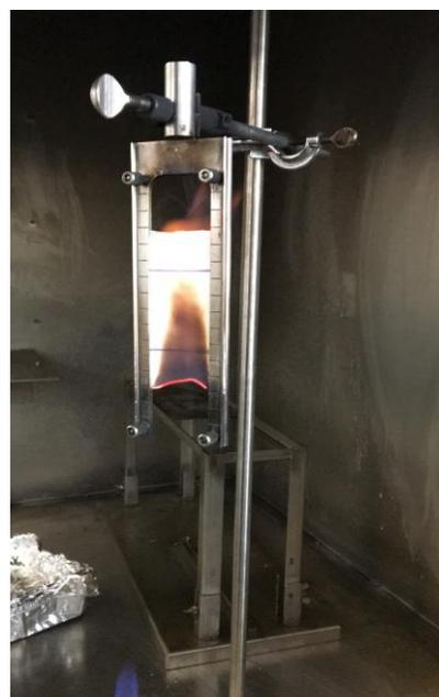
**Figure 2.5.** UL94 burning test (in horizontal configuration)
