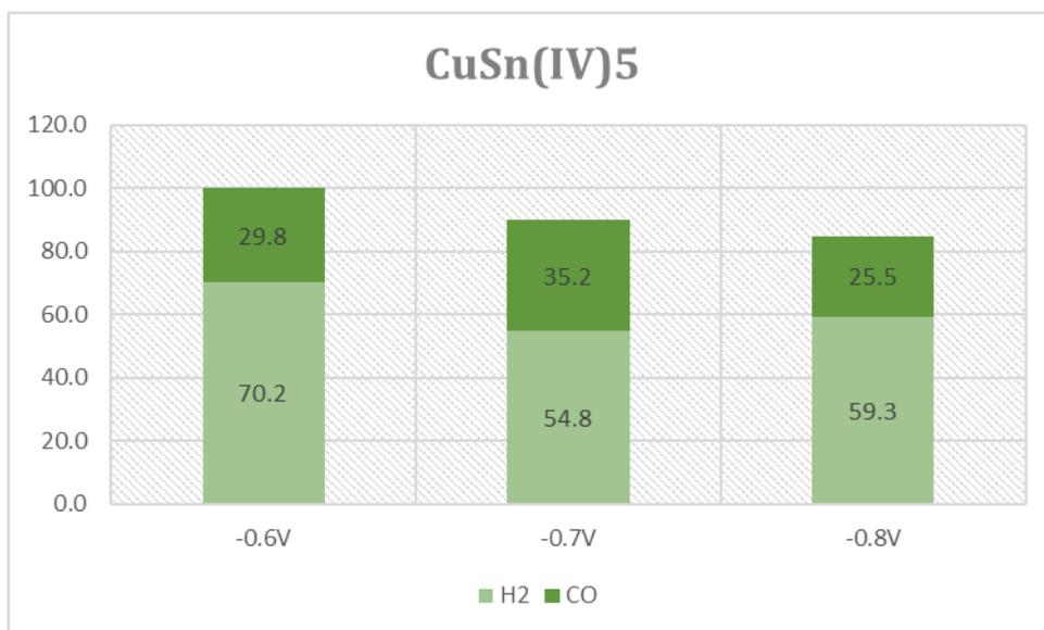
**Fig.3.32** Faradaic efficiencies of CuSn(IV)5 for hydrogen and carbon monoxide at the three different potentials.
