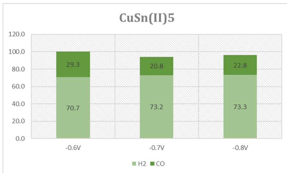
**Fig.3.25** Faradaic efficiencies of CuSn(II)<sub>5</sub> for hydrogen and carbon monoxide at the three different potentials.
