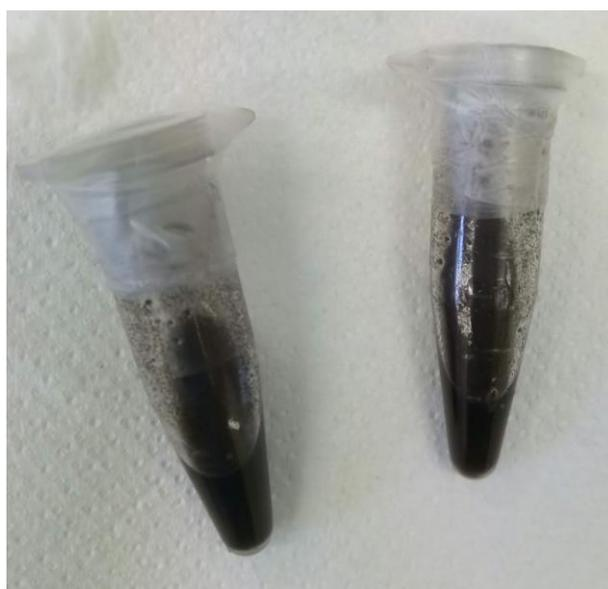
**Fig.2.7** Ink containing the catalyst powder, isopropanol and Nafion®.
