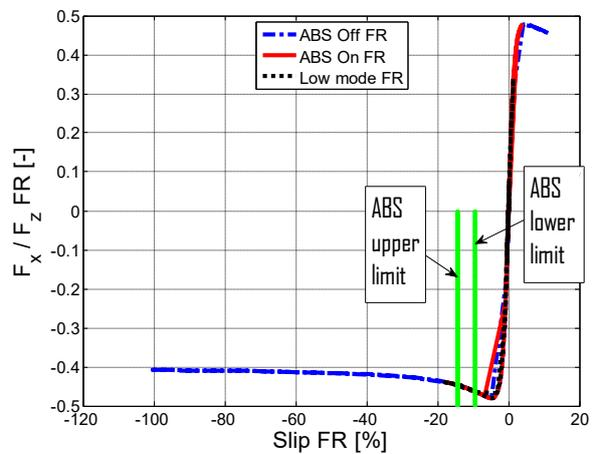
Figure 2.72 –  $F_x / F_z$  vs slip, front right.
