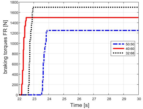
Figure 3.4.42 – Braking torques, front.
