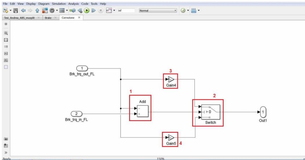
Figure 3.4.26 – Correction introduced in Simulink model.
