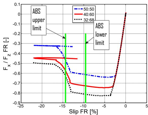
Figure 2.107 –  $F_x / F_z$  vs slip, front.
