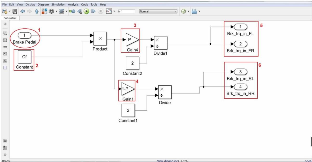
Figure 3.33 – Braking distribution subsystem.
