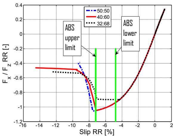
Figure 2.106 –  $F_x / F_z$  vs slip, rear.
