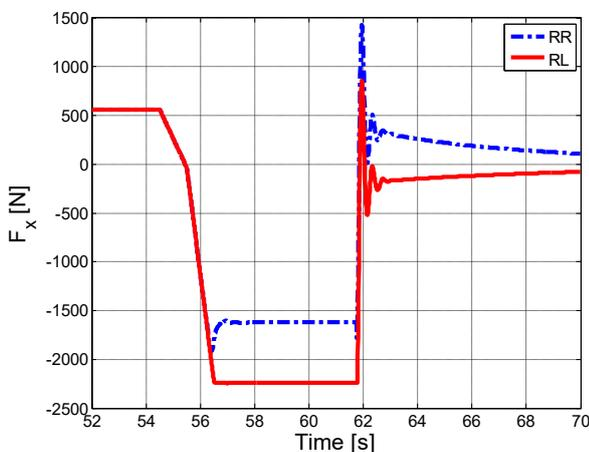
Figure 1.62 – Longitudinal rear forces.
