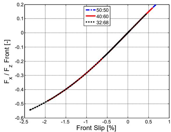
Figure 1.59 – Longitudinal force vs slip, front.
