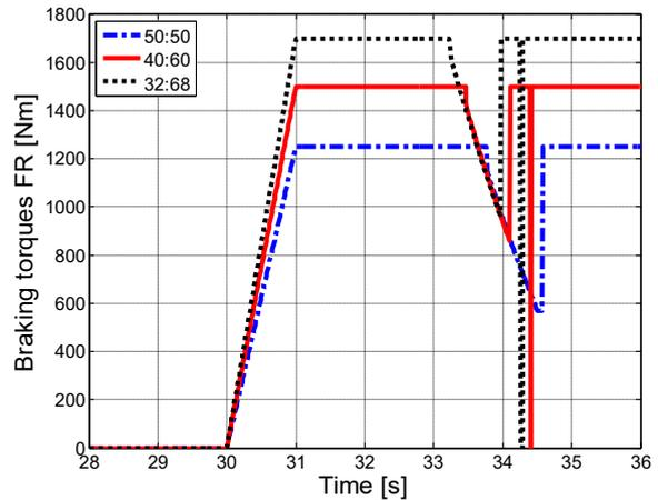
Figure 2.101 – Braking torques, front .
