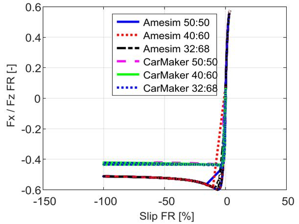
Figure 3.4.50 –  $F_x/F_z$  vs slip, front.
