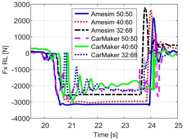
Figure 3.4.31 – Longitudinal forces, rear.
