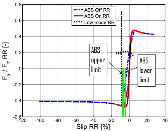
Figure 2.52 –  $F_x / F_z$  vs slip, rear right.
