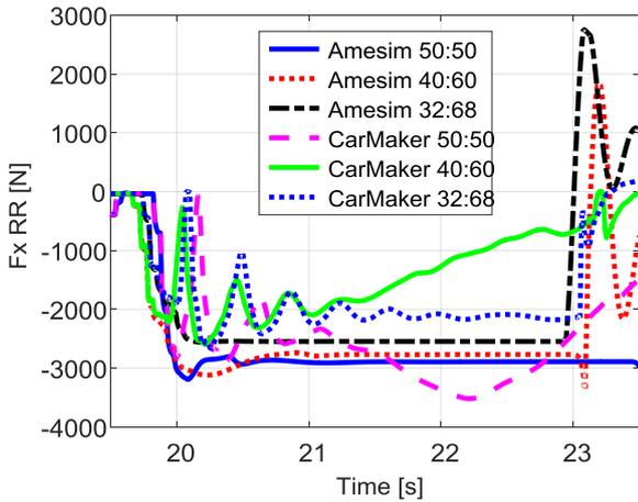
Figure 3.4.5 – Longitudinal forces, rear.
