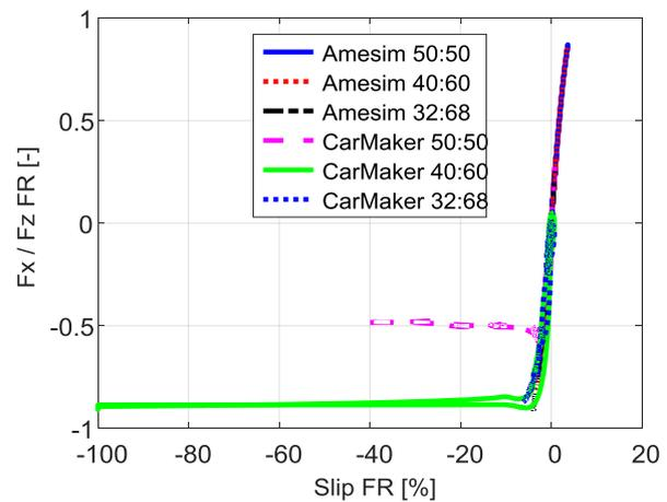
Figure 3.4.12 – Fx/Fz vs slip, front.
