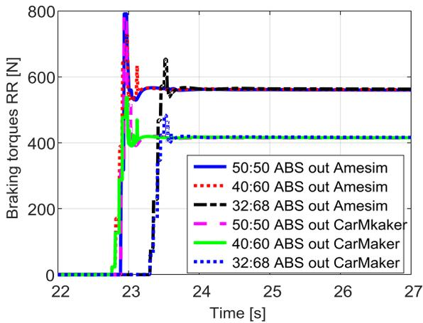
Figure 3.4.64 – Braking torques, rear.
