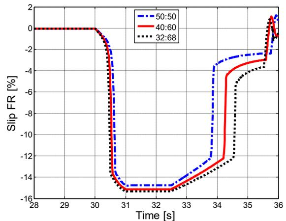
Figure 2.118 – Longitudinal slips, front.
