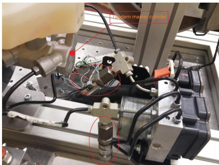
Figure 4.5 – TMC pressure sensors
