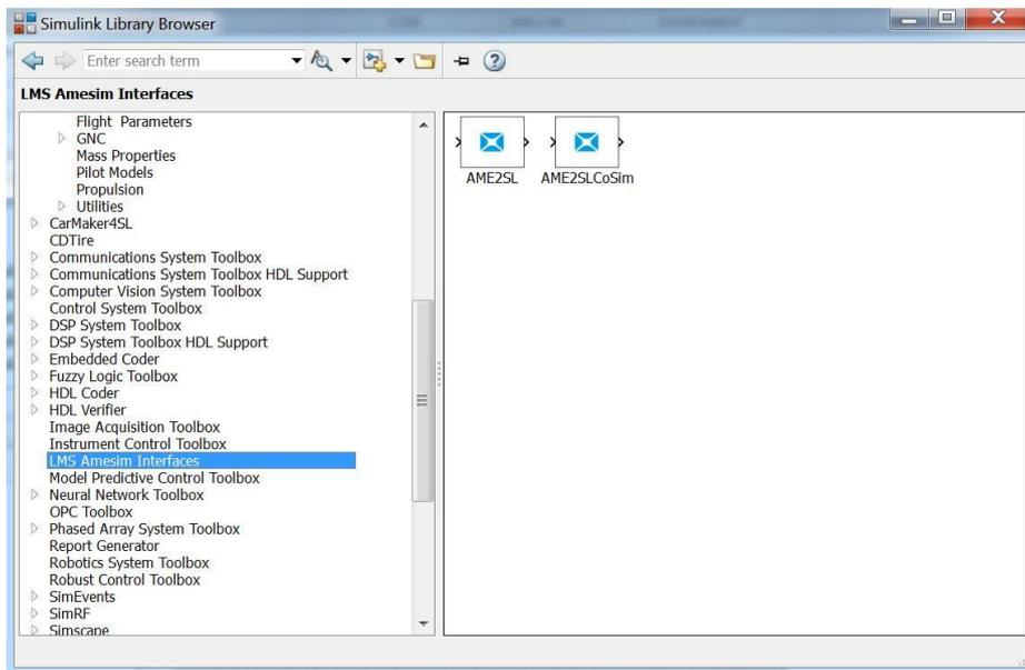
Figure 3.22 – Simulink library with Amesim blocks.
