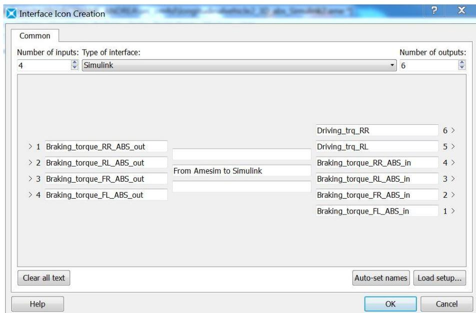
Figure 3.26 – Creation of interface block Amesim/Simulink.
