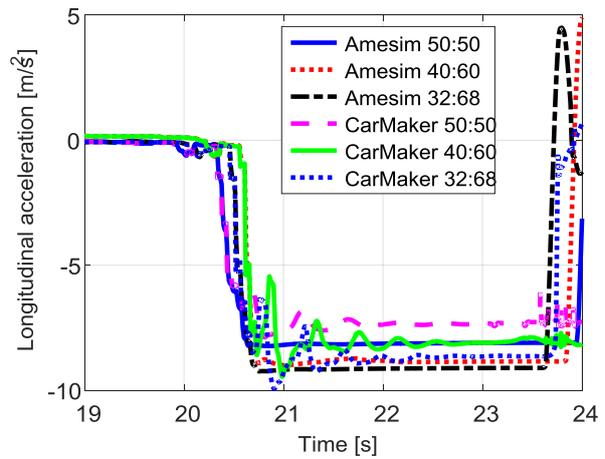
Figure 3.4.28 – Longitudinal acceleration.
