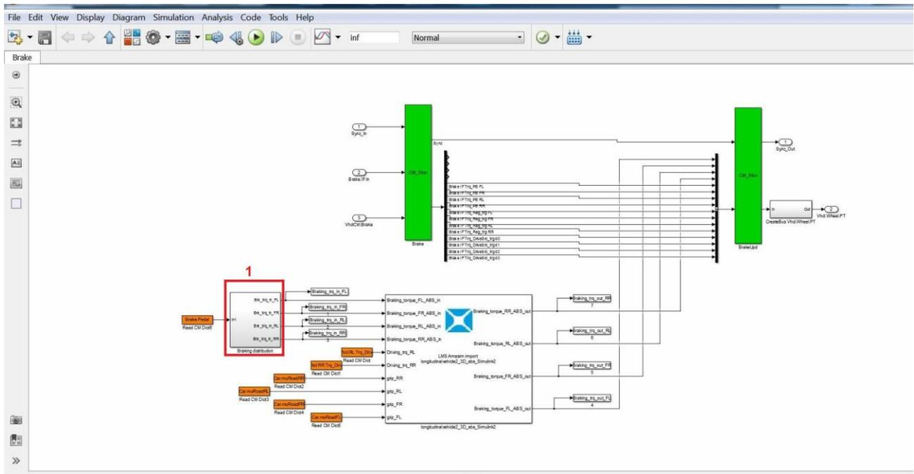
Figure 3.32 – Amesim model inserted in the Simulink model of CarMaker.
