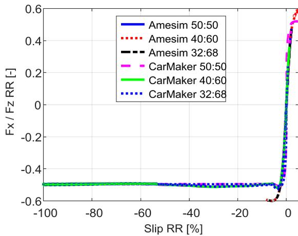
Figure 3.4.70 – Fx/Fz vs slip, rear.
