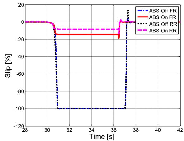
Figure 2.27 – Longitudinal slips.
