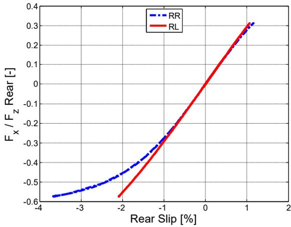
Figure 1.74 – Longitudinal forces vs slip, rear.
