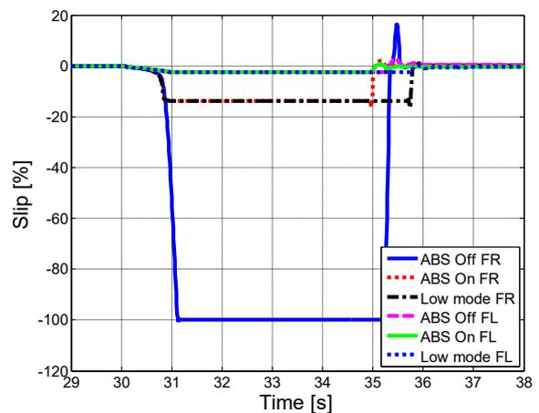
Figure 2.49 – Longitudinal slips, front.
