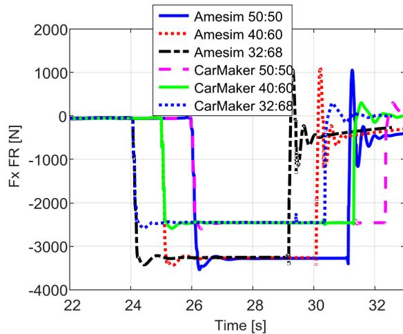
Figure 3.4.56 – Longitudinal forces, front.
