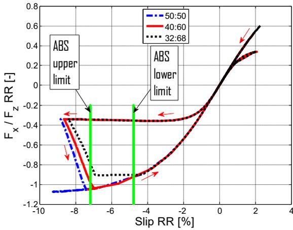
Figure 2.119 –  $F_x / F_z$  vs slip, rear.
