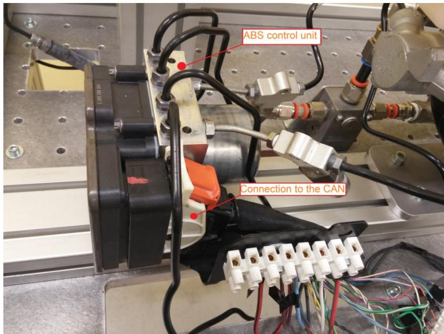
Figure 4.7 – ABS and CAN connection
