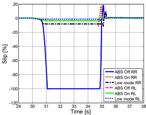
Figure 2.86 – Longitudinal slips, rear.
