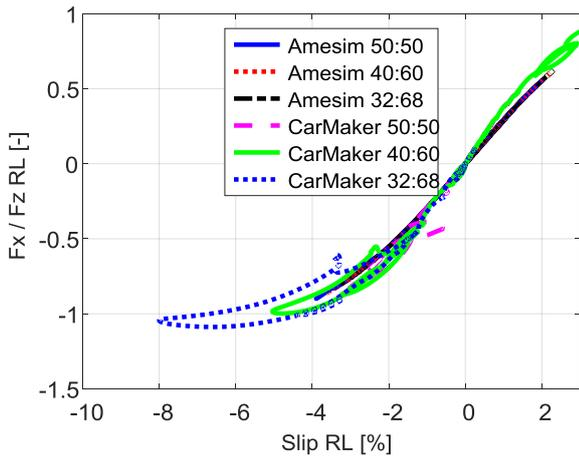
Figure 3.4.94 –  $F_x/F_z$  vs slip, RL.
