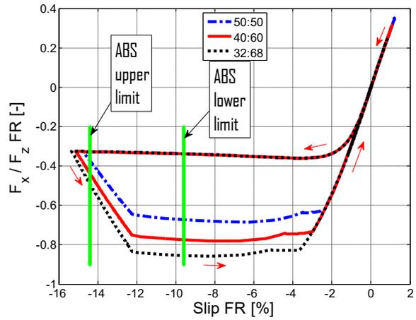
Figure 2.120 –  $F_x / F_z$  vs slip, front.
