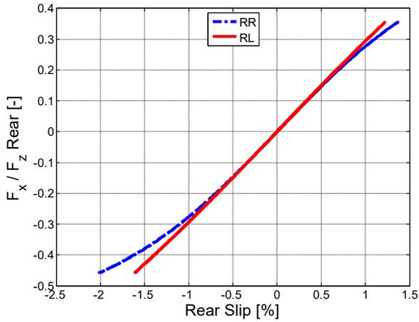
Figure 1.82 – Longitudinal forces vs slip, rear.
