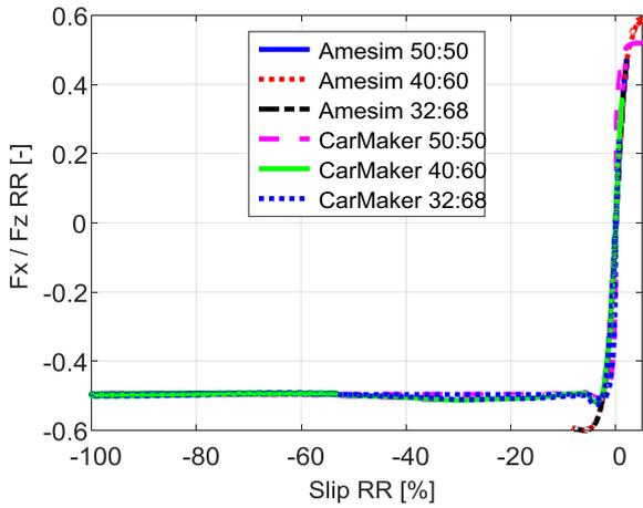
Figure 3.4.60 – Fx/Fz vs slip, rear.
