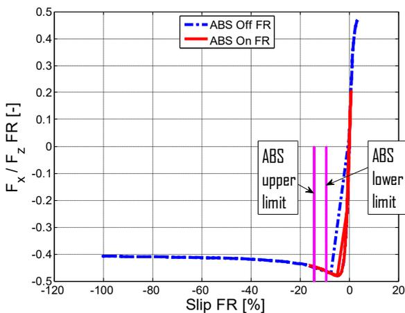
Figure 2.19 –  $F_x / F_z$  vs slip, front.
