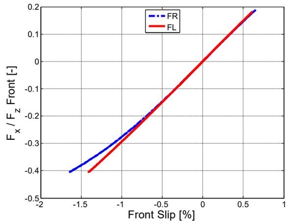
Figure 1.67 – Longitudinal forces vs slip, front.
