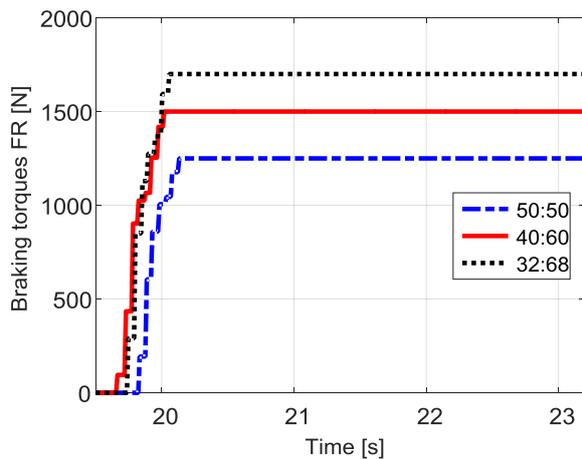
Figure 3.4.4 – Braking torques, front.
