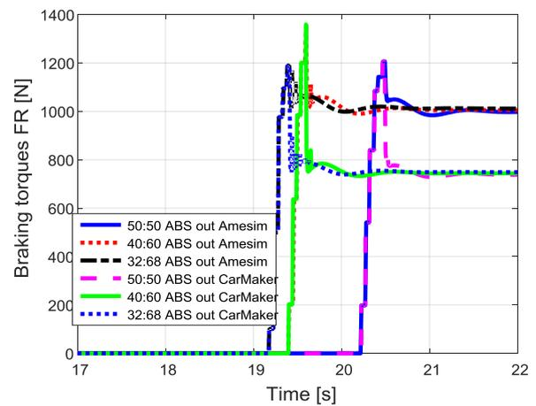
Figure 3.4.85 – Braking torques, FR.
