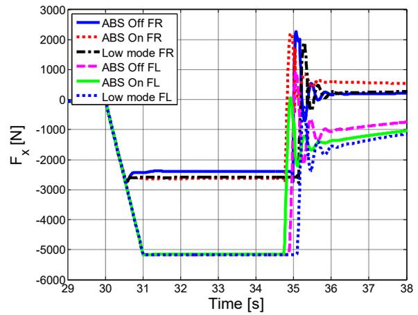
Figure 2.85 – Longitudinal forces, front.
