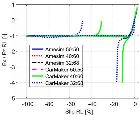
Figure 3.4.37 – Fx/Fz vs slip, rear.
