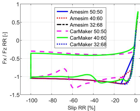
Figure 3.4.11 – Fx/Fz vs slip, rear.
