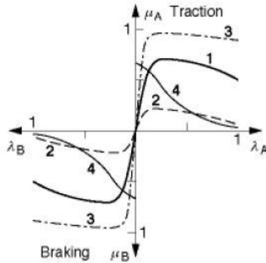
Figure 2.1 – Adherence / slip curves.
