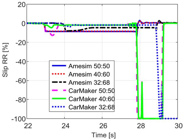
Figure 3.4.68 – Longitudinal slips, rear.
