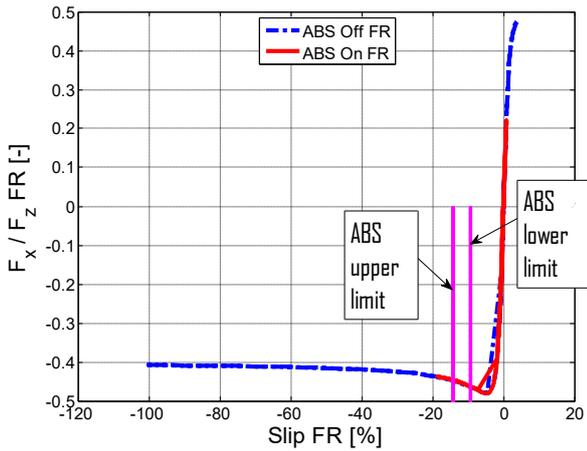
Figure 2.28 –  $F_x / F_z$  vs slip, front.
