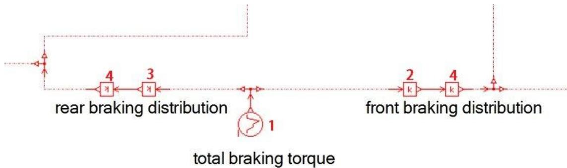
Figure 1.13 – Braking torque block.
