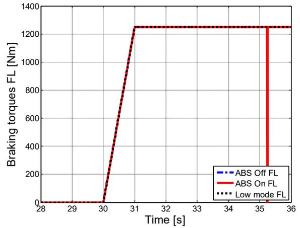
Figure 2.43 – Braking torques, front left.
