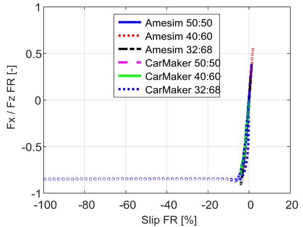
Figure 3.4.24 –  $F_x/F_z$  vs slip, front.
