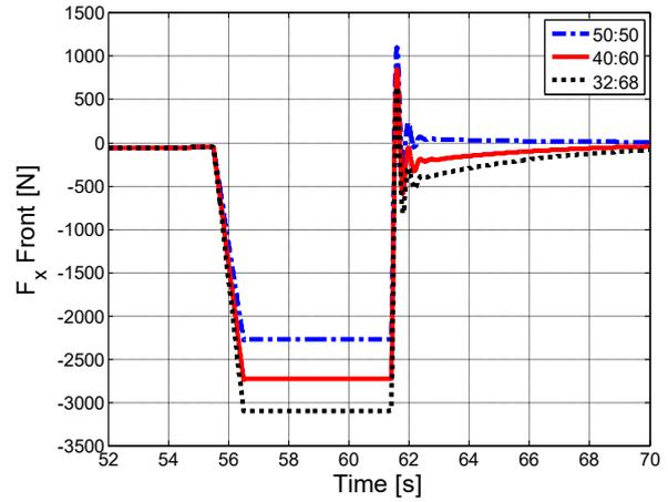
Figure 1.20 – Longitudinal forces, front.
