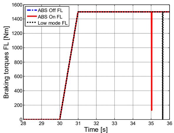
Figure 2.62 – Braking torques, front left.
