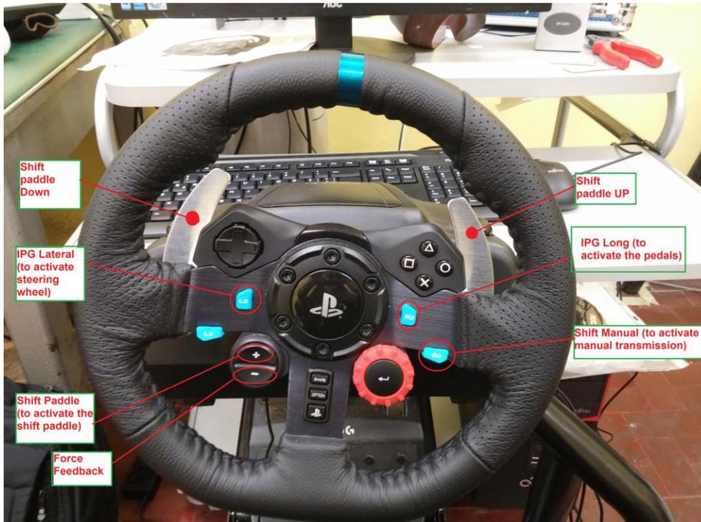
Figure 3.6 – Steering wheel: function of the buttons.
