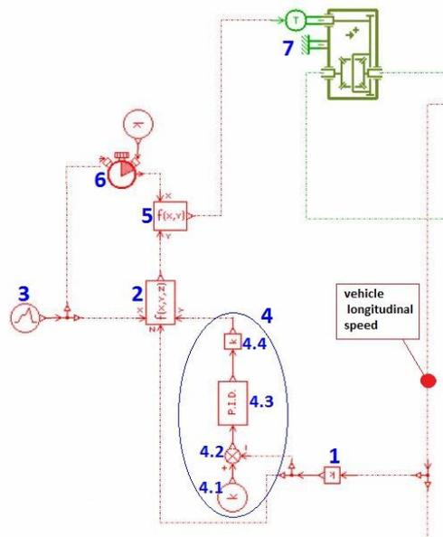
Figure 2.8 – Vehicle speed control.
