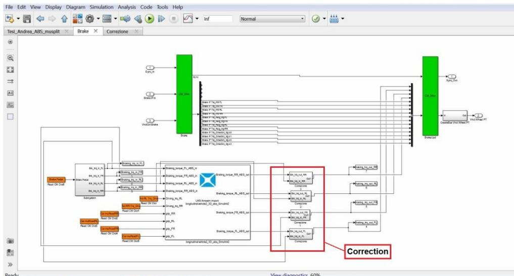
Figure 3.4.25 – Correction introduced in Simulink model.
