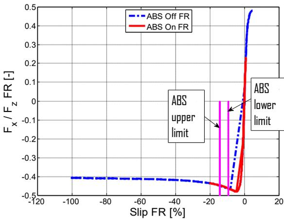
Figure 2.37 –  $F_x / F_z$  vs slip, front.
