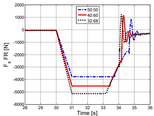
Figure 2.103 – Longitudinal forces, front.
