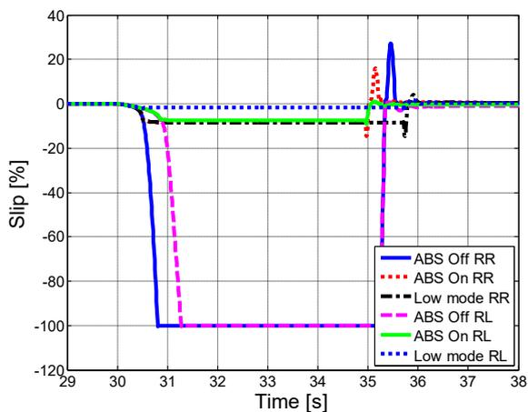
Figure 2.48 – Longitudinal slips, rear.
