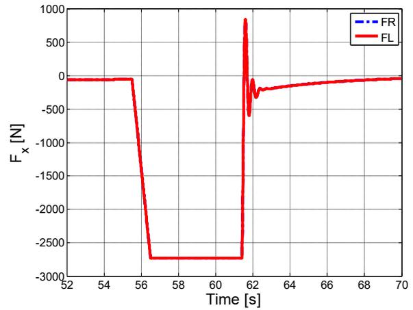
Figure 1.71 – Longitudinal front forces.
