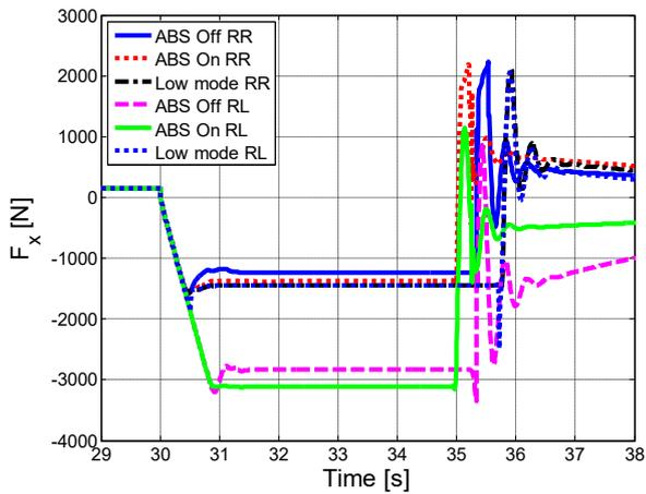
Figure 2.46 – Longitudinal forces, rear.
