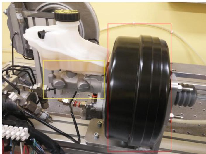
Figure 4.4 – Brake booster (red) and tandem master cylinder (yellow).
