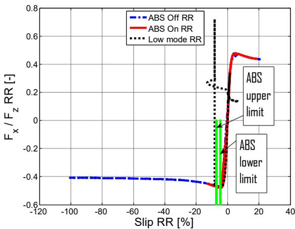
Figure 2.71 –  $F_x / F_z$  vs slip, rear right.
