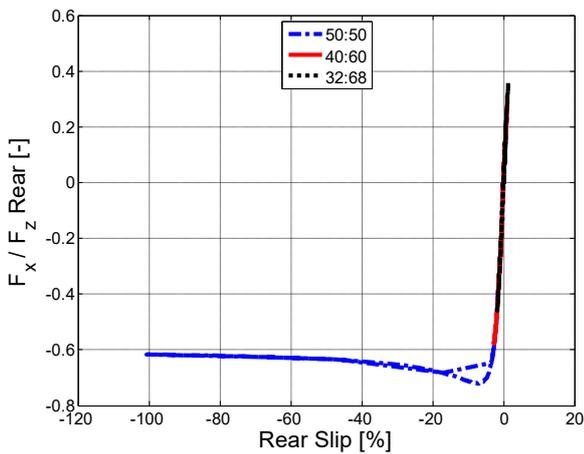
Figure 1.58 – Longitudinal force vs slip, rear.
