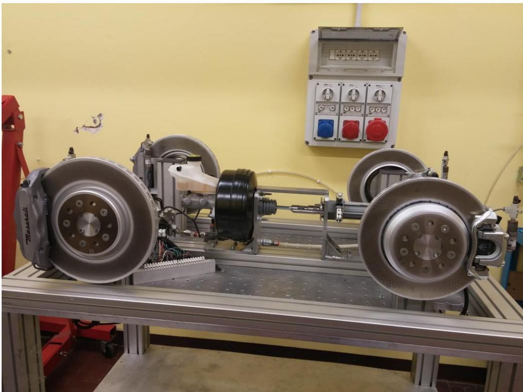
Figure 4.2 – Brake test rig.
