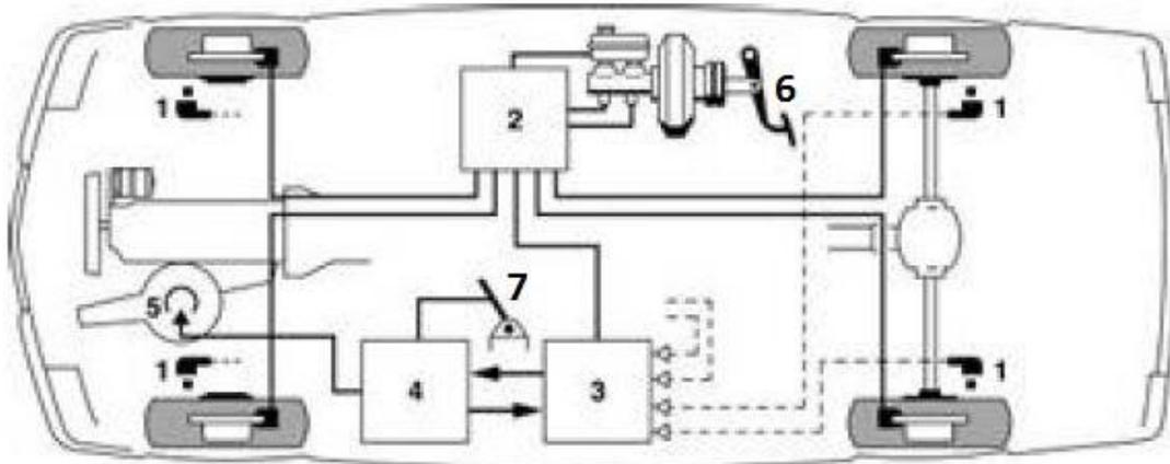
Figure 2.4 – ABS / TCS system components for car.
