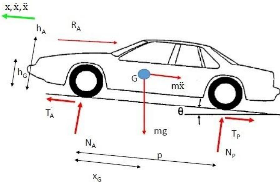
Figure 1.1 – Forces acting on the vehicle.
