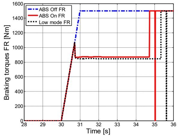
Figure 2.64 – Braking torques, front right.
