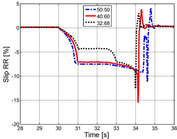
Figure 2.104 – Longitudinal slips, rear.
