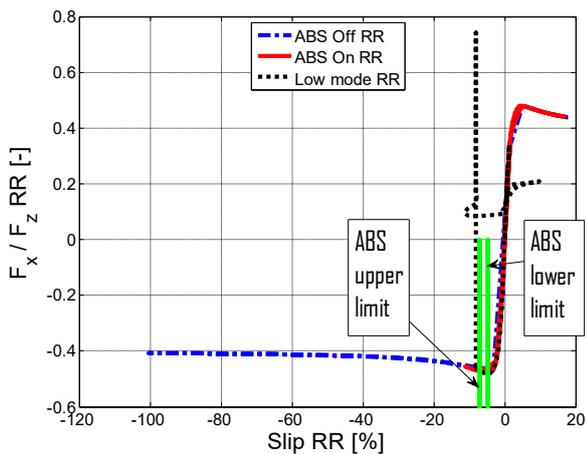
Figure 2.90 –  $F_x / F_z$  vs slip, rear right.
