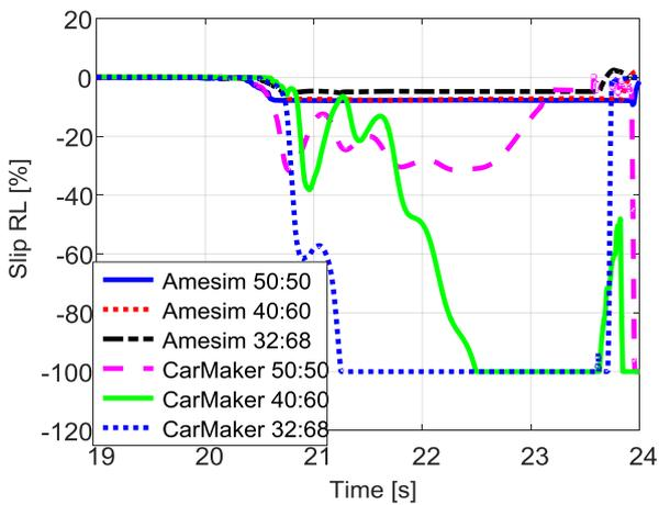
Figure 3.4.33 – Longitudinal slips, rear.
