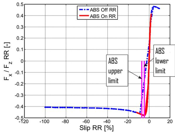
Figure 2.38 –  $F_x / F_z$  vs slip, rear.
