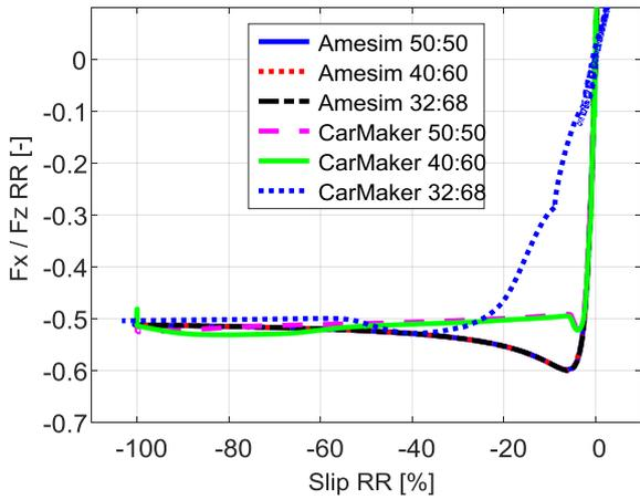
Figure 3.4.49 –  $F_x/F_z$  vs slip, rear.
