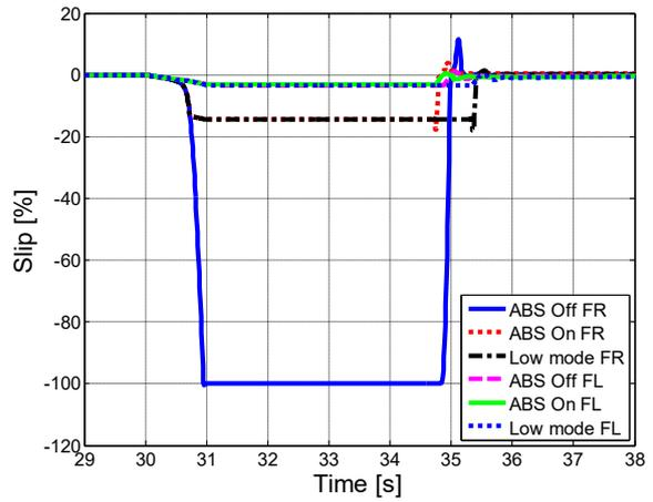
Figure 2.68 – Longitudinal slips, front.
