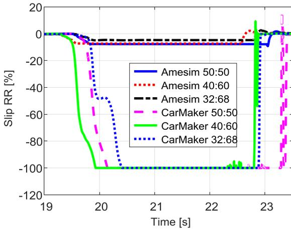
Figure 3.4.19 – Longitudinal slips, rear.
