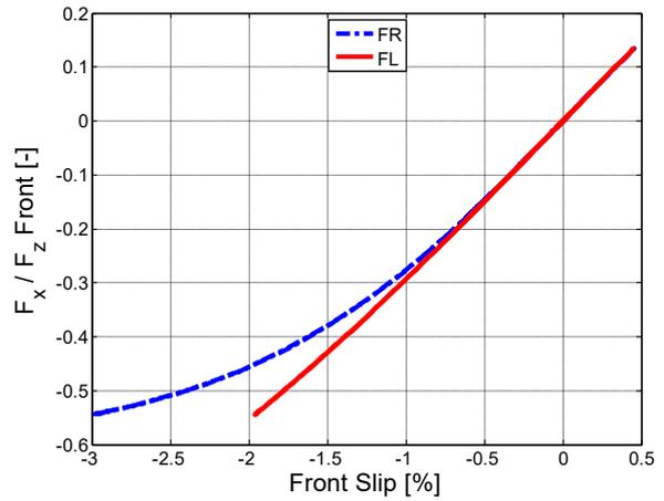
Figure 1.83 – Longitudinal forces vs slip, front.
