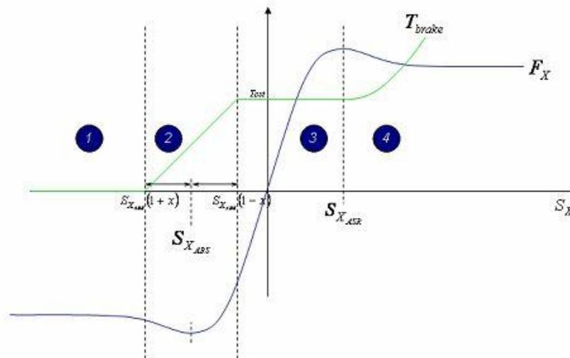
Figure 2.7 – How to ABS and ASR work.
