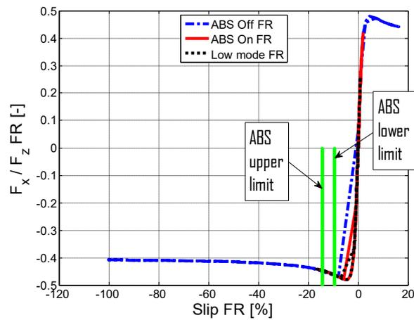
Figure 2.53 –  $F_x / F_z$  vs slip, front right.
