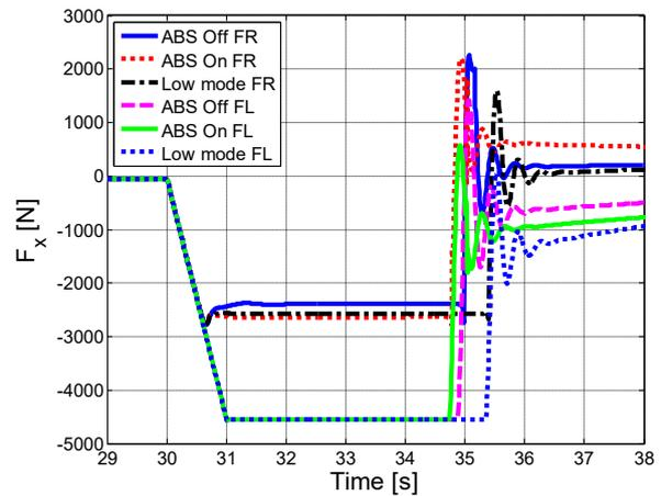
Figure 2.66 – Longitudinal forces, front.
