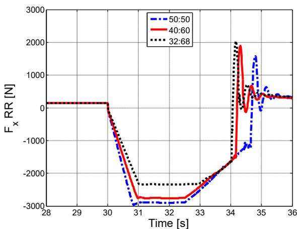
Figure 2.102 – Longitudinal forces, rear.
