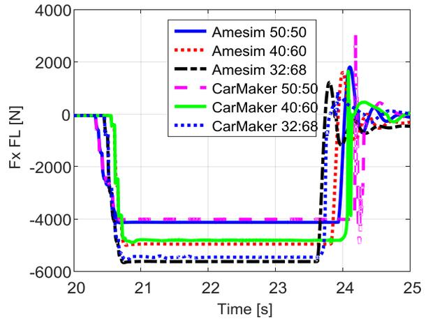
Figure 3.4.32 – Longitudinal forces, front.
