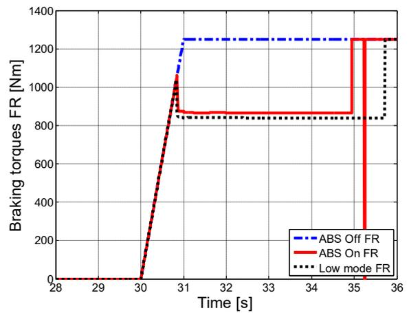
Figure 2.45 – Braking torques, front right.
