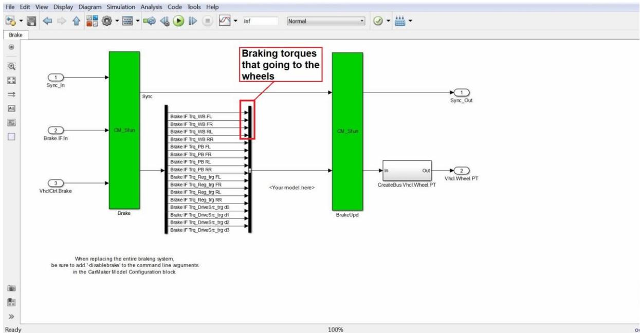
Figure 3.31 – Brake subsystem content.
