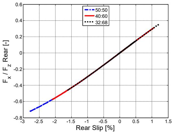
Figure 1.25 – Longitudinal force vs slip, rear
