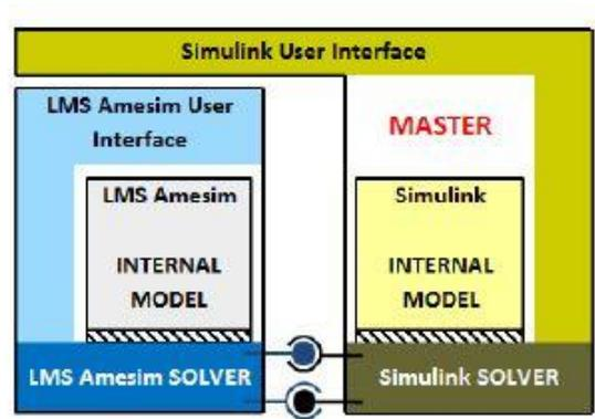
Figure 3.24 – Operation block AME2SLCosim.
