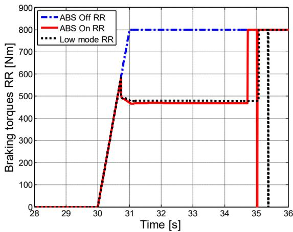
Figure 2.82 – Braking torques, rear right.
