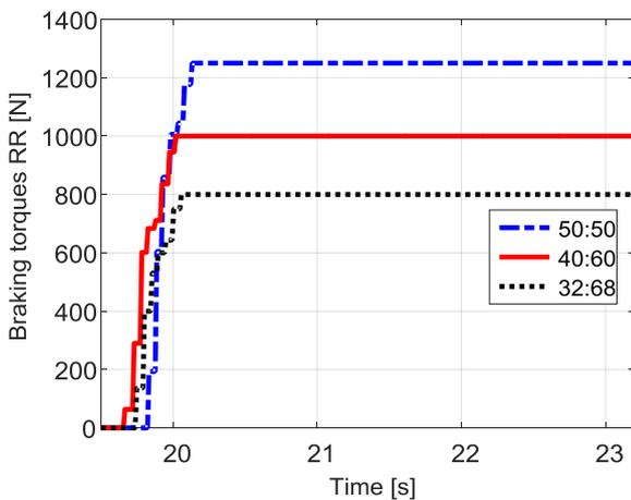
Figure 3.4.3 – Braking torques, rear.
