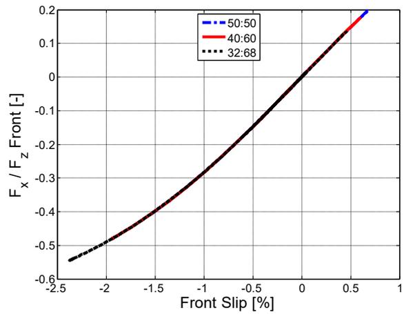
Figure 1.36 – Longitudinal force vs slip, front.
