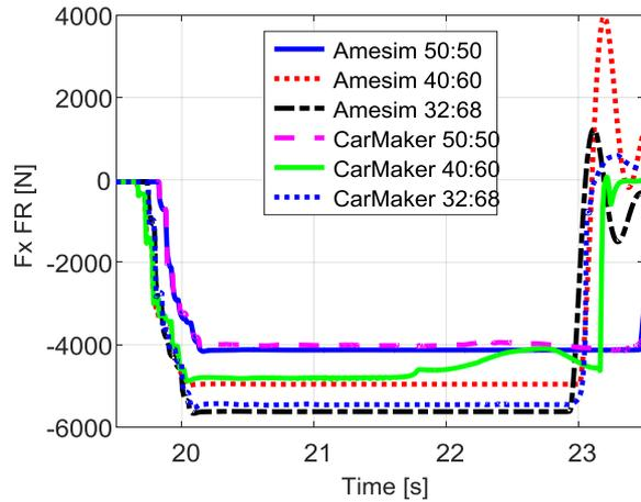
Figure 3.4.6 – Longitudinal forces, front.
