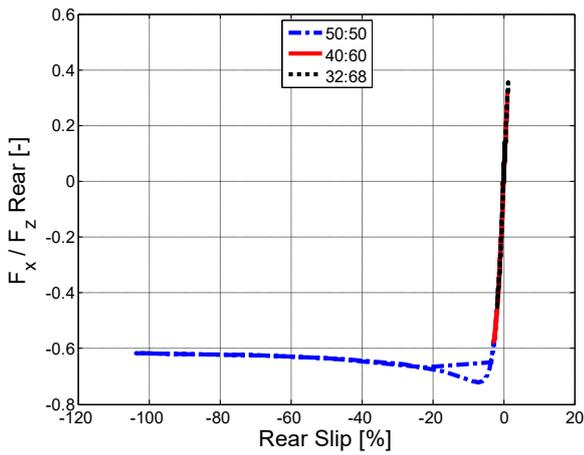
Figure 1.35 – Longitudinal force vs slip, rear.
