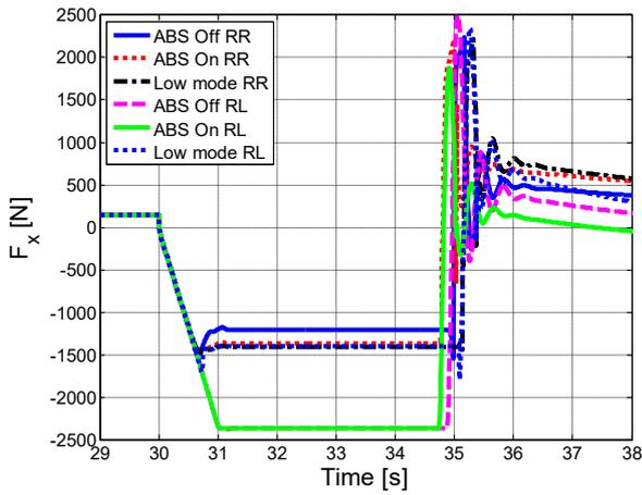
Figure 2.84 – Longitudinal forces, rear.
