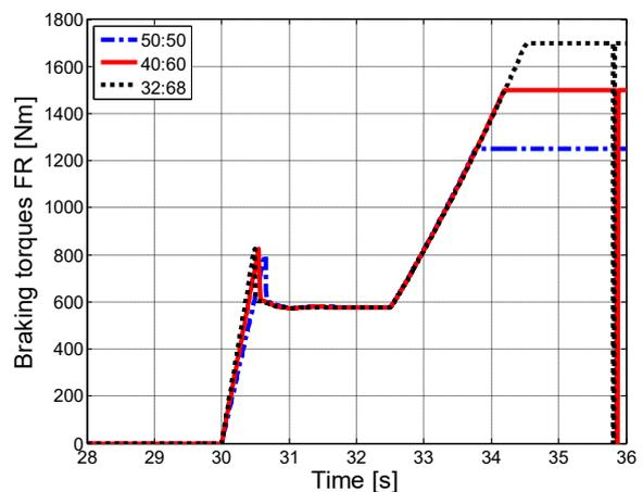
Figure 2.114 – Braking torques, front.
