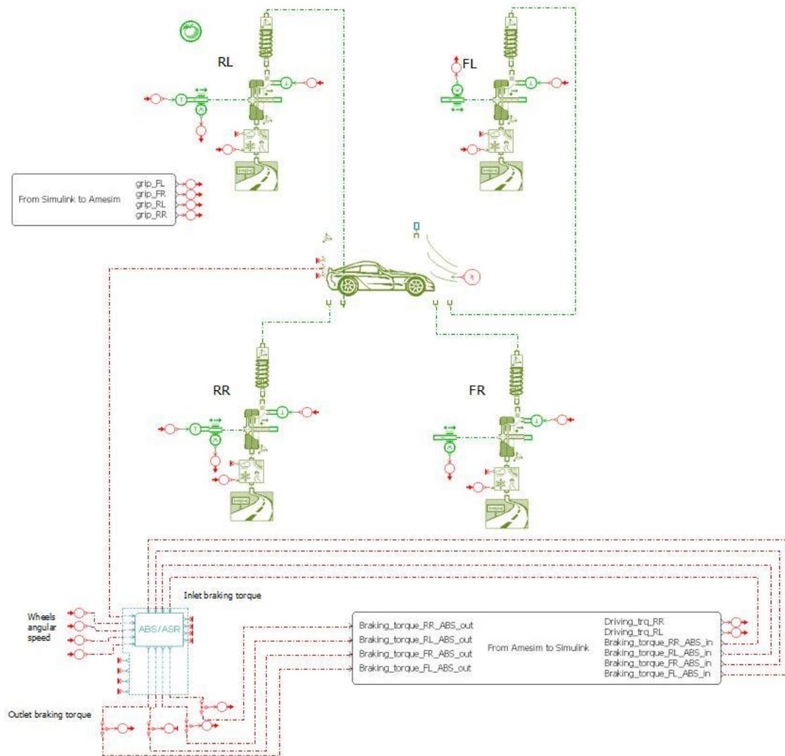
Figure 3.28 – Amesim complete model.
