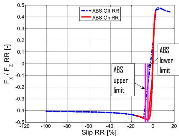
Figure 2.20 –  $F_x / F_z$  vs slip, rear.
