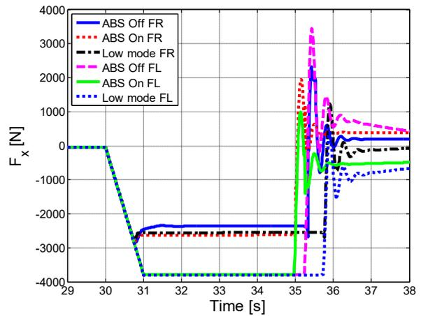
Figure 2.47 – Longitudinal forces, front.
