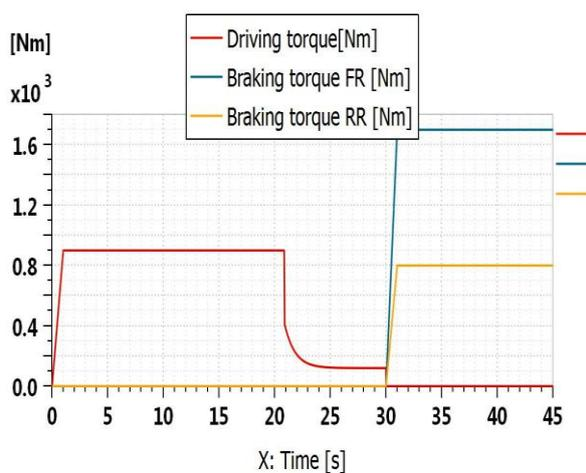
Figure 2.9 – Driving and braking torque.
