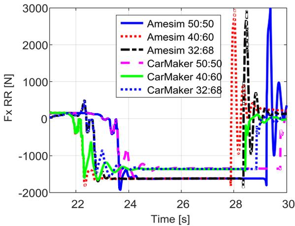
Figure 3.4.43 – Longitudinal forces, rear.
