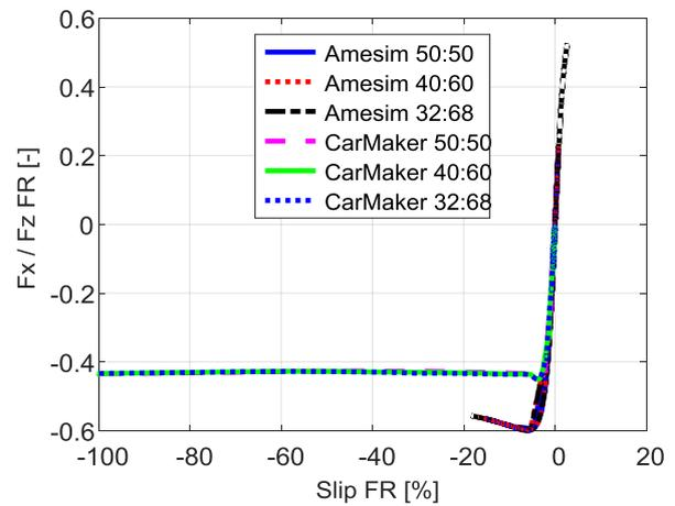
Figure 3.4.71 – Fx/Fz vs slip, front.
