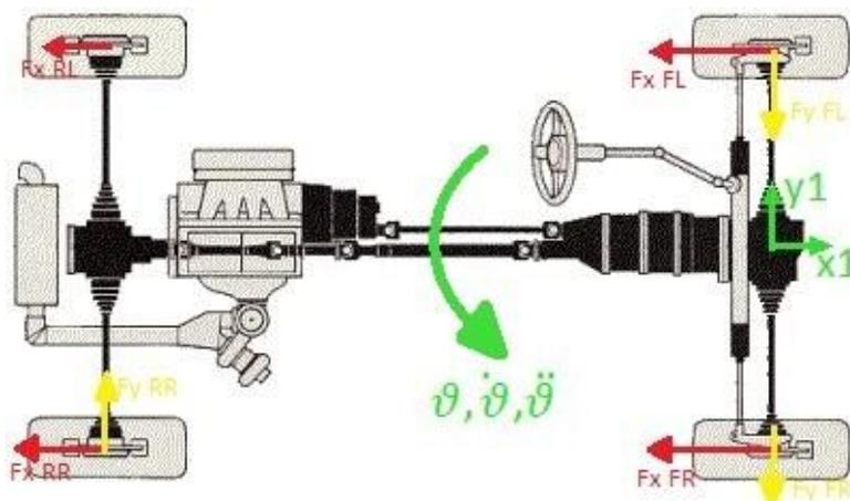
Figure 1.61 –Forces on the vehicle.
