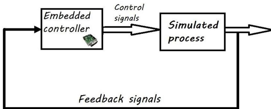
Figure I – Hil test scheme.
