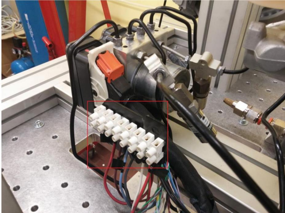
Figure 4.10 – Power terminal block
