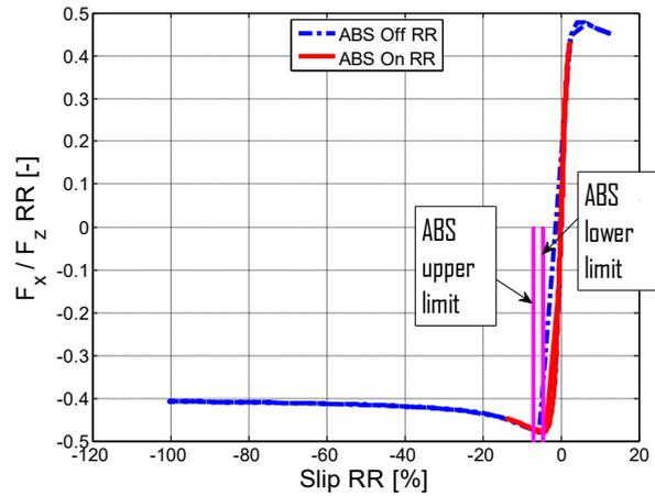
Figure 2.29 –  $F_x / F_z$  vs slip, rear.
