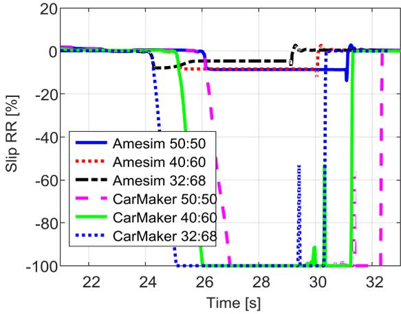
Figure 3.4.57 – Longitudinal slips, rear.
