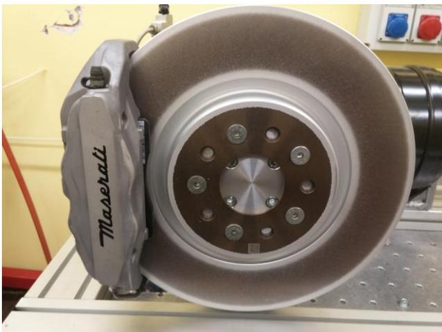
Figure 4.8 – Front brake disk and caliper.
