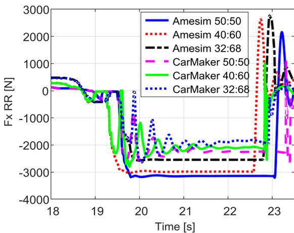
Figure 3.4.17 – Longitudinal forces, rear.
