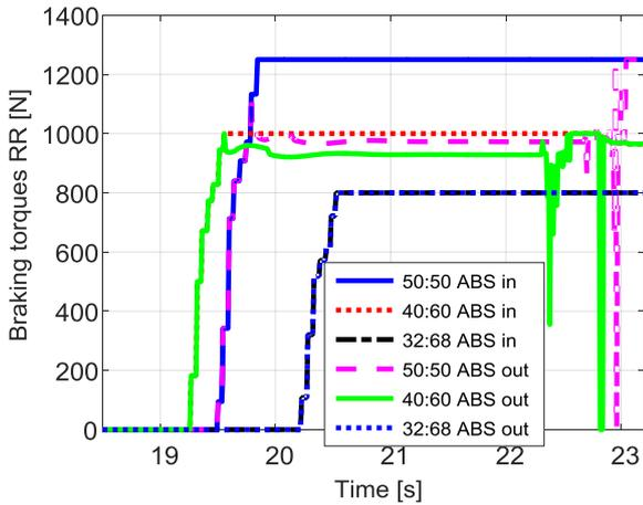
Figure 3.4.15 – Braking torques, rear.
