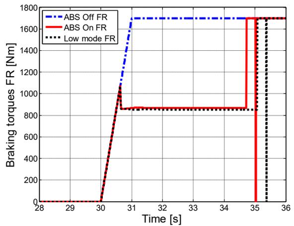
Figure 2.83 – Braking torques, front right.
