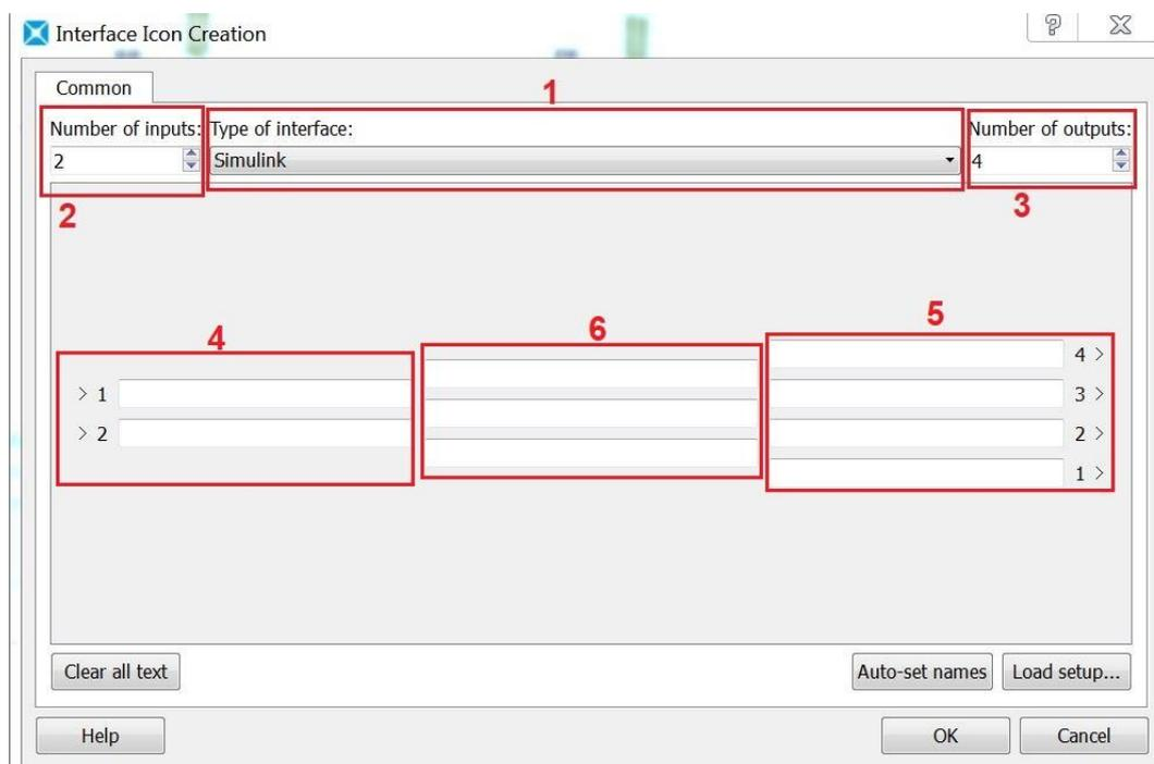
Figure 3.21 – Creation Amesim/Simulink interface.
