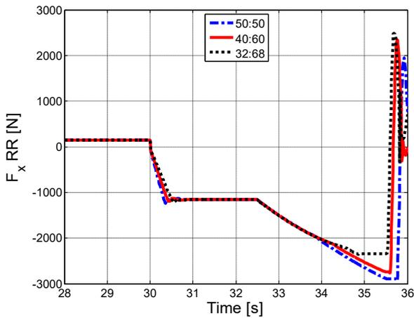
Figure 2.115 – Longitudinal forces, rear.
