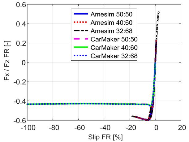
Figure 3.4.61 – Fx/Fz vs slip, front.
