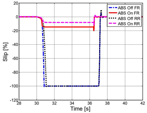
Figure 2.36 – Longitudinal slips.
