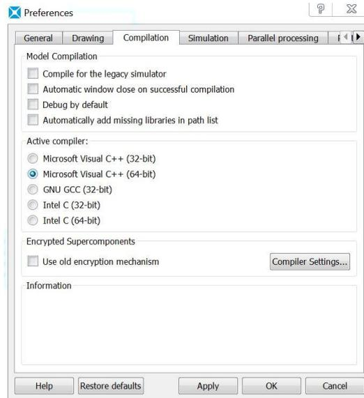
Figure 3.16 – Amesim, correctly selected compiler.
