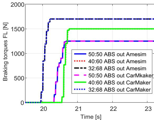
Figure 3.4.30 – Braking torques, front.
