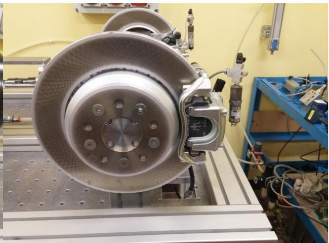
Figure 4.9 – Rear brake disk and caliper.
