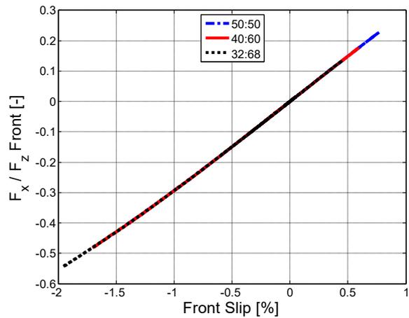
Figure 1.26 – Longitudinal force vs slip, front
