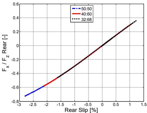
Figure 1.48 – Longitudinal force vs slip, rear.
