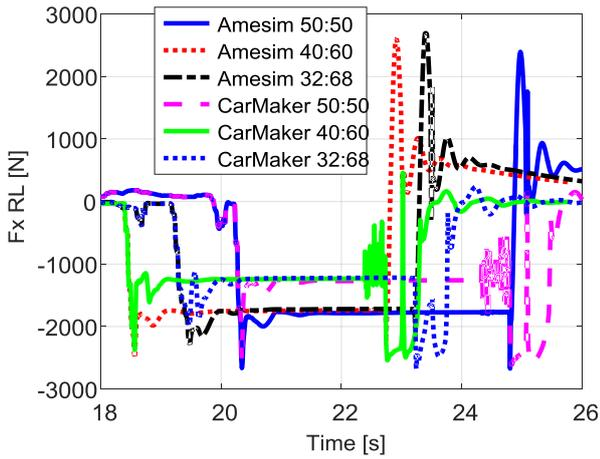
Figure 3.4.86 – Longitudinal forces, RL.
