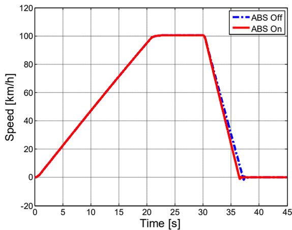
Figure 2.22 – Longitudinal speed.
