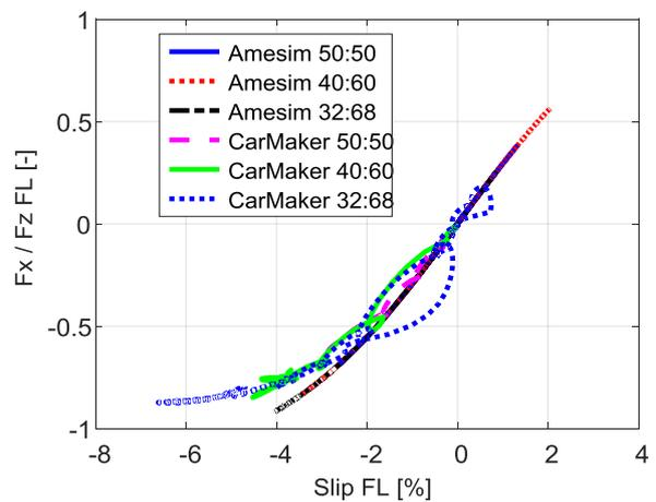
Figure 3.4.38 – Fx/Fz vs slip, front.
