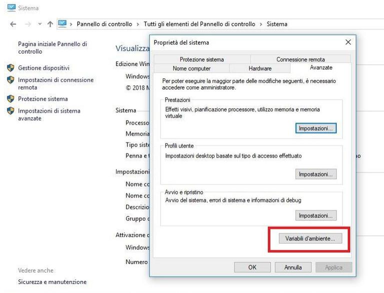
Figure 3.18 – How to set environment variable (the screen is in italian).
