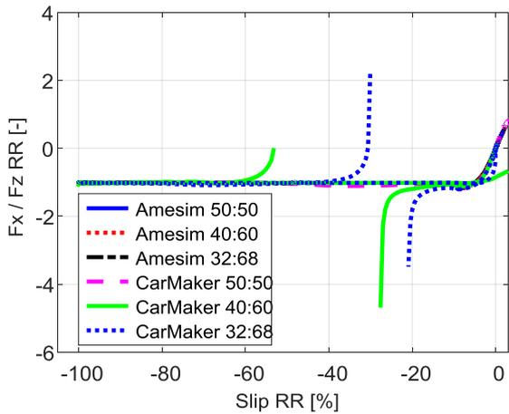
Figure 3.4.23 –  $F_x/F_z$  vs slip, rear.
