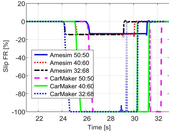
Figure 3.4.58 – Longitudinal slips, front.
