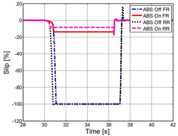
Figure 2.18 – Longitudinal slips.
