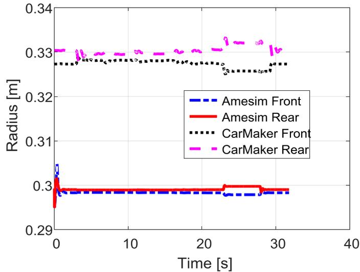
Figure III – Radius of the wheel.
