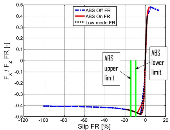
Figure 2.91 –  $F_x / F_z$  vs slip, front right.
