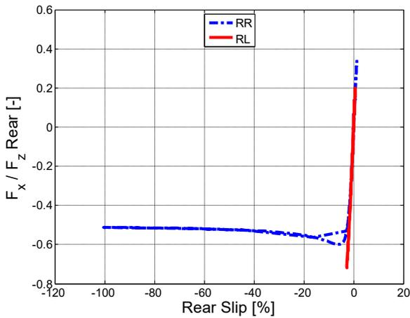
Figure 1.66 – Longitudinal forces vs slip, rear.
