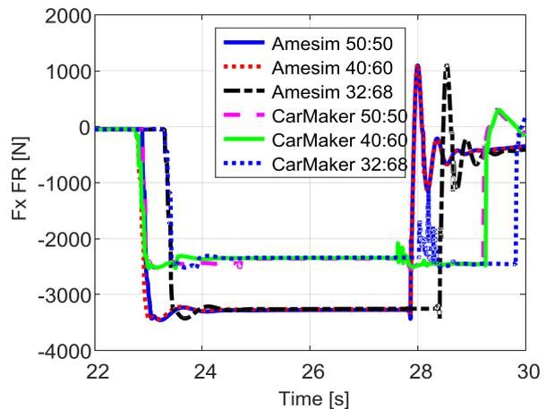
Figure 3.4.67 – Longitudinal forces, front.
