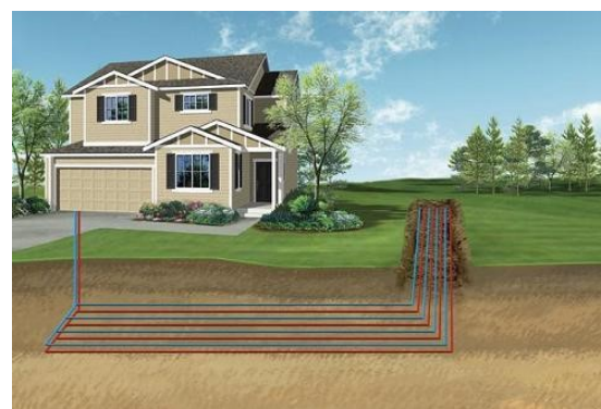
Figure 2.8 Closed loop system: horizontal ( www.firstgeothermalenergy.com )
