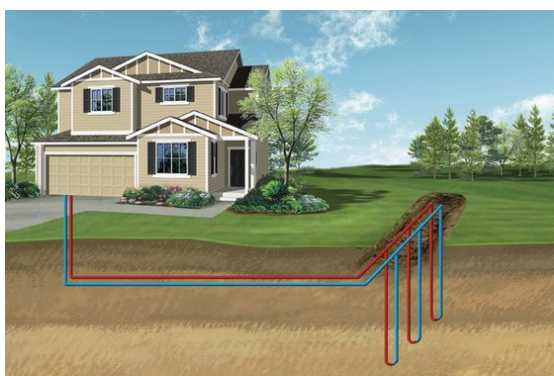
Figure 2.7 Closed loop system: vertical ( www.firstgeothermalenergy.com )
