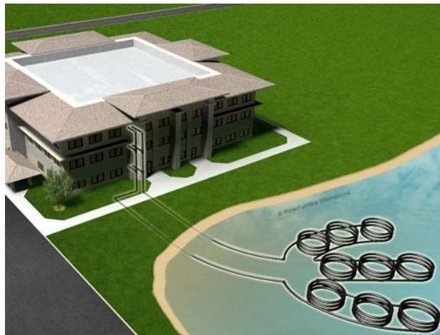
Figure 2.10 Pond loop system ( www.waterfurnace.com )
