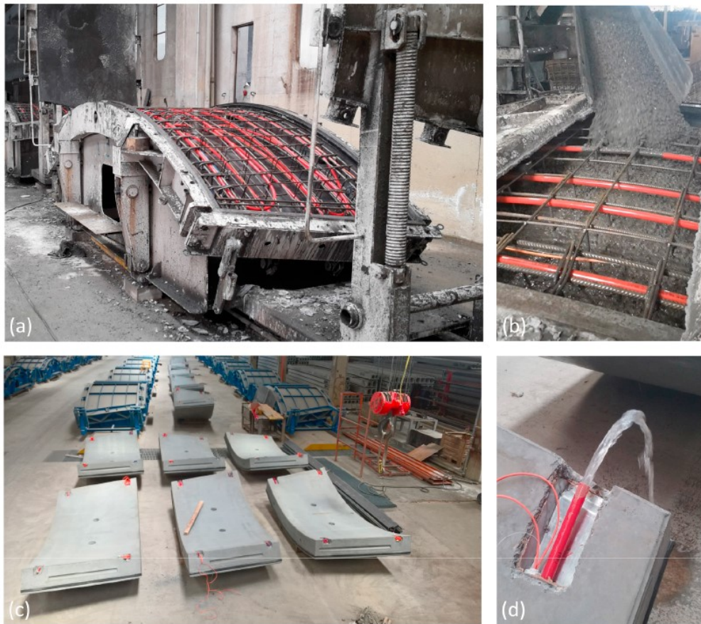
Figure 3.6 Preparation stages of energy segments: (a) moulding, (b) casting, (c) demoulding and (d) circulation test. (Barla et al., 2019)
