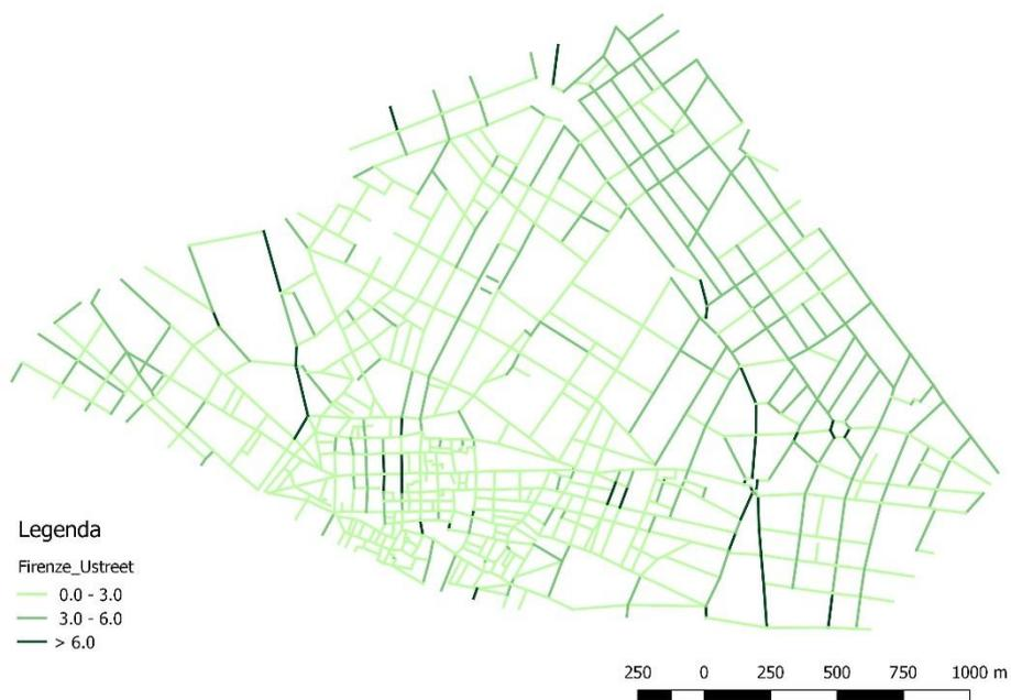
Figura 3.3.2.10 -  $U_{st}$ , per  $U = 10 \text{ m/s}$ ,  $\varphi = 180^\circ$
