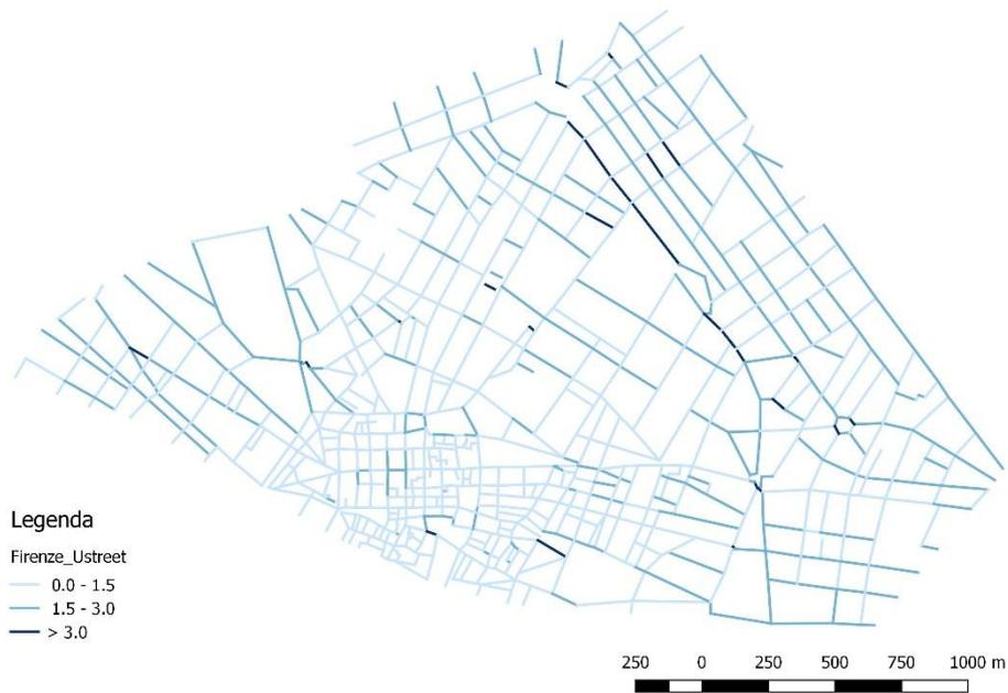
Figura 3.3.2.5 -  $U_{st}$ , per  $U = 5 \text{ m/s}$ ,  $\varphi = 135^\circ$
