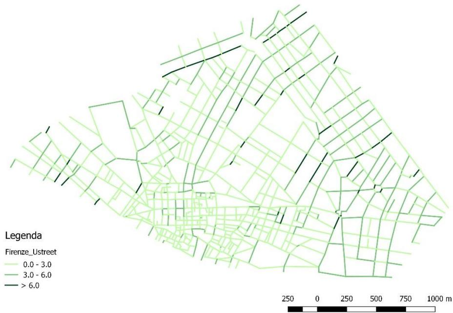
Figura 3.3.2.7 -  $U_{st}$ , per  $U = 10$  m/s,  $\varphi = 45^\circ$
