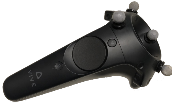
(a) Vive controller with retro-reflective markers
