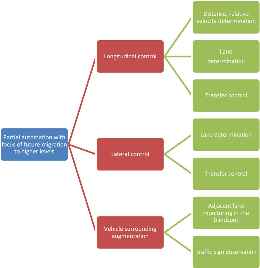
Figure 25 Objectives to preliminary function derived from concept exploration of ADAS functions
