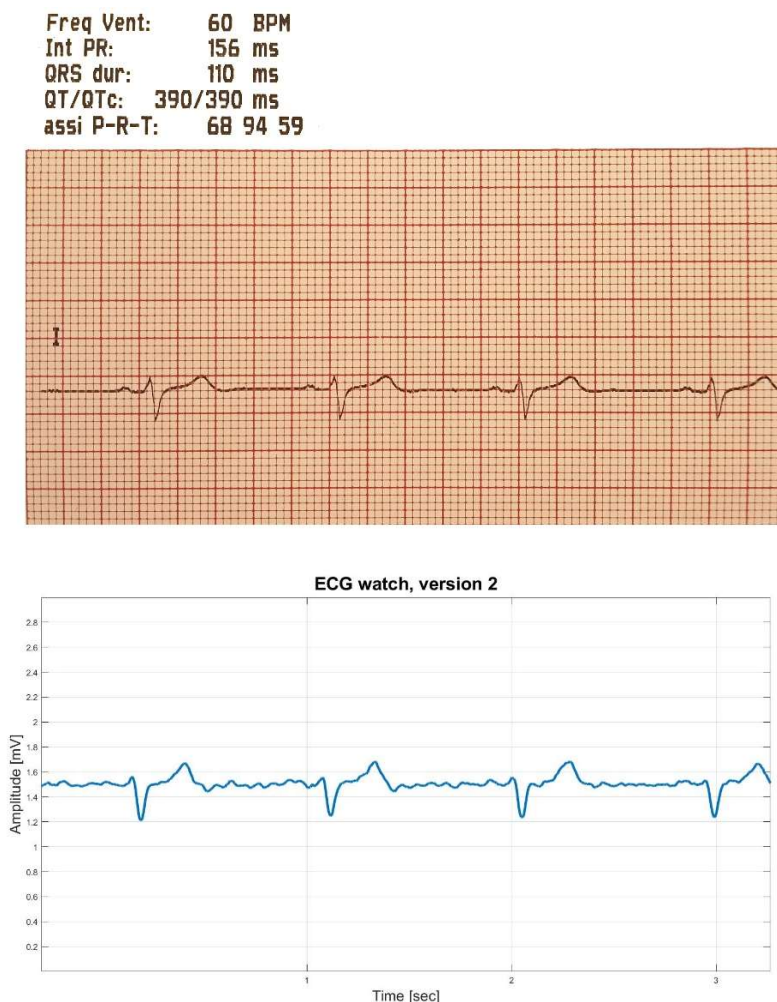
Figure 7.6: Comparison between a diagnostic ECG and the version 2 of the ECG watch; male patient, 27 years old.
