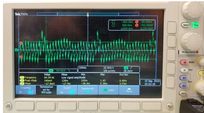
Figure 2.9: Oscilloscope displaying an ECG signal affected by the 50 Hz disturbance.
