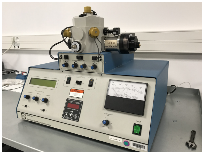
Figure 2.9: Gatan PECS sample coating and etching system Source: Texplained
