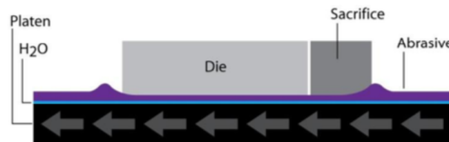
(b) A sacrificial silicon layer can be used to protect the sample from unwanted edge effects
