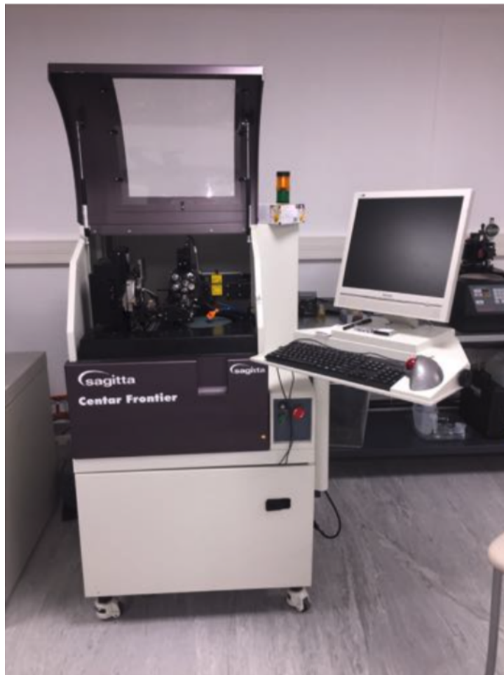
Figure 2.5: Sagitta station, integrating a CMP machine and an optical microscope Source: Texplained
