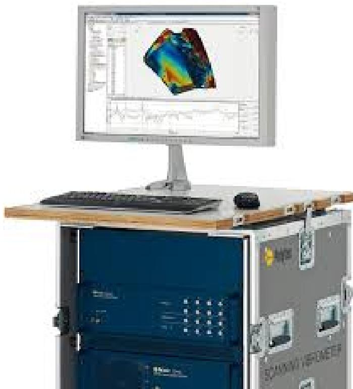
Figure 4.1: A figure showing the electronic unit of the polytec laser scanning vibrometer
