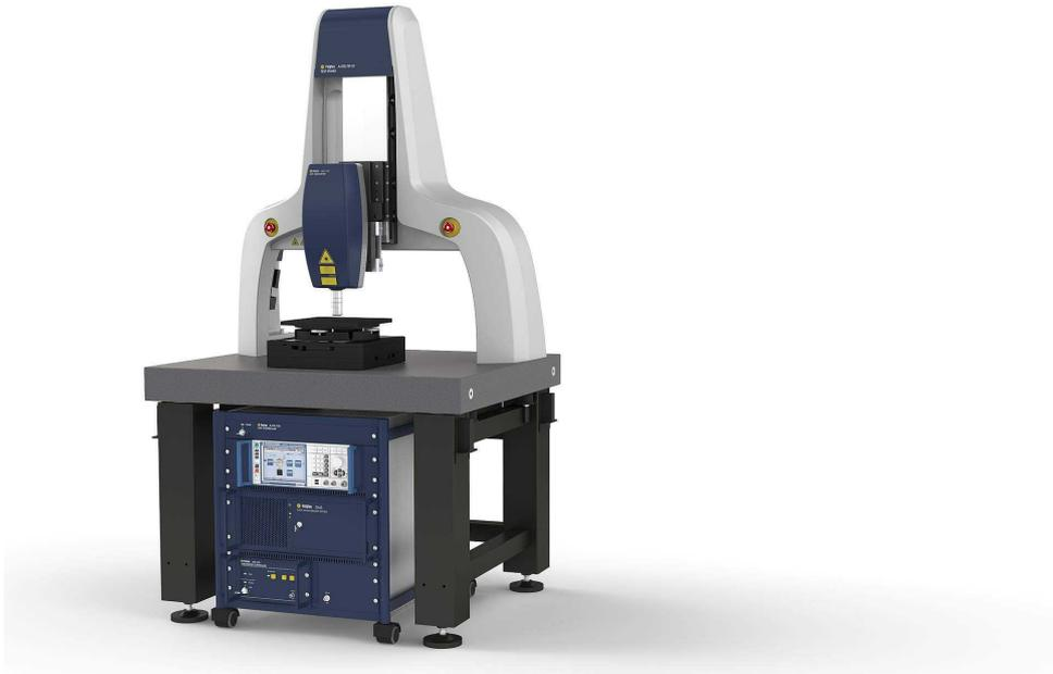
Figure 4.2: A figure showing the scanning vibrometer of the polytec laser scanning vibrometer
