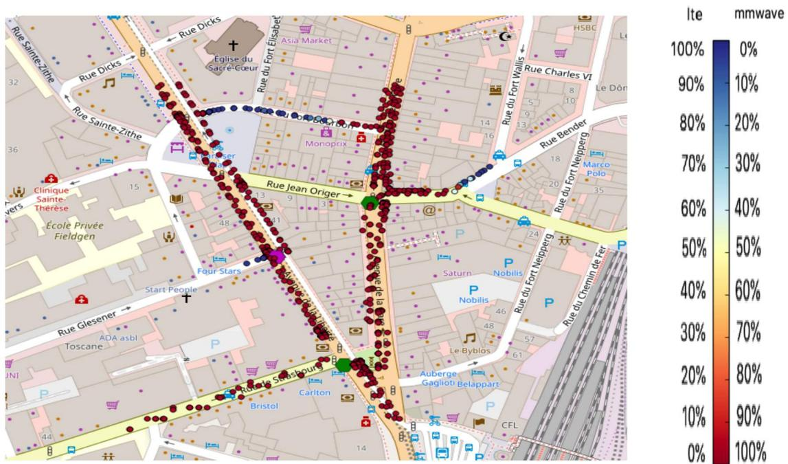
**Figure 5.7** Colourmap with percentage of short-term throughput LTE and mmwave per user using two gNB with RLC UM and ULA 4x4
