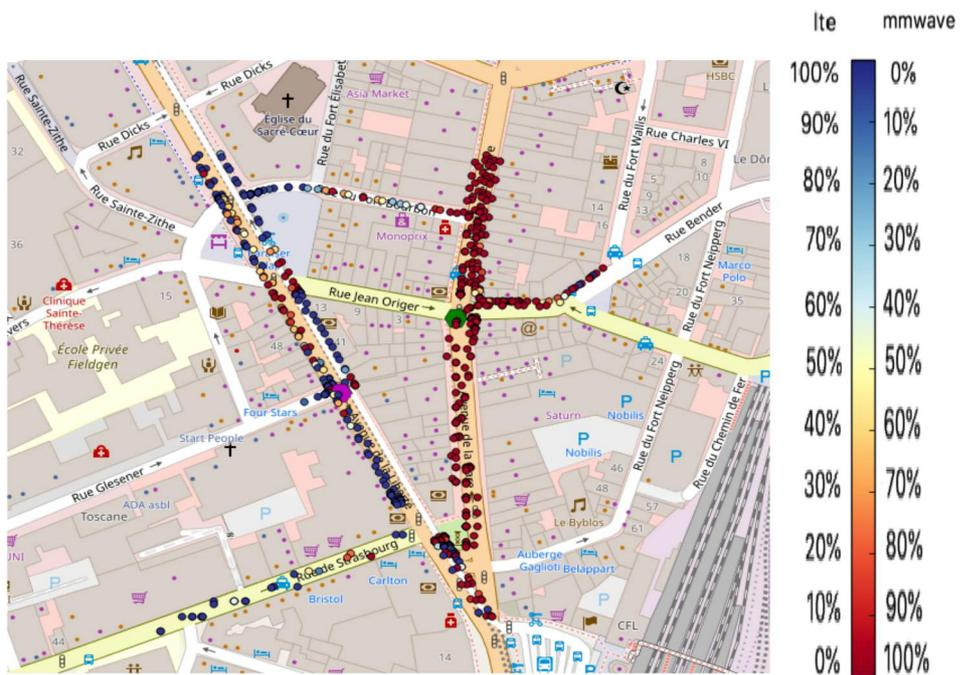
**Figure 5.21** Colourmap with percentage of short-term throughput LTE and mmwave per user using one gNB with RLC UM and ULA 64x64
