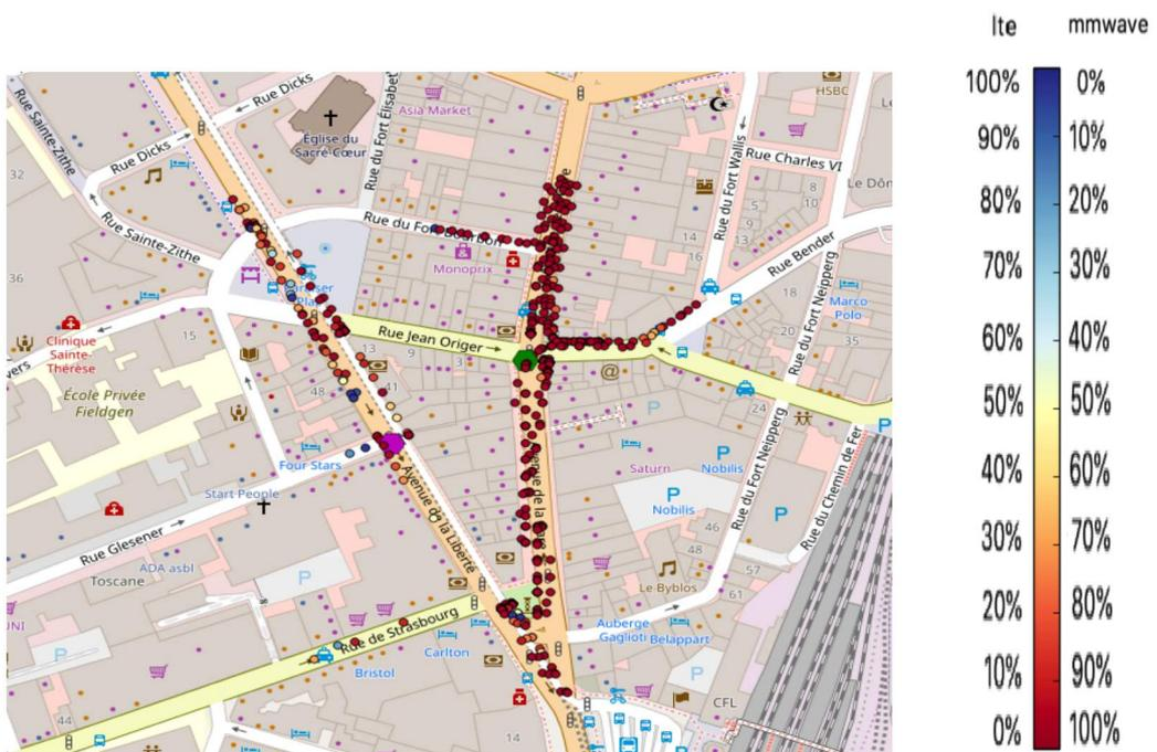
**Figure 5.29** Colourmap with percentage of short-term throughput LTE and mmwave per user using one gNB with RLC AM and ULA 64x64
