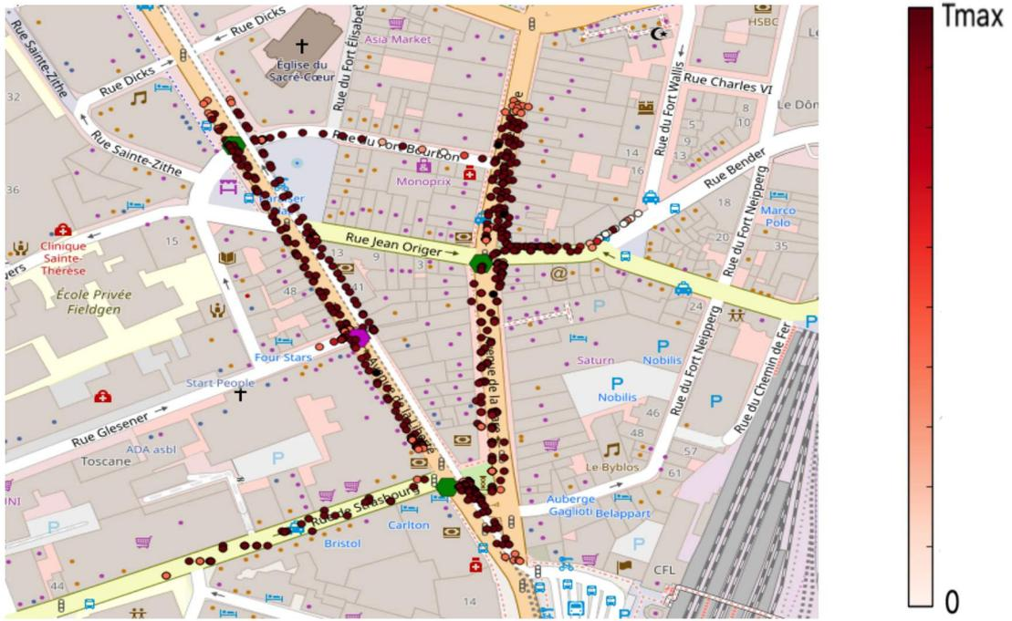
**Figure 5.8** Colourmap with short-term throughput indication per user using three gNB with RLC UM and ULA 4x4
