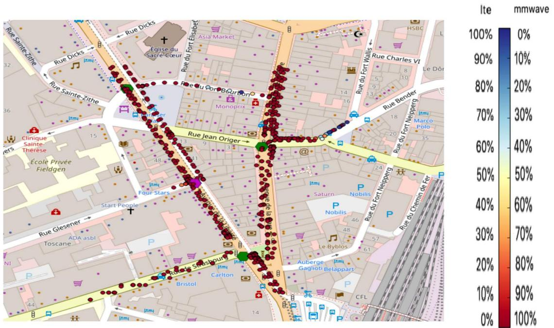
**Figure 5.9** Colourmap with percentage of short-term throughput LTE and mmwave per user using three gNB with RLC UM and ULA 4x4
