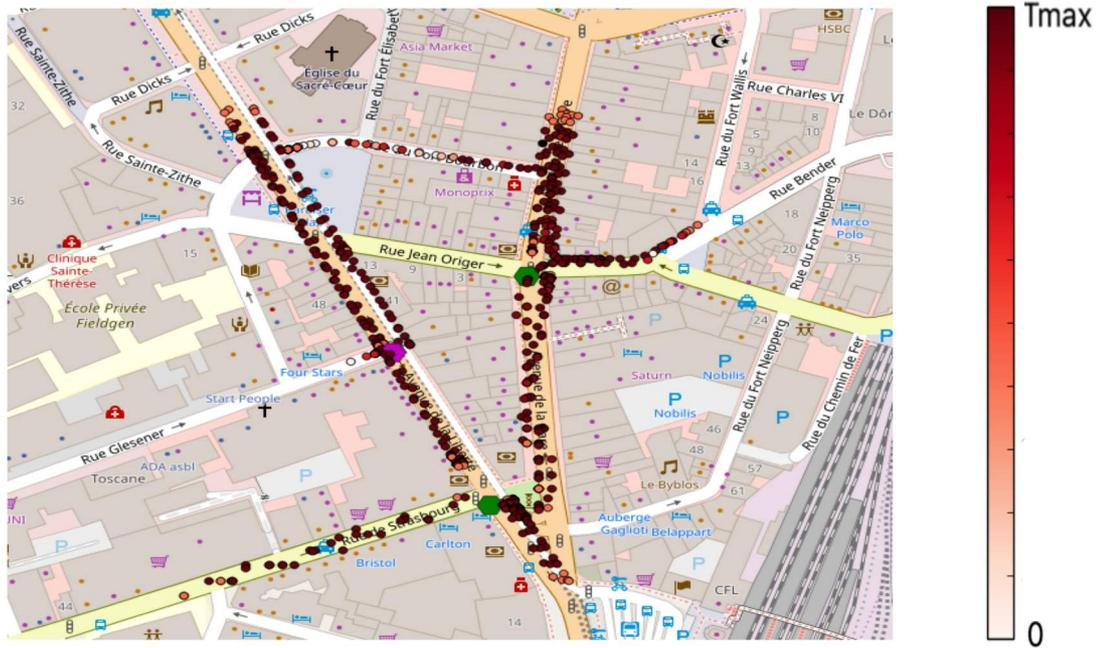
Figure 5.16 Colourmap with short-term throughput indication per user using two gNB's with RLC UM and ULA 16x16
