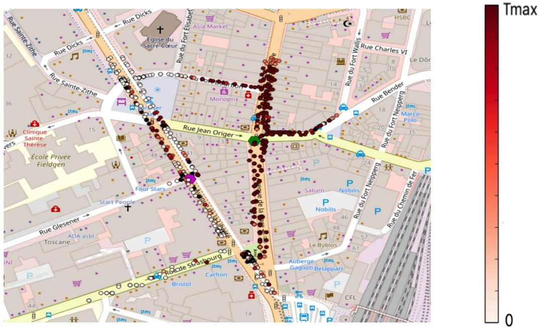
**Figure 5.14** Colourmap with short-term throughput indication per user using one gNB with RLC UM and ULA 16x16
