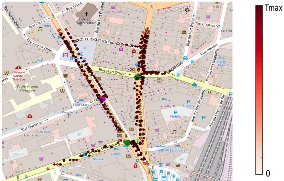
**Figure 5.6** Colourmap with short-term throughput indication per user using two gNB with RLC UM and ULA 4x4
