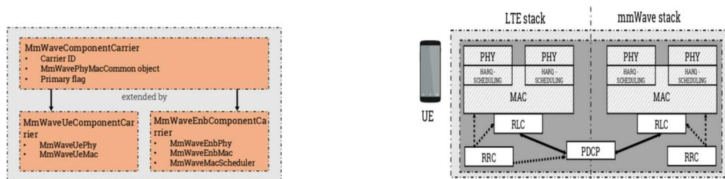
**Figure 3.9 (a)** Information represented by instances of `MmWaveComponentCarrier` and extensions
