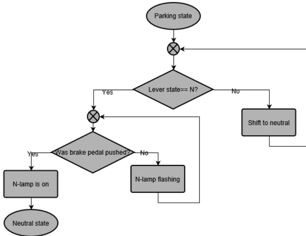
Figure 8 Parking to Neutral Transition Flowchart
