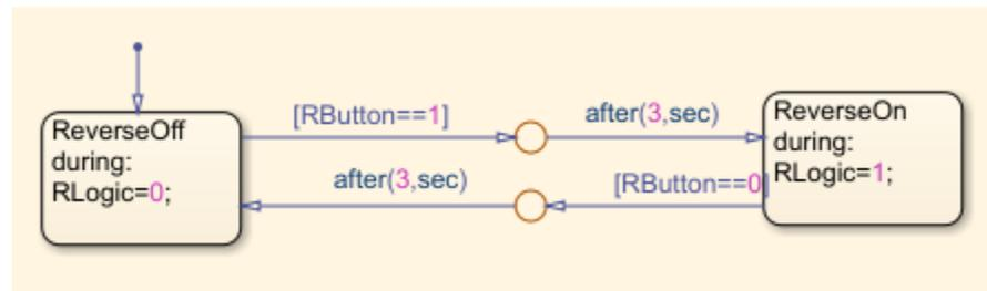
Figure 21 Reverse Logic Modelling in Stateflow
