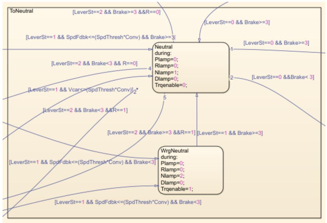
Figure 25 Moving to Neutral from Drive Logic Modelling in Stateflow
