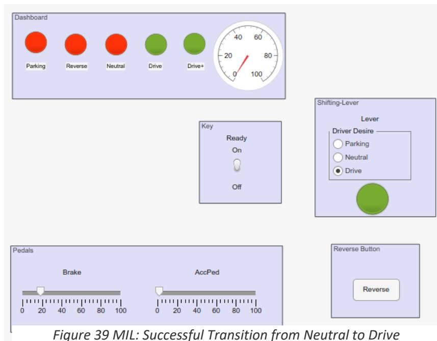
Figure 39 MIL: Successful Transition from Neutral to Drive
