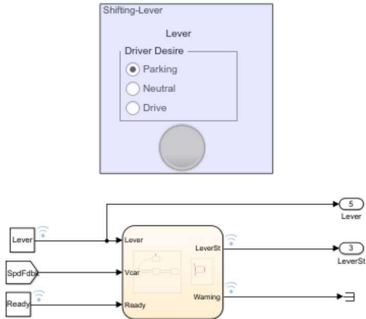
*Figure 15 Gear-Shift Lever Modelling in Simulink*
