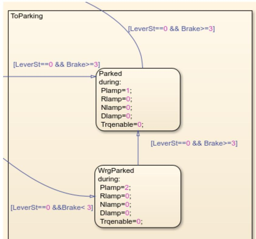
Figure 26 Moving from Neutral to Parking Logic Modelling in Stateflow
