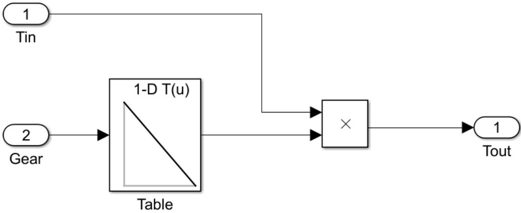
Figure 31 Transmission Ratio Selection
