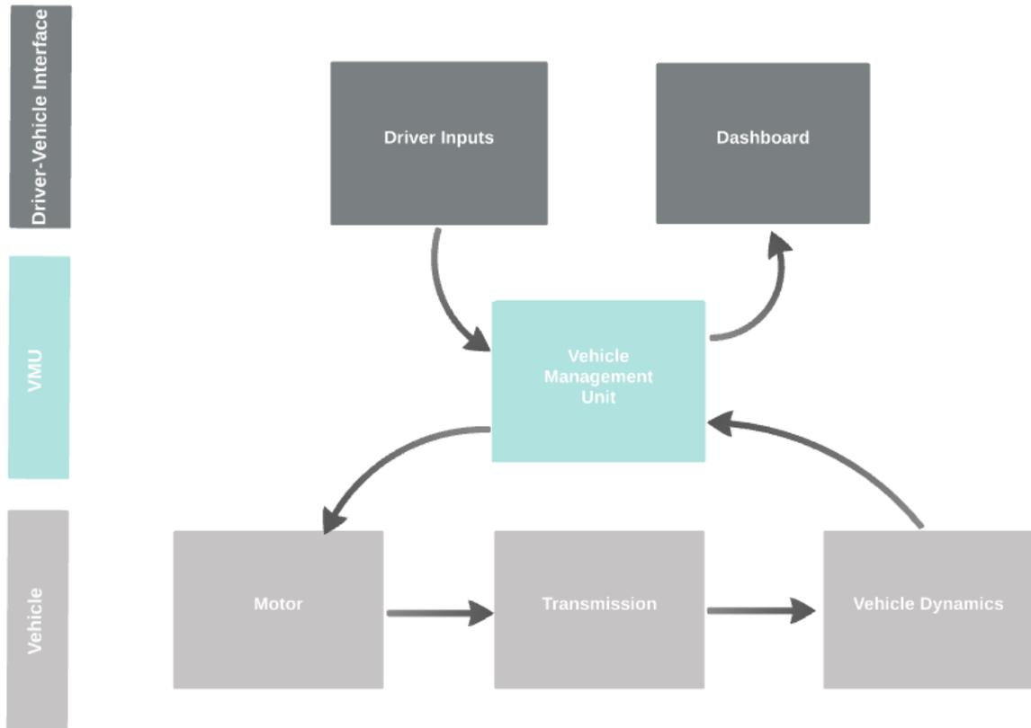
*Figure 6 System Overall Scheme*
