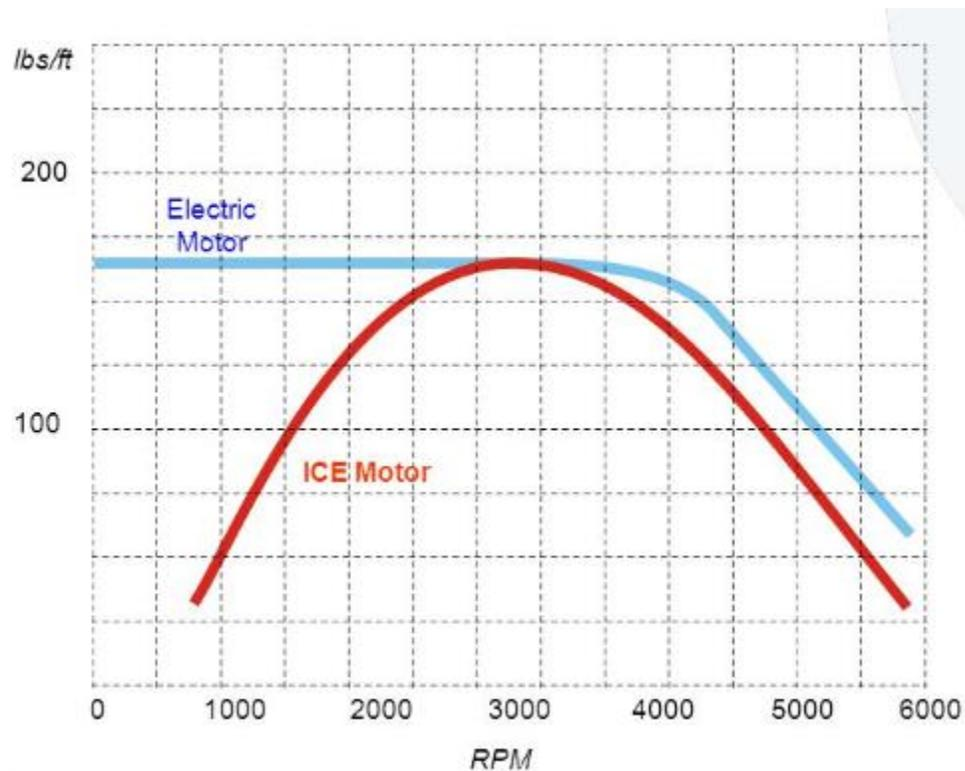
Figure 2 Electric Motor Vs. ICE Torque-Speed Diagram
