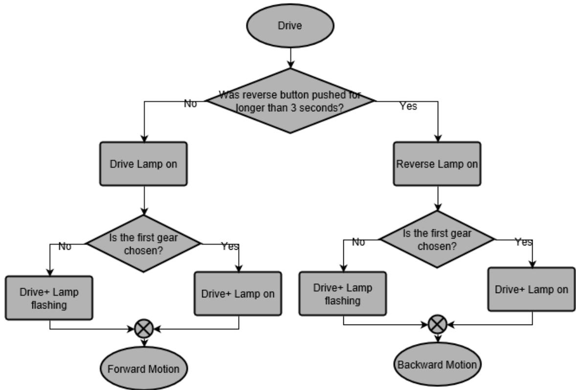
Figure 10 Moving Forward and Backward Flowchart
