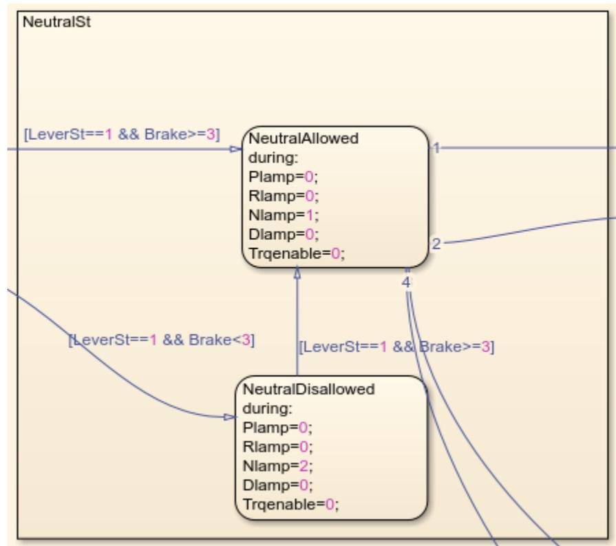
Figure 23 Moving to Neutral Logic Modelling in Stateflow
