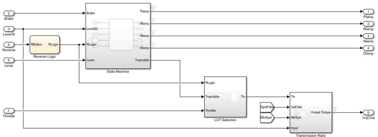
*Figure 20 Vehicle Management Unit in Simulink*
