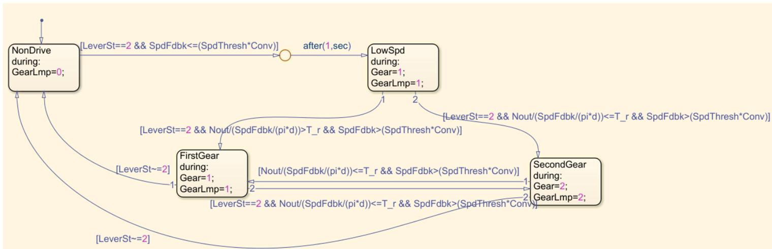
Figure 30 Gear Detection Logic Modelling in Stateflow
