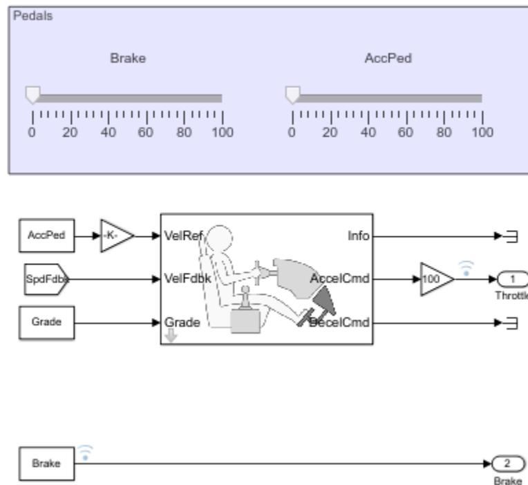
Figure 14 Pedals Modelling in Simulink
