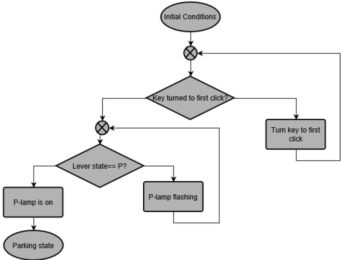
Figure 7 Initial Conditions Flowchart
