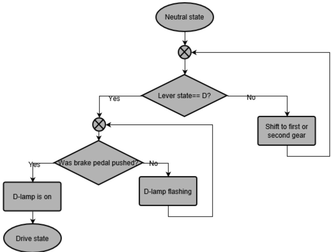
Figure 9 Activating Drive State Flowchart
