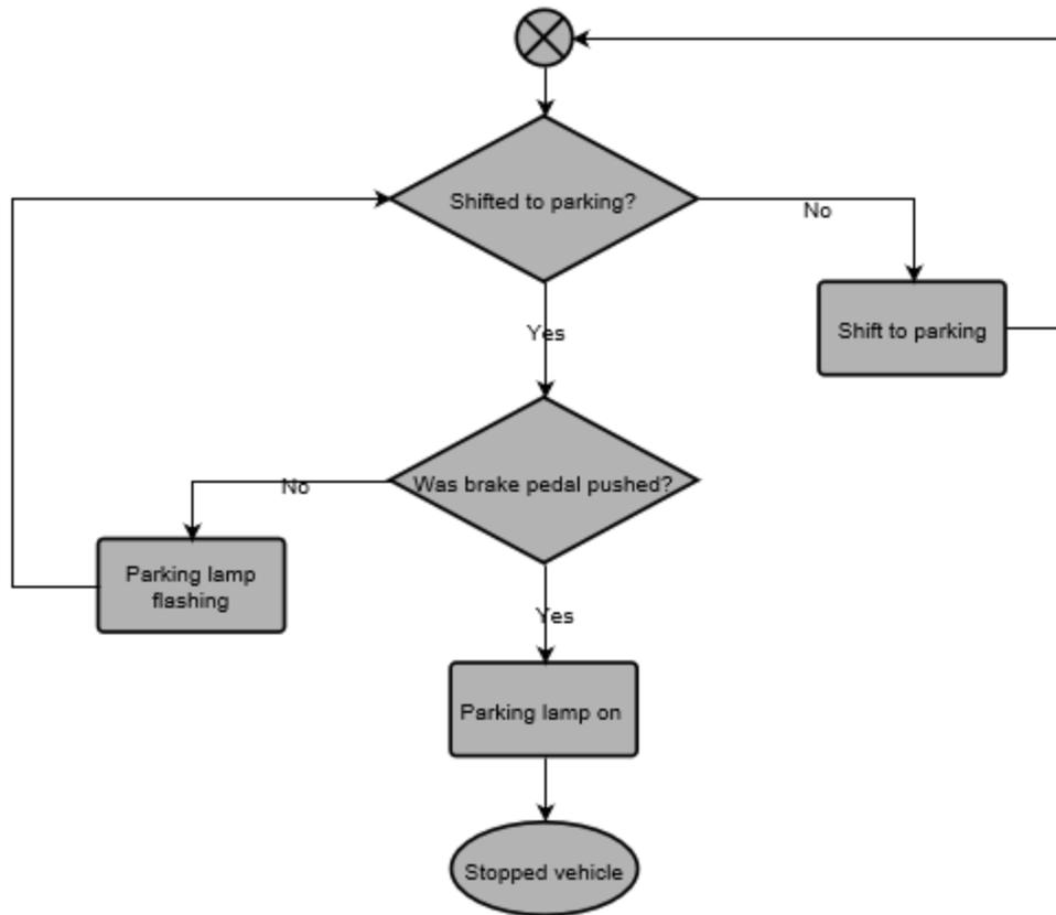
Figure 11 Going to Neutral and Parking from Drive Flowchart
