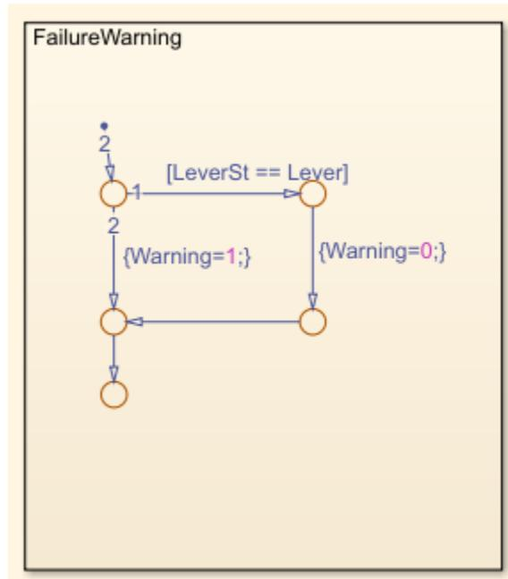
Figure 17 Lever Warning Logic in Stateflow
