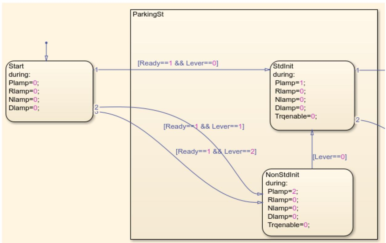
Figure 22 Initial Standard Conditions Logic Modelling in Stateflow
