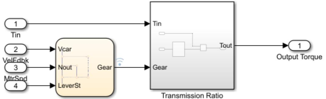
Figure 29 Gear Detection Modelling in Simulink
