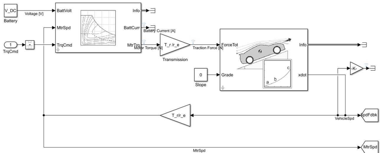
Figure 32 Vehicle Dynamics Modelling in Simulink
