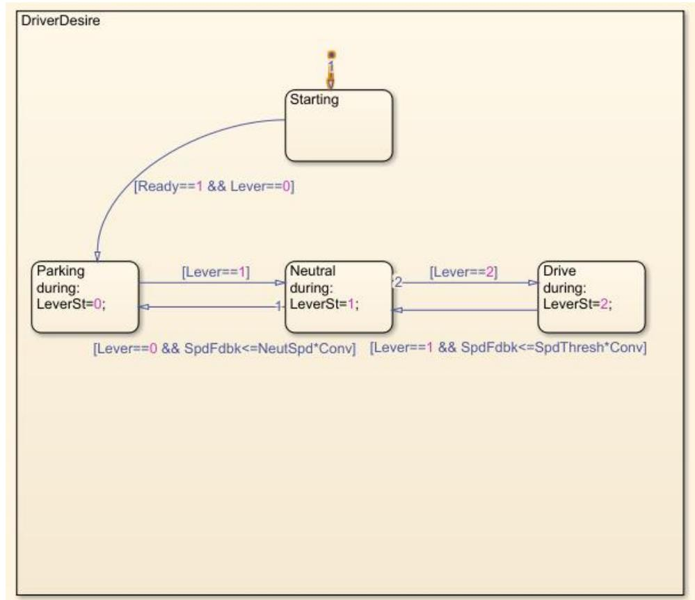
Figure 16 Lever State Machine in Stateflow
