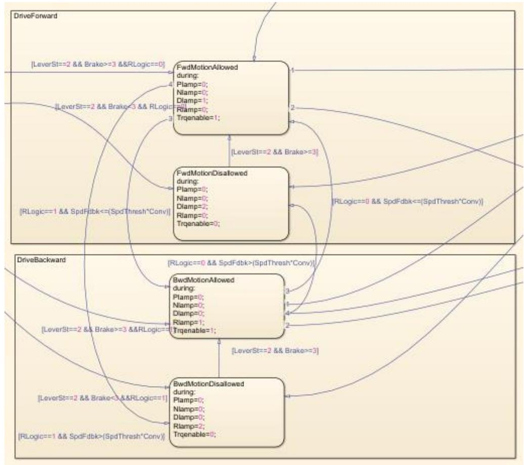
Figure 24 Moving Forward and Backward Logic Modelling in Stateflow
