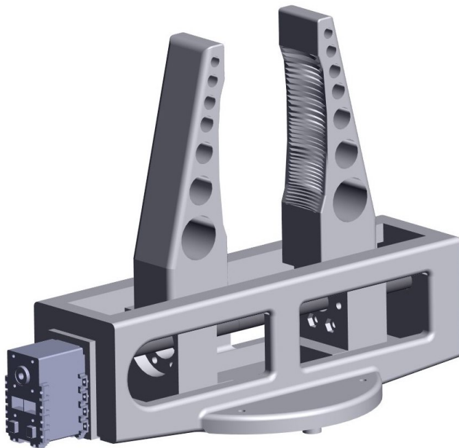
Figure 4.14: The gripper with screw mechanism
