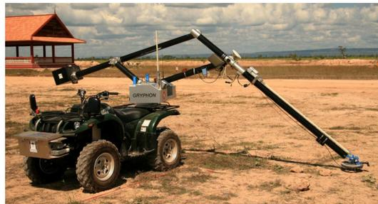
Figure 1.5: pantograph manipulator balanced by a counterweight, mounted on a demining rover.
