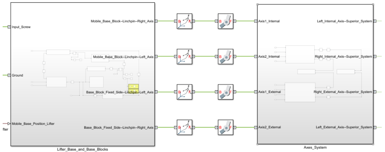
Figure 3.52: Assembly of axes system with base system model
