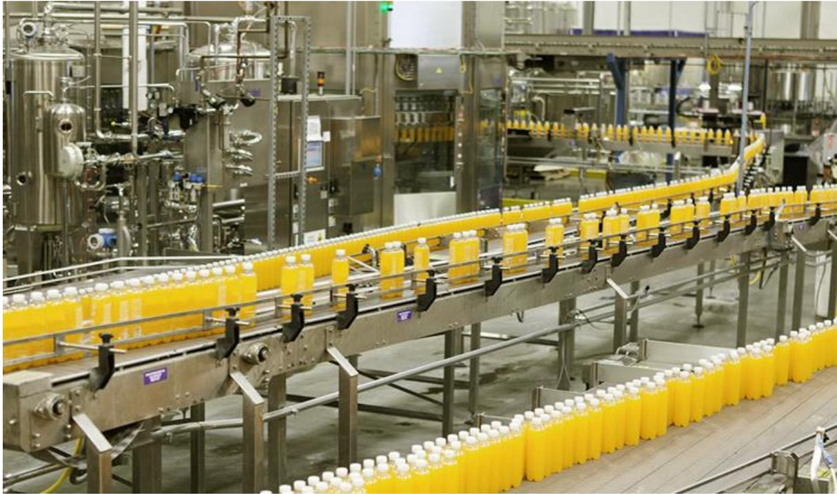
Figure 27: Conveyer system in beverage industry [43].
