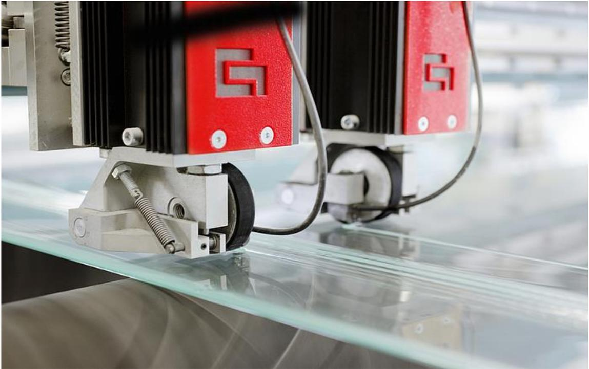
Figure 26: Float glass cutting tool [42].
