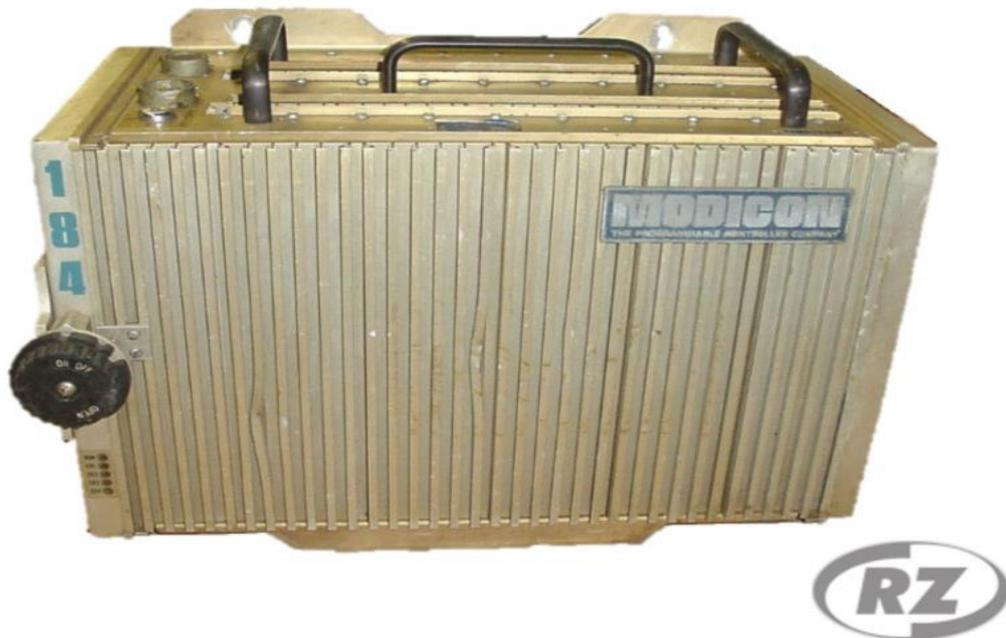
Figure 2: Modicon 184, second generation of PLC by Modicon [18].
