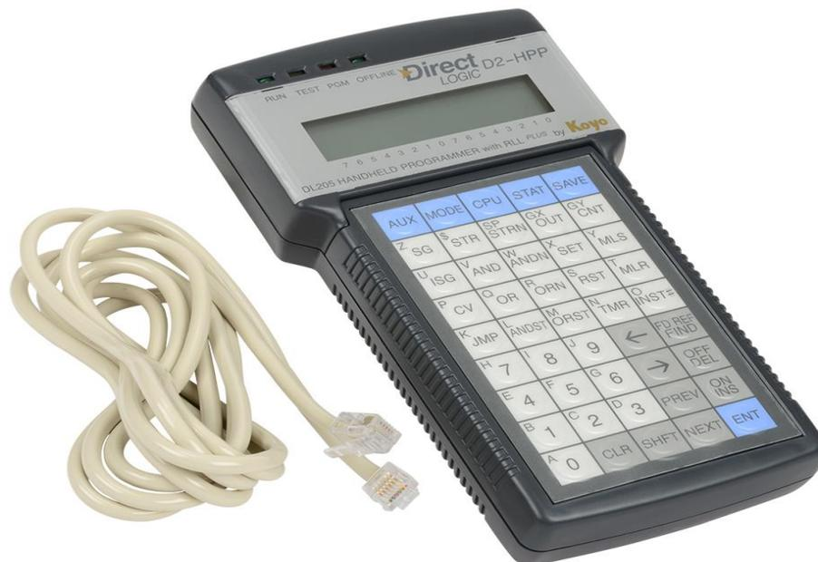
Figure 9: Hand-Held programming device [25].
