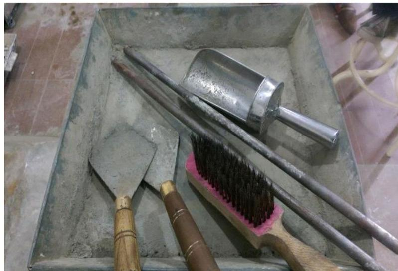
**Figure3. 11**Trowels, trays and tamping rods
