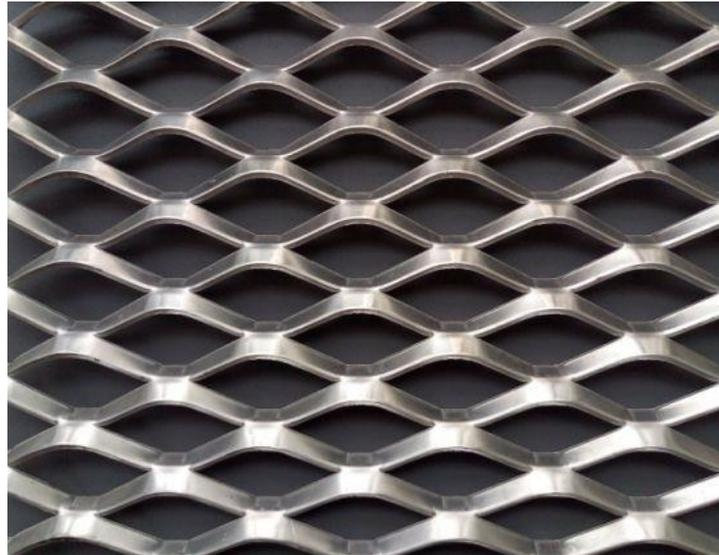
**Figure3. 2:** Expanded steel mesh close view
