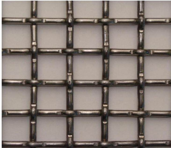
**Figure3. 4:** Woven steel mesh close view
