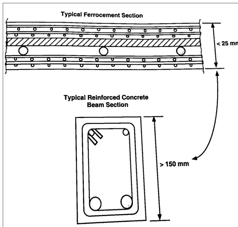
**Figure1. 4:** Typical cross section of Ferro-cement VS reinforced concrete
