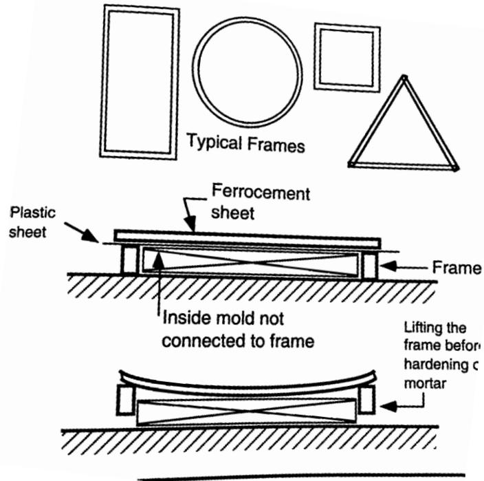
**Figure5. 4:** Shell shaped elements (NAMAAN 2000)
