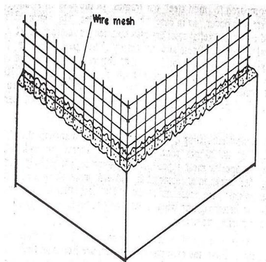
**Figure1. 1:** Typical section of Ferro-cement element
