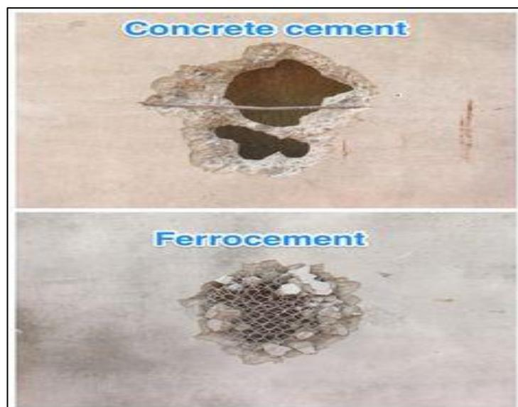
**Figure4. 7:** Explosive protection of RCC and Ferro-cement
