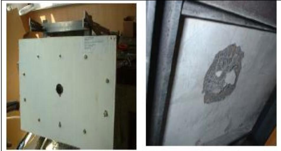
**Figure4. 4:** impact resistance of Ferro-cement sample
