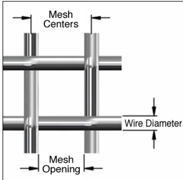
**Figure3. 1:** Mesh openings close view
