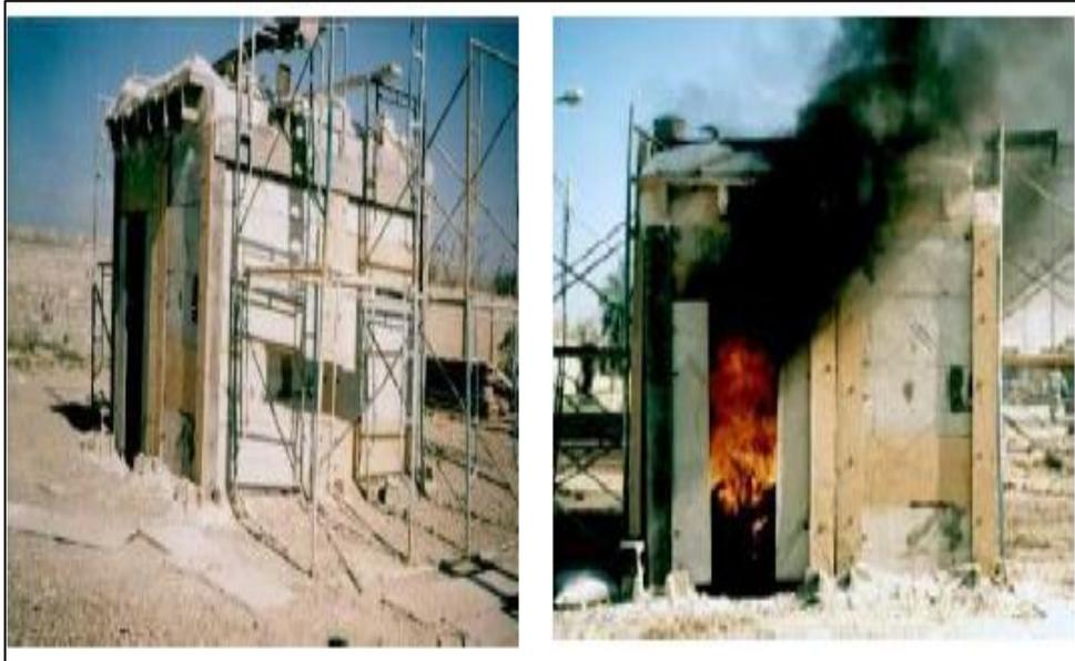
**Figure4. 6:** Fire resistance of Ferro-cement compartment
