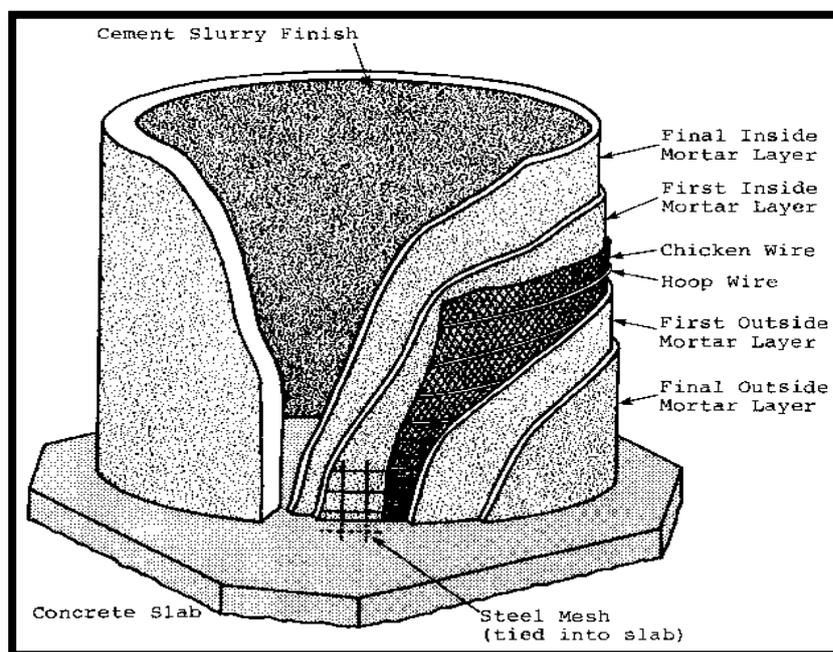
**Figure3. 14:** Detailed View of Ferro-cement Construction
