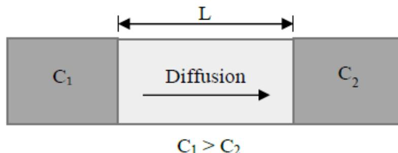
**Figure4. 1:** Schematic representation of the diffusion process (Bertolini, 2006)
