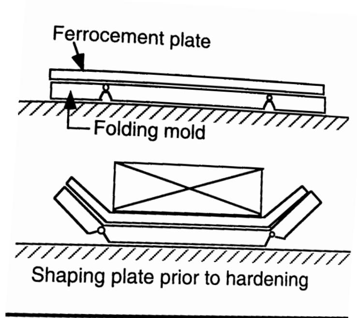
**Figure5. 3:** Moulding of flat plate to U shaped section (NAMAAN 2000)
