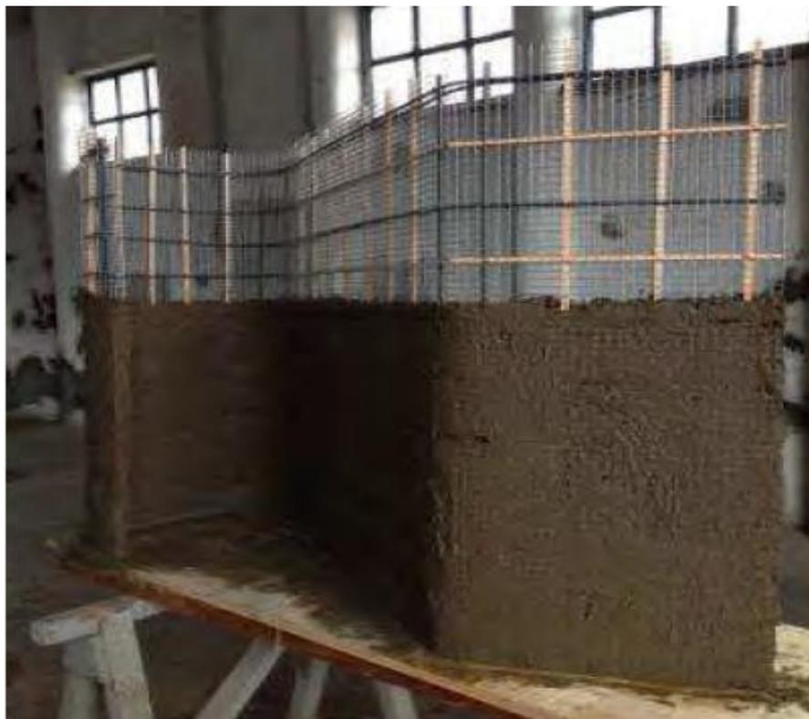
**Figure5. 12:** Ferro-cement Model Curly wall
