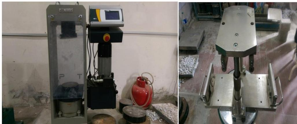
**Figure3. 9:** Compression Testing Machine with flexural arrangement
